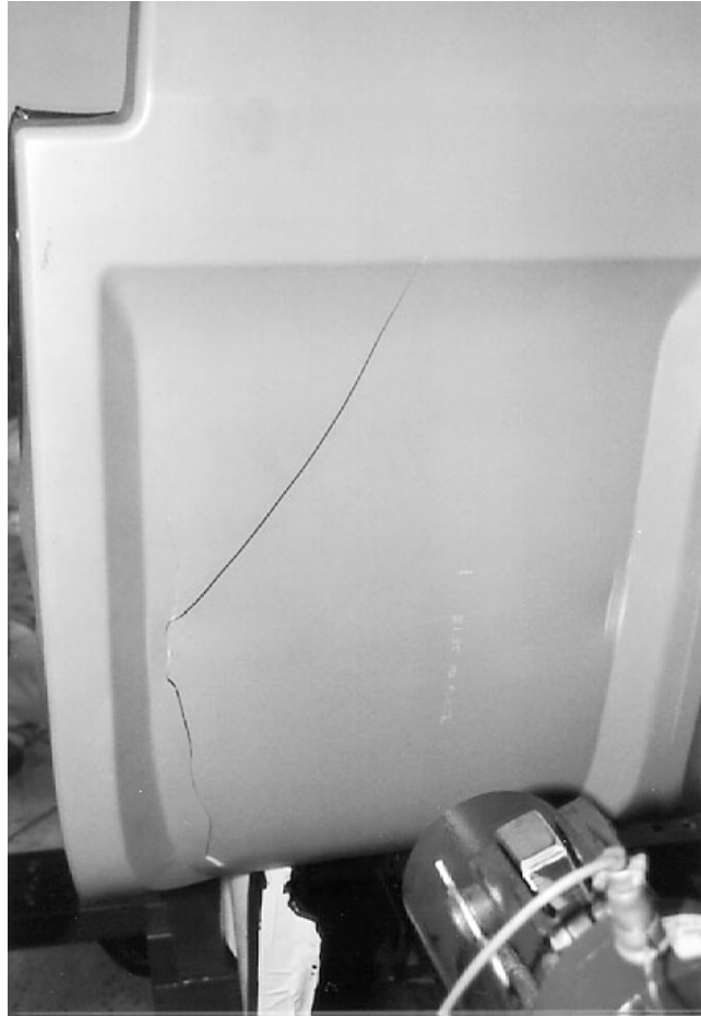
Figure 17. M-Style Lower (Post-test) - Plastic Shroud Cracked
