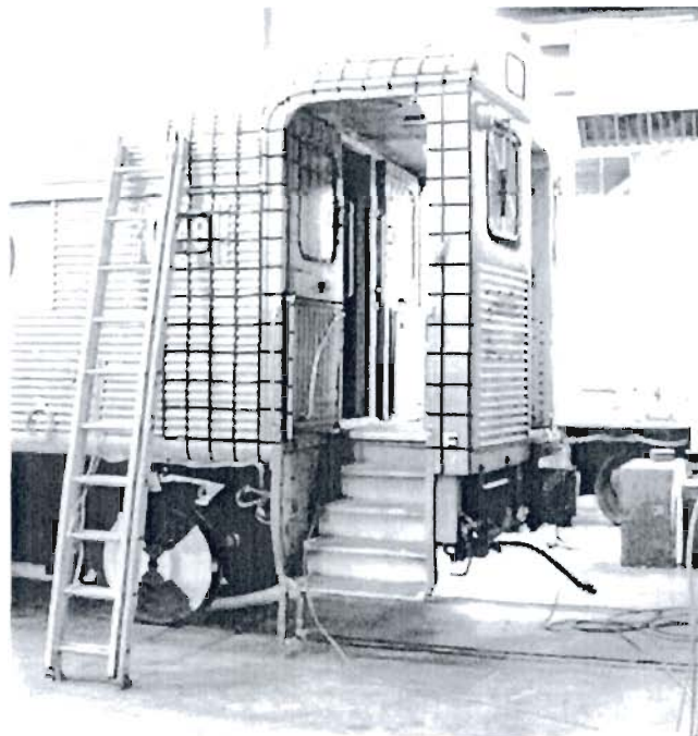
Figure 16. Photo of Impact End of Leading Car Prior to Two-Car Impact Test
