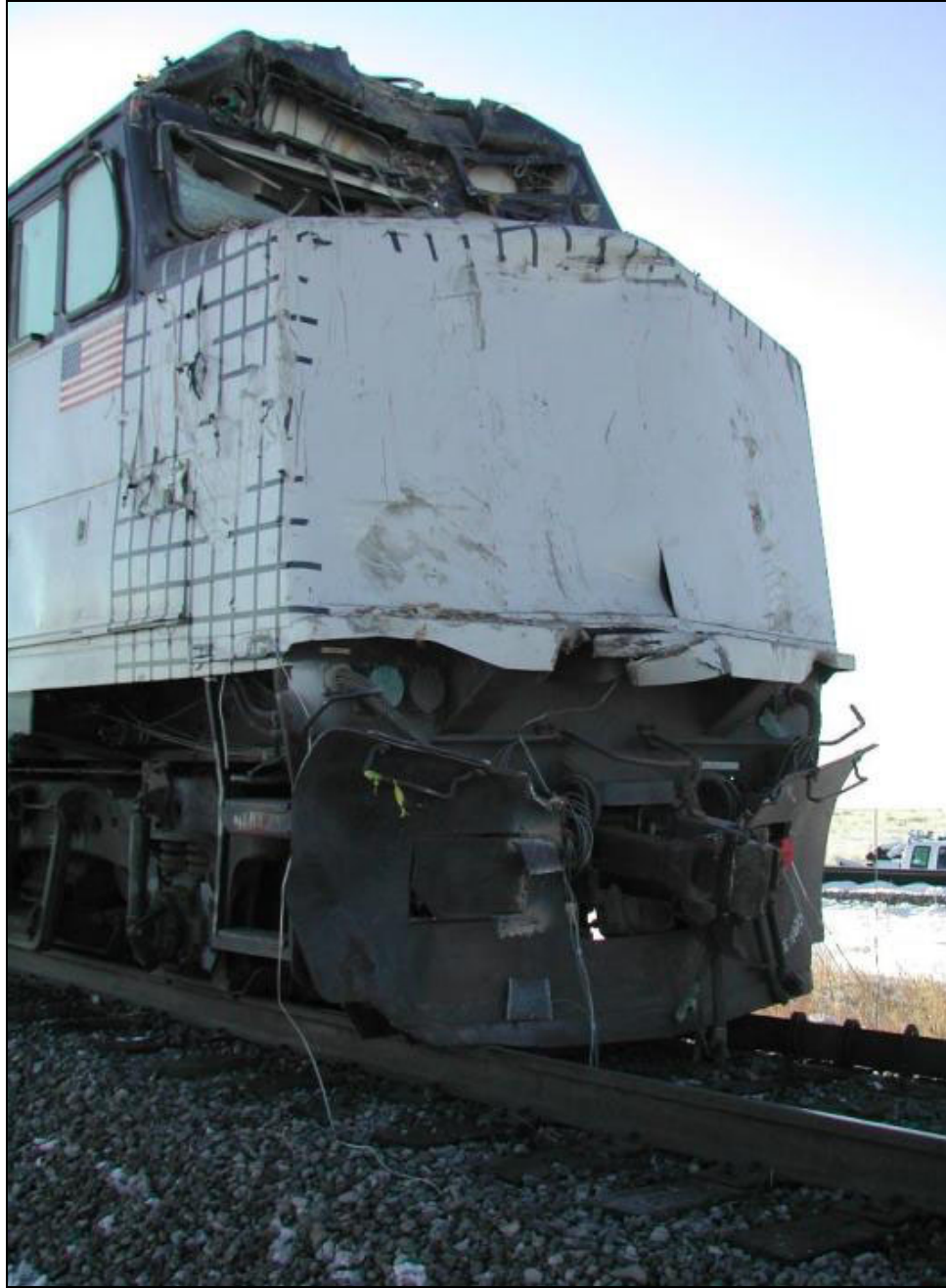
Figure 11. Locomotive after Impact
