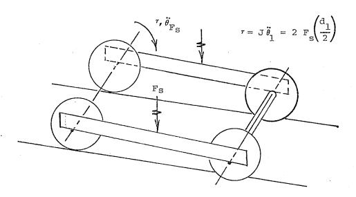
Case 2: Two spring forces ( $\frac{1}{2}$  weight of car body) acclerates the truck.
