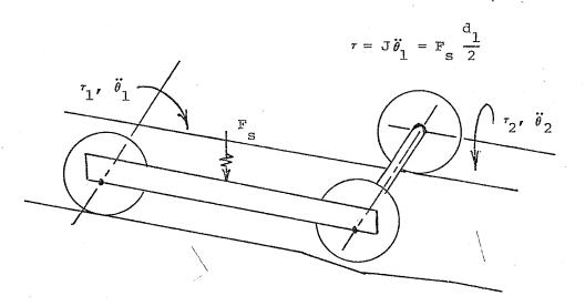
Case 1: Only a single spring force ( $\frac{1}{4}$  weight of car) accelerates the truck
