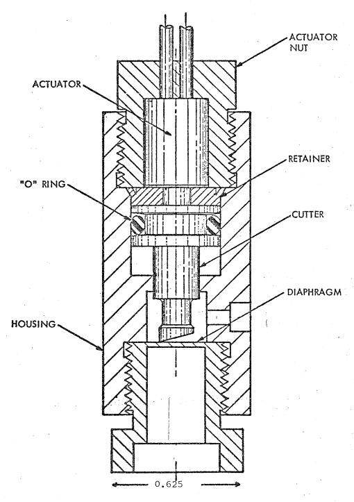
FIGURE P-1. EXPLOSIVE DIAPHRAGM CUTTER ASSEMBLY
