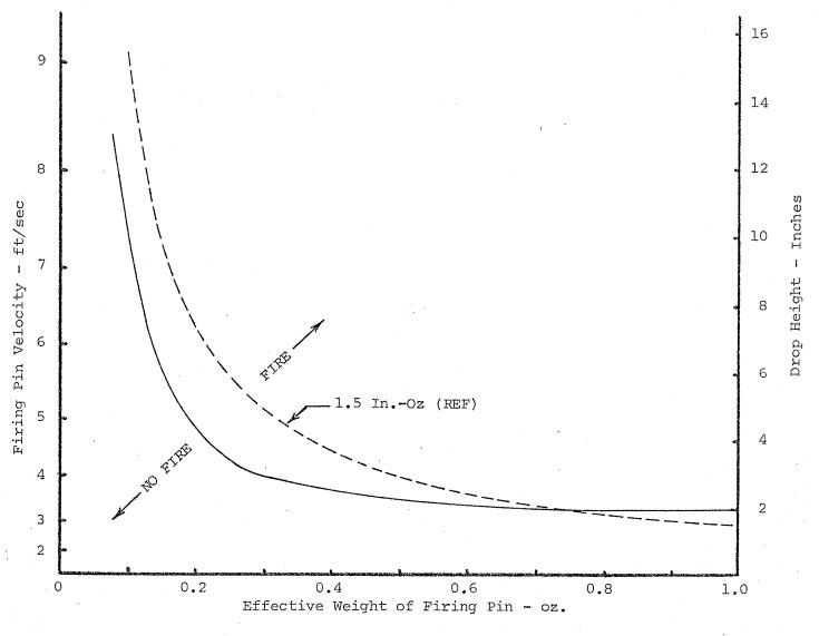
FIGURE 8. STAB PRIMER FIRING ENERGY - TYPICAL
