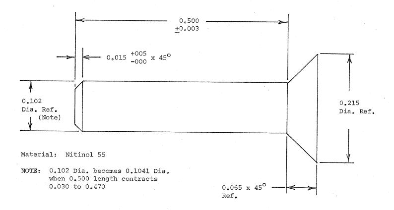
FIGURE 15. THERMAL RELEASE PIN
