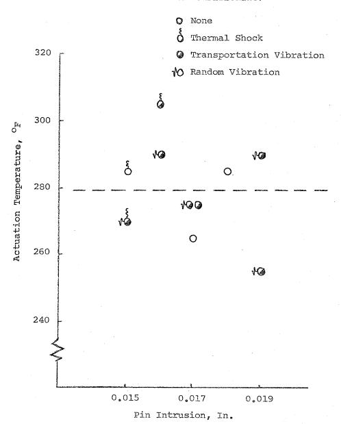
FIGURE 16. NITINOL THERMAL SENSOR TESTS, ACTUATION TEMPERATURE VERSUS PIN INTRUSION
