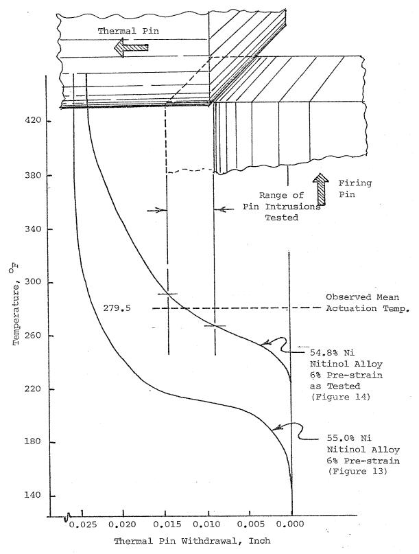
FIGURE 17. THERMAL SENSOR DESIGN ANALYSIS
