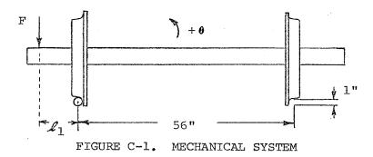
The force acting on the system is the total weight of the car and lading acting through the springs. This results in a torque being applied to the entire wheel-axle side frame system. This torque is resisted by the rotational inertia of the wheels, axles and the far side frame about an axis through the point of wheel-rail contact in the following manner:
