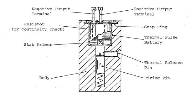
FIGURE 27. THERMAL SENSOR-THERMAL BATTERY OUTPUT
