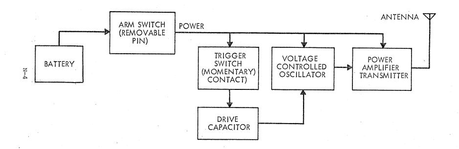
FIGURE N-1. NBB FUNCTIONAL BLOCK DIAGRAM
