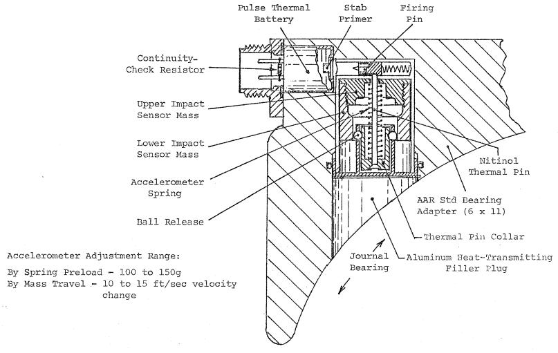
FIGURE 22. COMBINATION ROADBED-IMPACT AND THERMAL SENSOR
