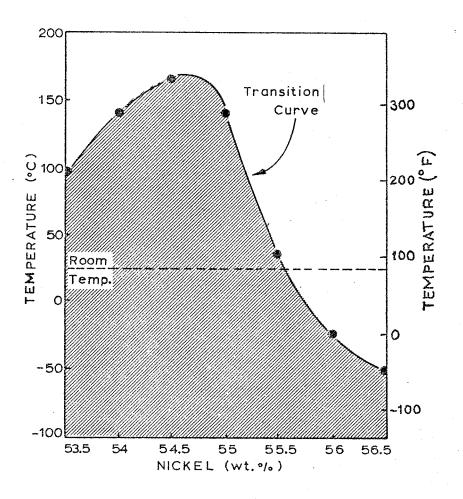
FIGURE 11. MARTENSITIC TRANSITION TEMPERATURE (T $_{\text{C}}$ ) CHANGE WITH MINOR VARIATIONS IN THE Ti:Ni RATIO
