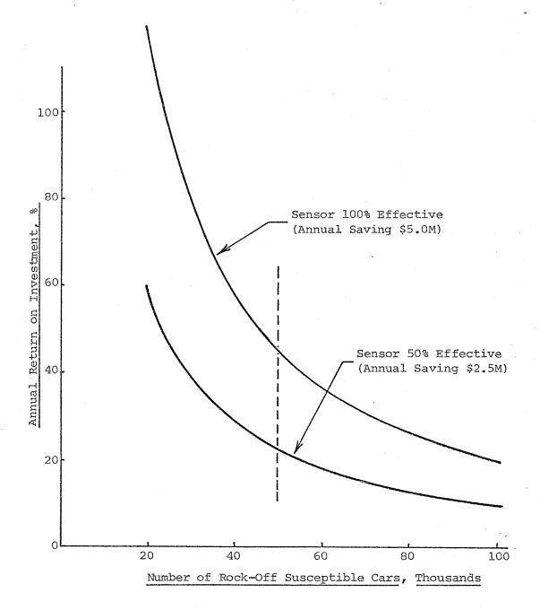
70 rock-off derailments per year (1970) \$70,000 average total cost per derailment Sensor incremental cost \$200 per car (installed) Sensor maintenance cost \$10 per car year
