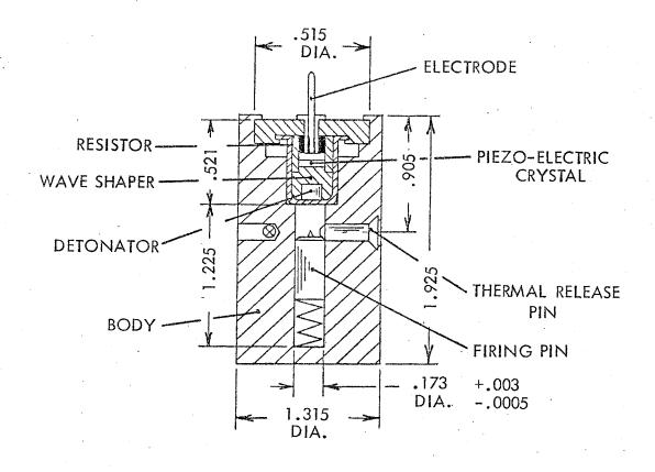
FIGURE 12. THERMAL SENSOR DESIGN - PIEZO-CRYSTAL OUTPUT
