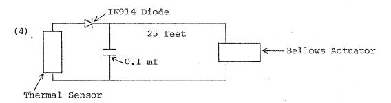
(Test attempt to match the high impedance of the thermal sensor crystal ( $\cong 200 \mathrm{K}\Omega$ ) with the low impedance ( $\cong 5\Omega$ ) of the bellows actuator and to release the crystal energy at the peak.)
