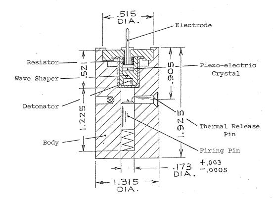
⊗ = Point of actuation-test temperature measurement
