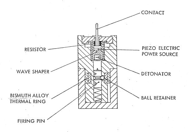
FIGURE 9. LOW-MELTING-ALLOY THERMAL SENSOR DESIGN - PIEZO CRYSTAL OUTPUT
