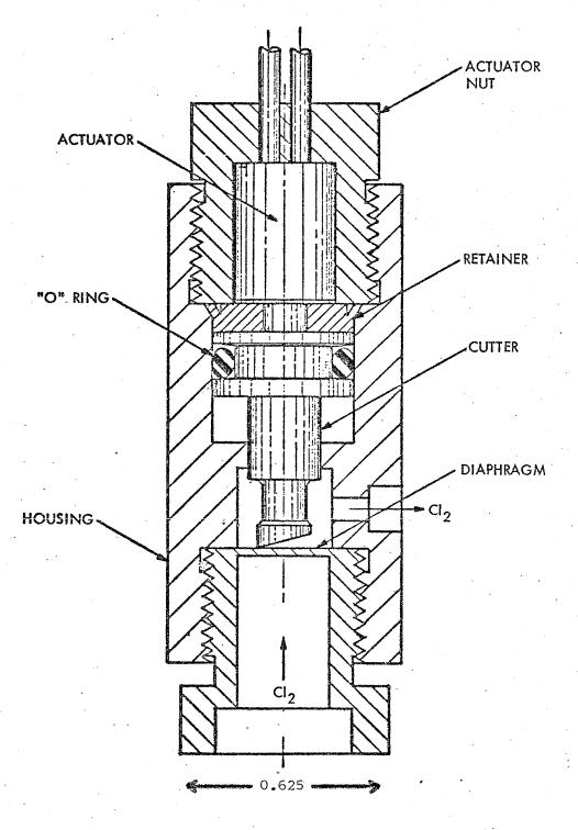
FIGURE 33. DIAPHRAGM CUTTER
