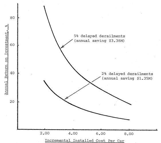
3000 miscellaneous road derailments per year (1970) \$75,000 average total cost per derailment (1970) Sensor effective on loaded car-miles only (60%) Sensor reduces average cost of delayed derailment by 50%
