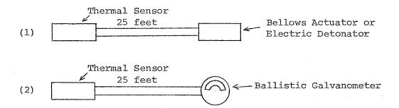
(Test to determine energy output from thermal sensor crystal after calibration of ballistic galvanometer.)
