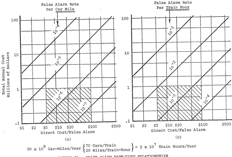
FIGURE 31. FALSE ALARM RATE/COST RELATIONSHIPS
