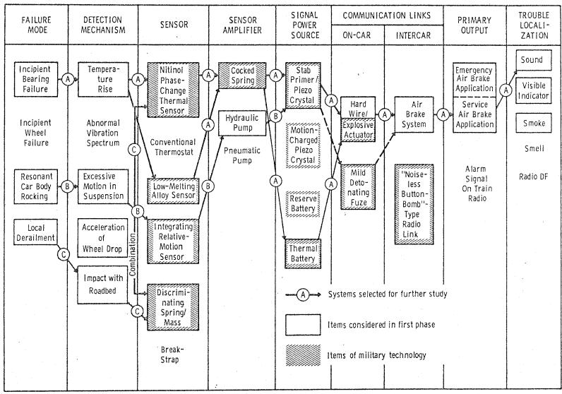
FIGURE 1. ANTI-DERAILMENT SENSOR STUDY MATRIX
