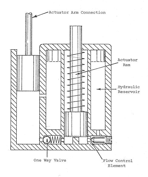
FIGURE 20. HYDRAULIC ACTUATOR WITH FLOW CONTROL ELEMENT
