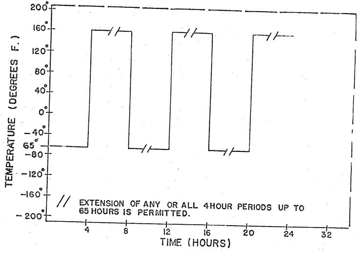
FIGURE 1. Thermal shock cycle.
