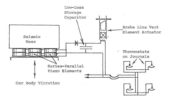
(a) Motion-Charged Piezo-Crystal Power Supply
