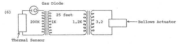
(Test attempt to match the high impedance of the thermal sensor crystal with the low impedance of the bellows actuator and to release the crystal energy at the peak.)
