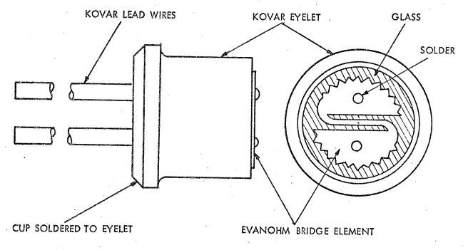
(As Used in Navy Detonator Mk 101)
