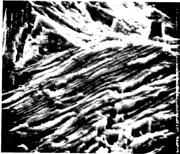
FIGURE 31. FRACTURE SURFACE OF SAMPLE 002 0.17 INCH FROM THE NOTCH TIP, \Delta K \approx 17 \text{ ksi-in.}^{\frac{1}{2}} Compare lines at 5000X with Figure 23(a).
