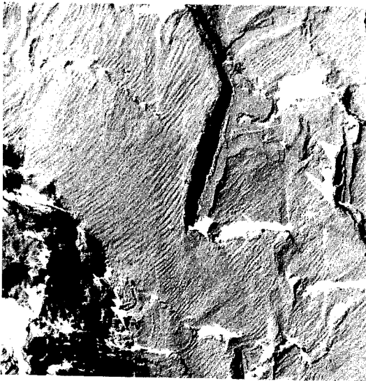
(a) Sample 004, 0.86 inch From Notch Tip, \Delta K \approx 29 \text{ ksi-in.}^{\frac{1}{2}}
