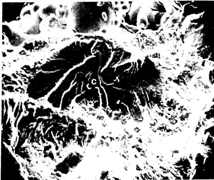
FIGURE 25. FRACTURE SURFACE OF SAMPLE 004 AT THE NOTCH TIP
