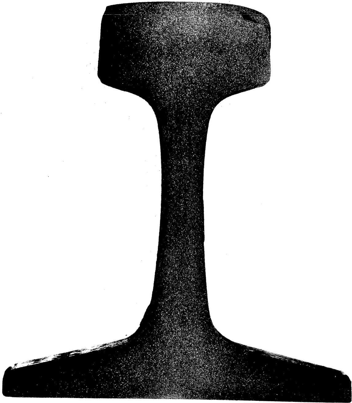
FIGURE 2. TYPICAL FINE-TEXTURED MACROSTRUCTURE OF RAILS - SAMPLE 019
