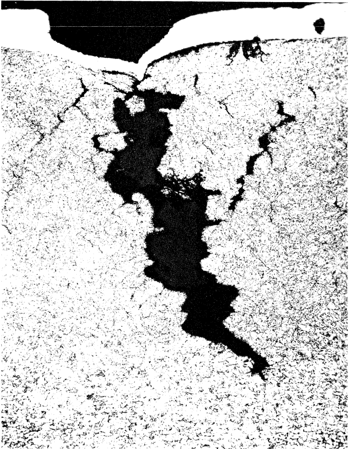
Figure 12. Secondary Crack on Tank Car I.D. Surface Arresting at Microstructure Interface
