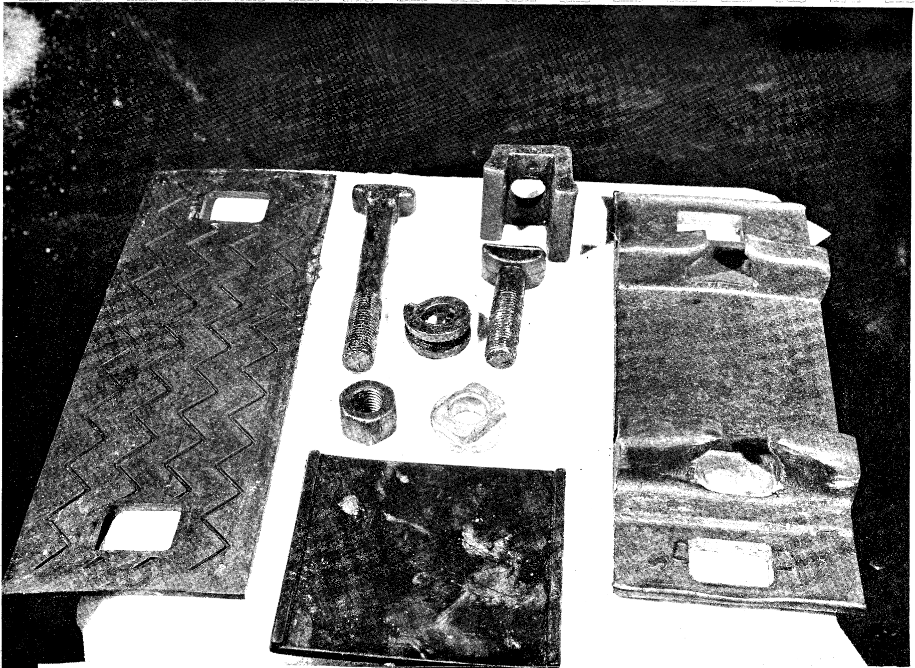
Figure 2-Tie "hardware" includes resilient tie plate pad, steel tie plate, resilient rail base pad, Tee head tie plate hold down bolts with steel nuts and double spiral lock washers, Tee head rail base hold down bolts with fibre washers and steel nuts and steel clips.
