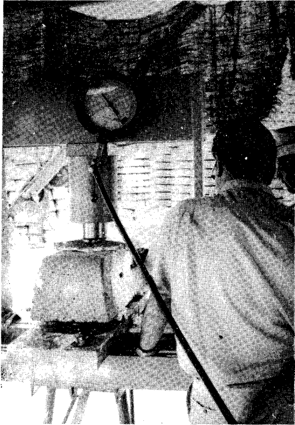
PLATE 13. BENDING TEST OF BLOCK IN NORMAL TIE POSITION
