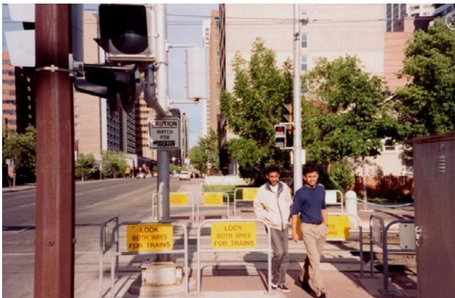
Figure 78. Bedstead Barrier Application
