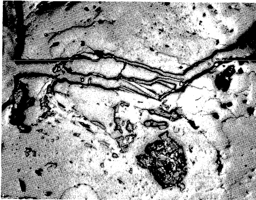
Figure 8a. Showing Part of the Notch and Extensive Side Cracking in Granite. 50X
