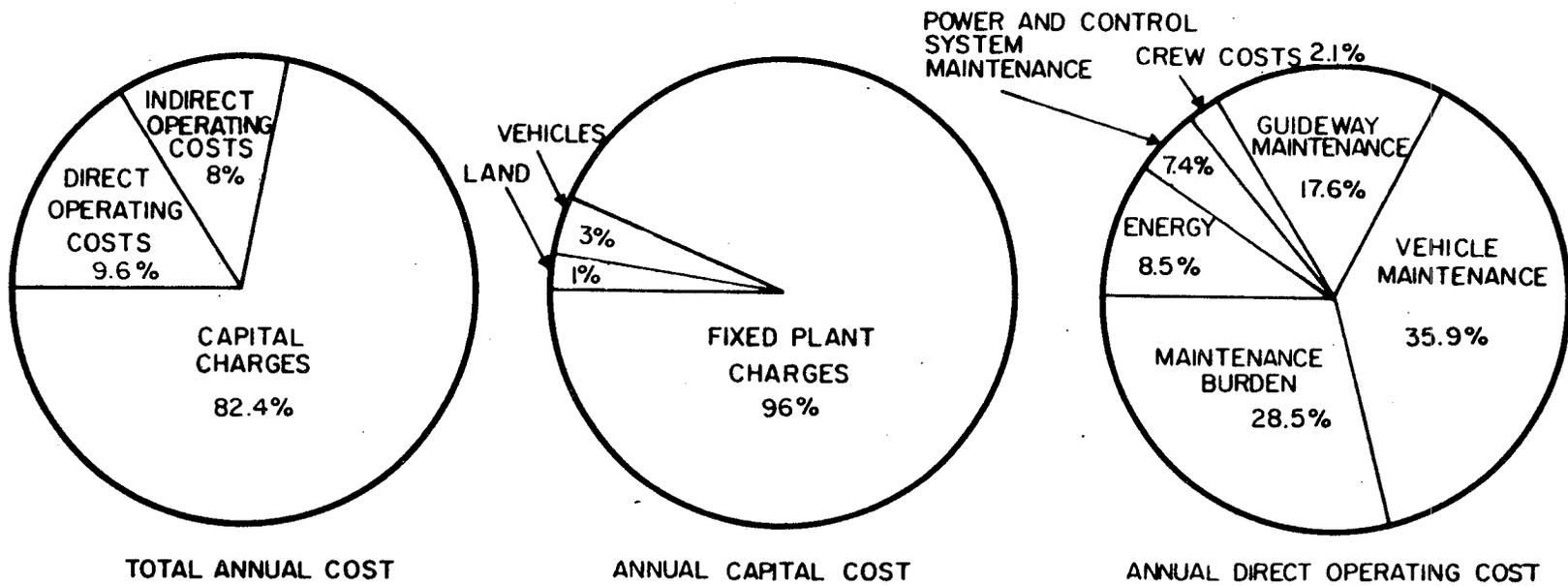
Figure 3-1. TVS Operating Cost Breakdown for Baseline System with VTOL Competition
