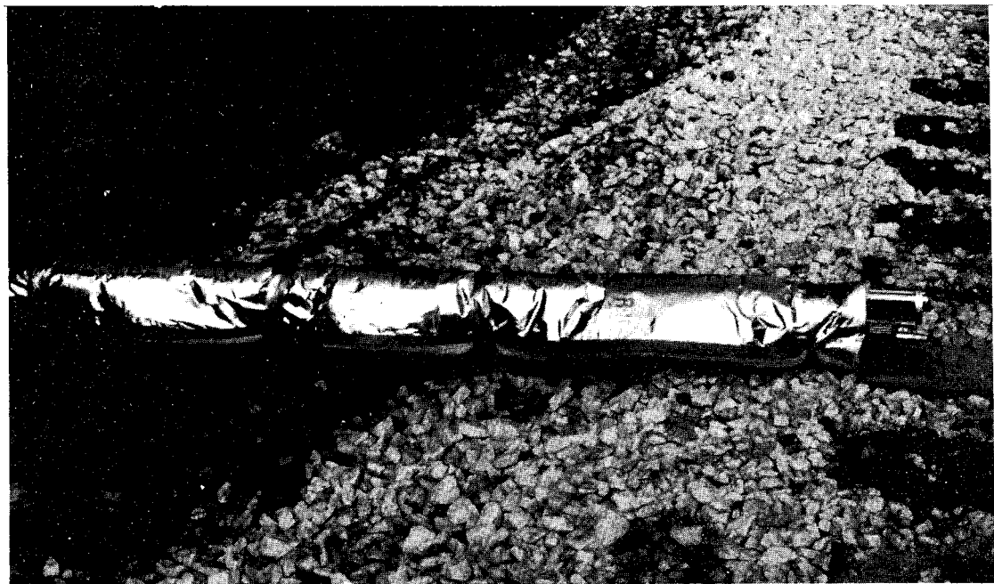
Figure 14. Typical Insulated Beam Holding Displacement Transducer Above Tie at Test Joint
