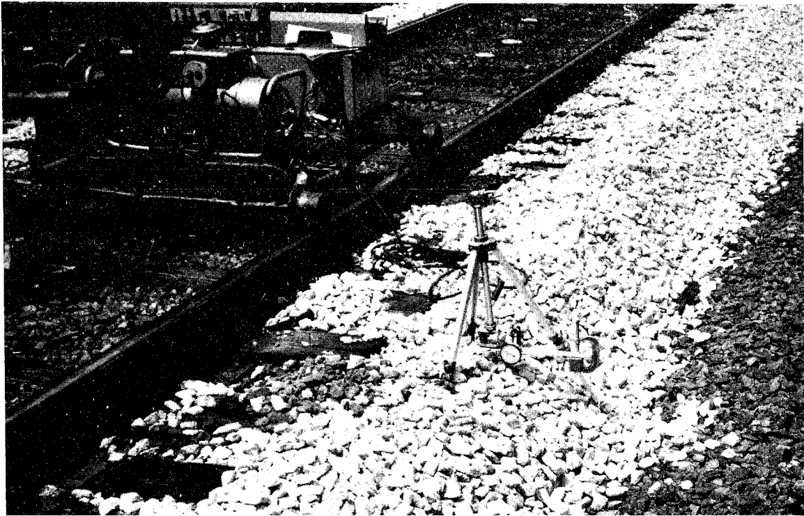
Figure C-6. Test Instrumentation Dial Gage and Displacement Transducer Used to Measure Lateral Displacement of Tie
