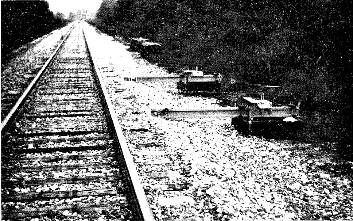
Figure C-9. Instrumentation for Measuring Vertical Movement of Test Tie
