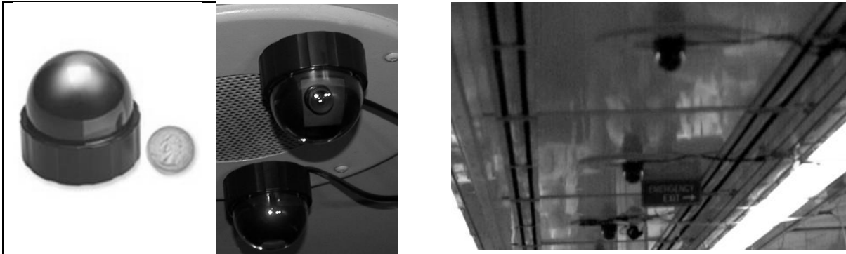
Figure 8. Miniature Video Cameras and Microphones Mounted on Seating Compartment Ceiling
