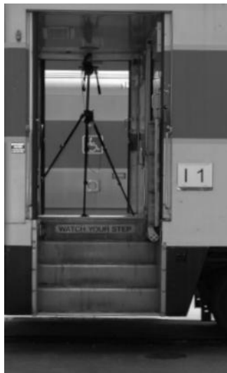
Figure 21. Car #515: Door Side Stairway – Interior and Exterior Video Cameras
