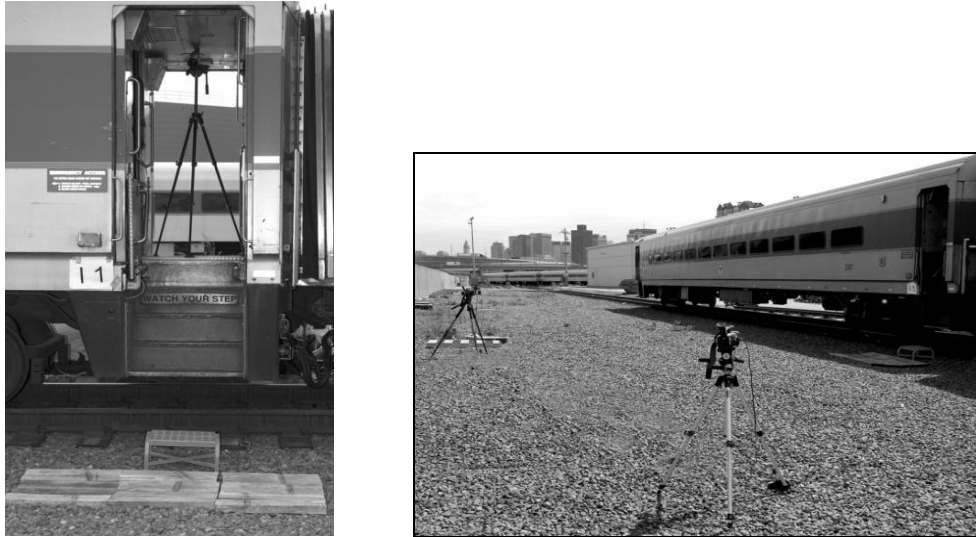
Figure 14. Car #237: Side Door Stairway – Interior and Exterior Video Cameras
