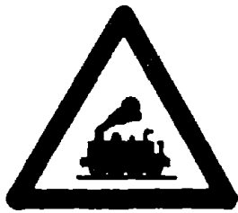
Level-crossing without gates
