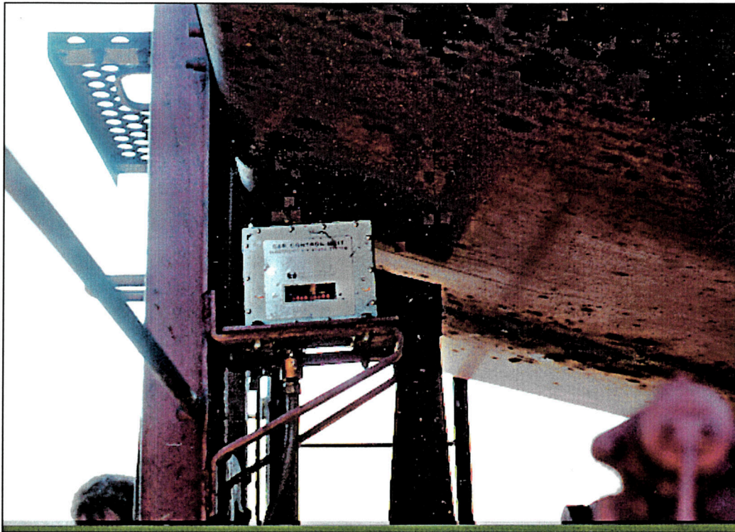
Figure 1. CCD Mounting on Conrail Coal Hopper
