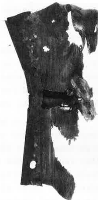
E. Front view—Second simulated wornout shoe after 3 stops.
