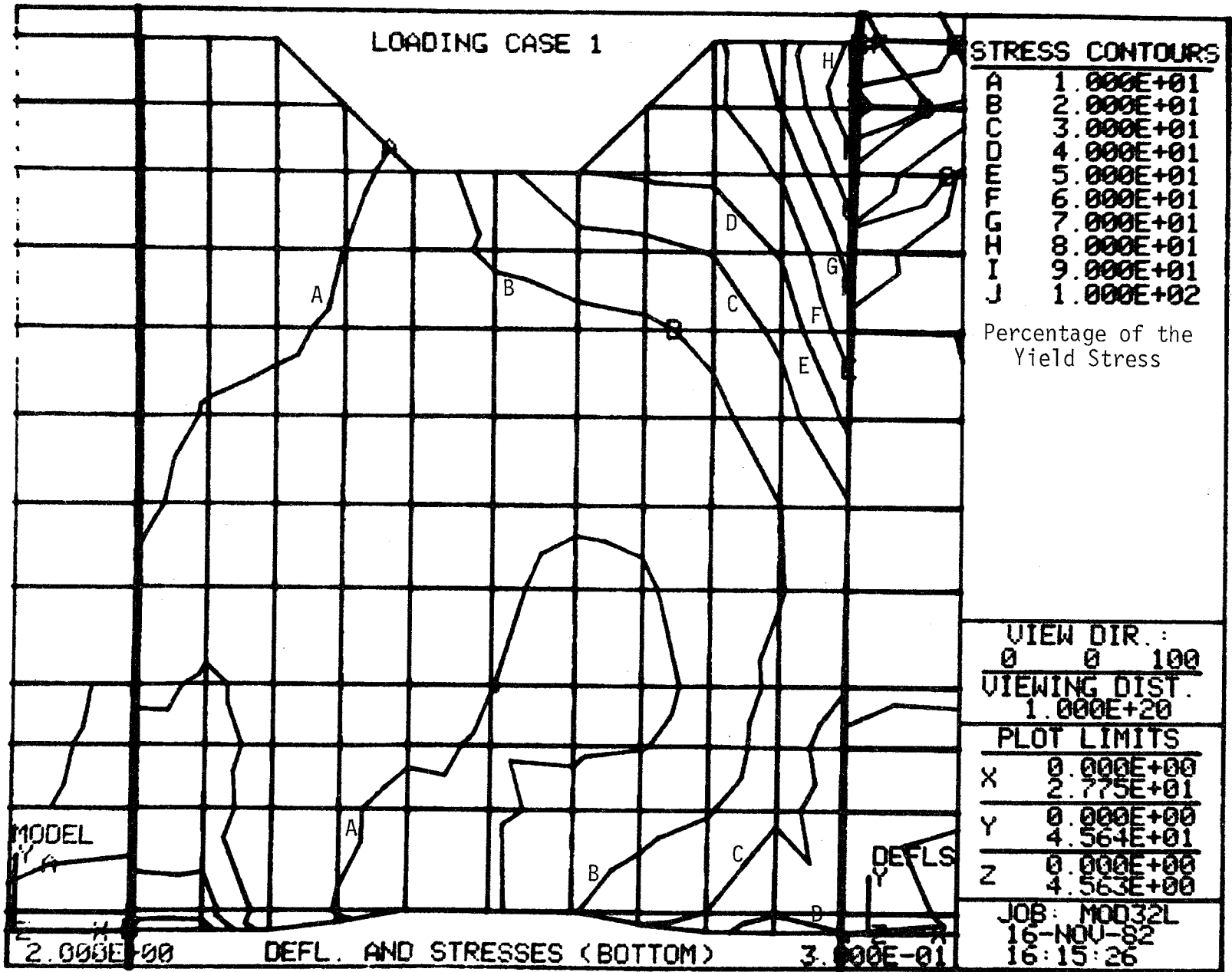
FIGURE 19b. ENLARGED VIEW OF STRESS CONTOUR FOR NON-UNIFORM LOAD.
