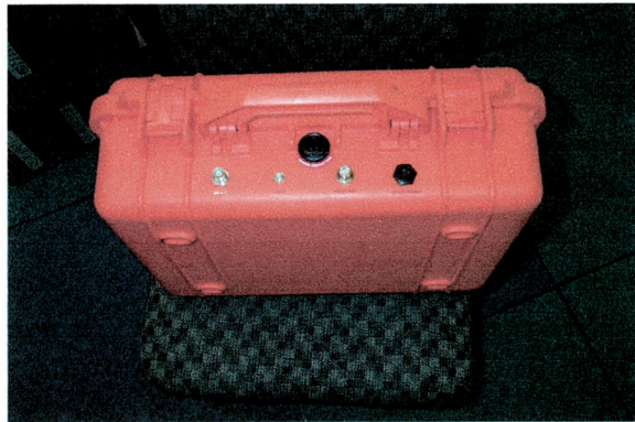
Figure 3. Portable Installation of Vehicle Tracking System Hardware (Courtesy of Radio Satellite Integrators, Inc.)
