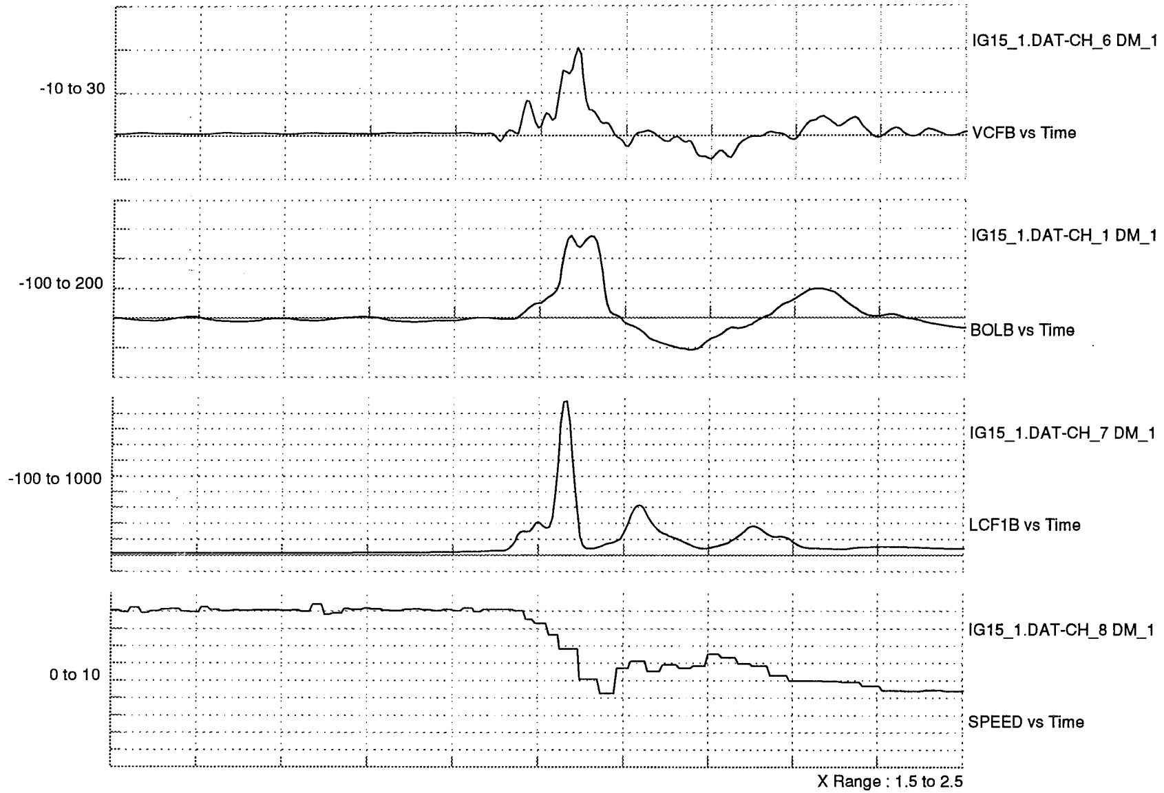
Figure 61. Surge Pressure Impact Test 9 mph Configuration A
