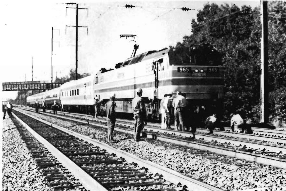
AMTRAK GENERAL ELECTRIC E-60 LOCOMOTIVE ALONG WITH THE FRA TEST CAR T-7 AND BUDD COMPANY AMCOACHES IN TEST ON NEC MILE POST 44.2, SEPTEMBER 28, 1976
