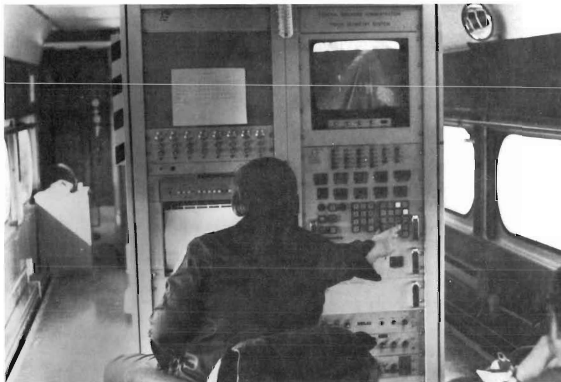
TRACK GEOMETRY INSPECTION INSTRUMENTATION SYSTEM
