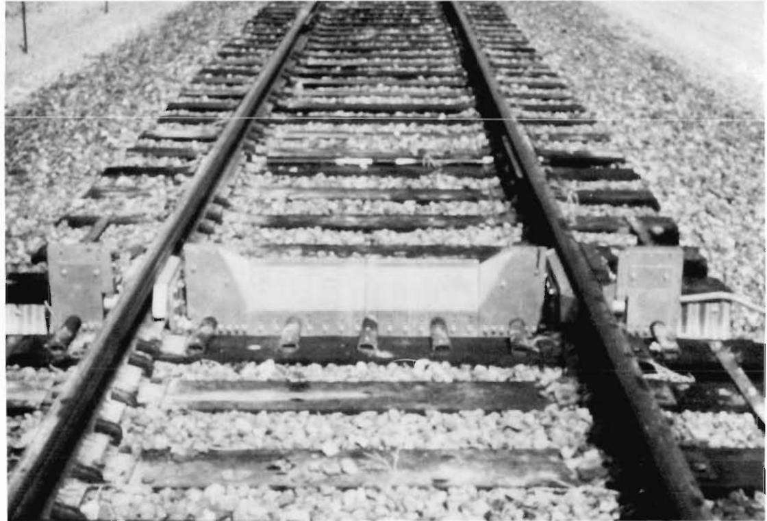
DRAGGING EQUIPMENT DETECTOR
