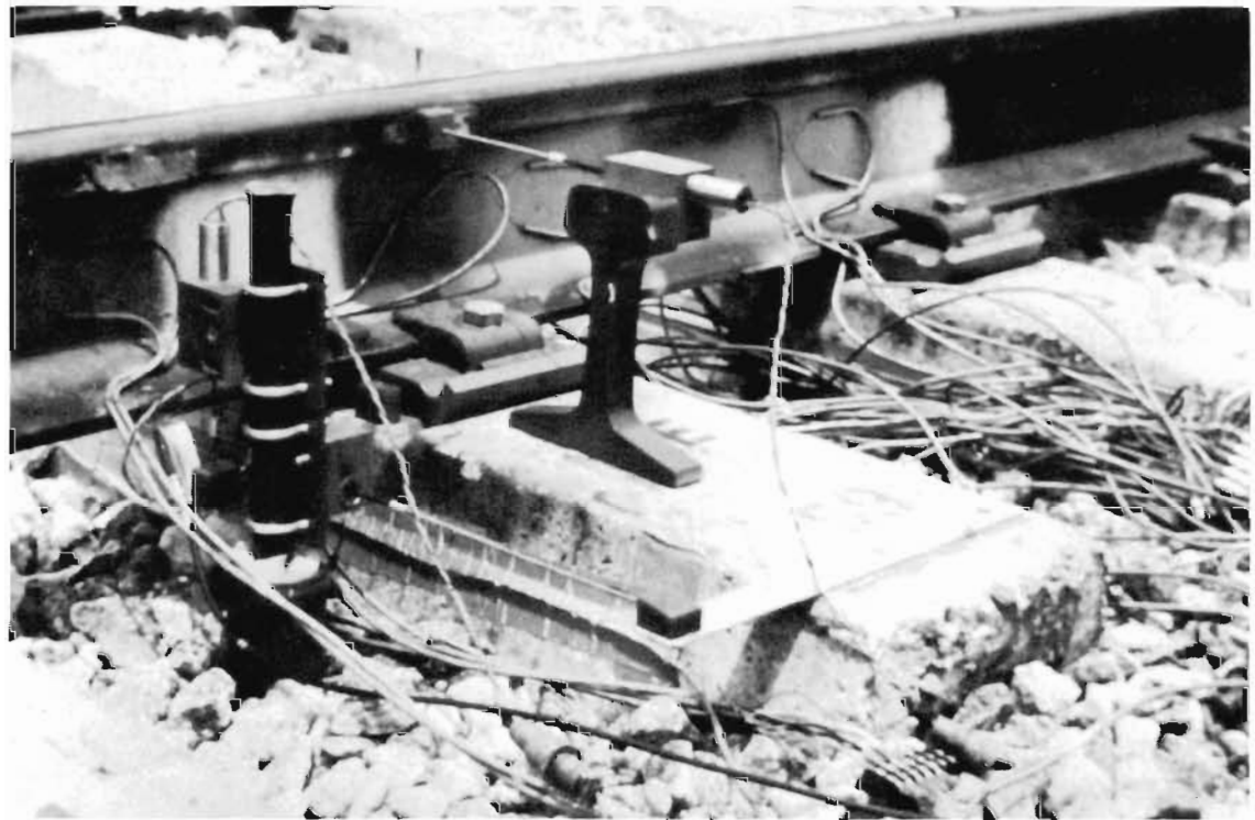
DEVICE WHICH MEASURES SERVICE LOADS FOR CONCRETE TIE AND TRACK WHICH IS UTILIZED FOR LONG TERM PERFORMANCE MEASUREMENT
