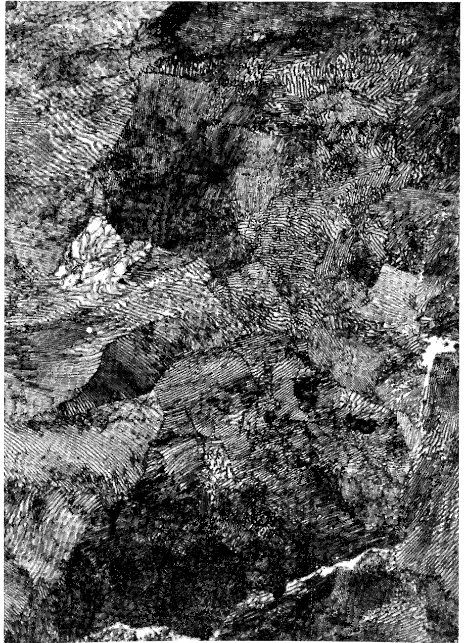
Figure B-4 Typical Structure in The Interior of Rail Head 8. (100X, Vilella's Etch)
