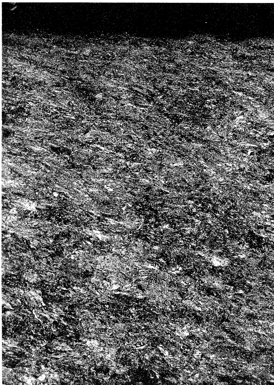
Figure B-7 Section Through The Top of The Used Rail Head 7. (100X, Nital Etch)
