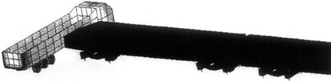
View of the DUPLEX TGV impacting a 38 ton truck
