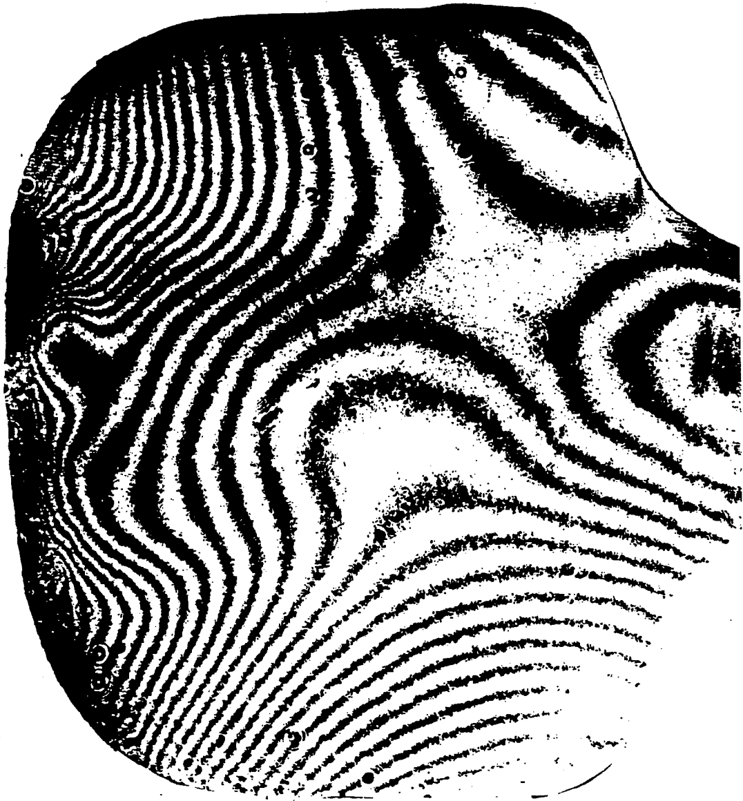
Fig. 66 w-field fringes by Twyman/Green interferometry (rail # 5 new CFI, 45° oblique slice)
