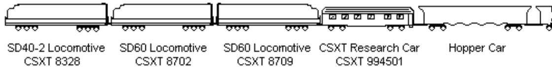
Figure 1-4. Test Consist Used for TOR Lubrication Evaluation Test
