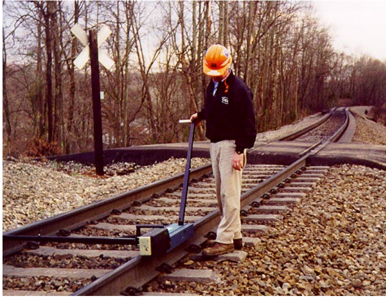
Figure 2-5. CSXT Personnel Using Tribometer
