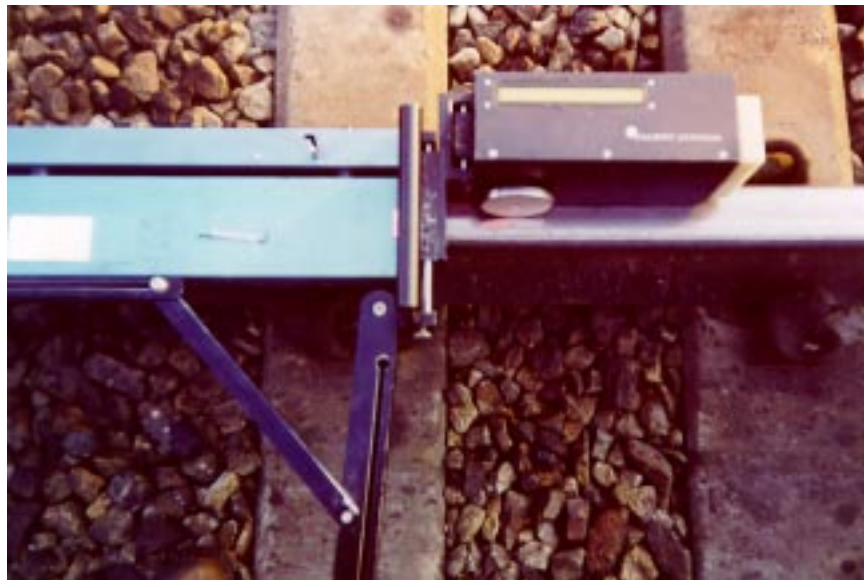
Figure 2-4. Tribometer Used for Determination of Friction Coefficients
