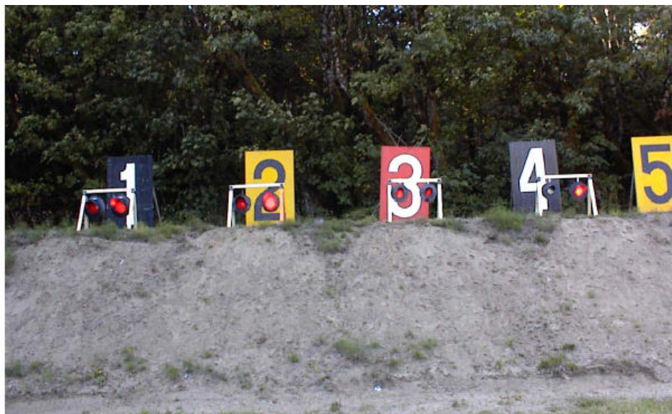
Figure 85. Field testing set-up of signal lights (Green and Milanovic, 2002).
