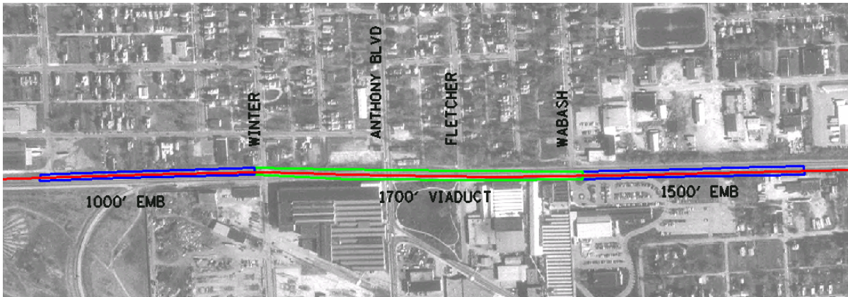
Exhibit 2-6: Alignment through Downtown Ft. Wayne, Showing Embankment and Viaduct Over Grade Crossings to Move from North Side to South Side
