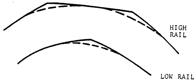
Figure 4-6. Tendency of High Rail to Go Out at Joints and Low Rail to Come In at Joints
