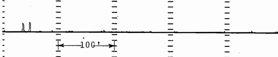
Figure C.1.a.5. Crosslevel and Profile Cusps at a Switch (Class 6, Tangent).
