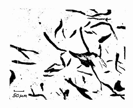
FIGURE 17. MICROSTRUCTURE OF WABCO DISC BRAKE TANG. NOTICE THE SIMILARITY TO THE MICROSTRUCTURE OF THE DISC FIG. 18. MAGNIFICATION 200X
