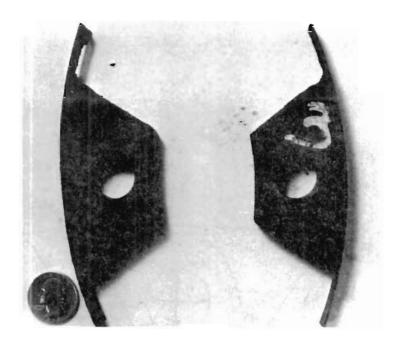
FIGURE 11. WABCO BRAKE DISC TANGS AS RECEIVED. SHOWN ARE THE STAMPED (left) AND PAINTED (right) SIDES OF HOLES NUMBER 2 AND 3. THE SIDE WITH THE LARGE PAINTED THREE IS THE OUTSIDE SURFACE WHILE THE OTHER HOLE SHOWS THE SURFACE THAT WAS IN CONTACT WITH THE HUB.
