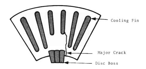
FIGURE 8. KNORR DISC CROSS-SECTION SHOWING LOCATION OF MAJOR CRACK NEAR HUB-DISC CONNECTION.
