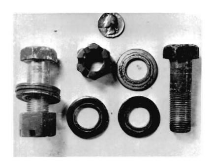
FIGURE 10. WABCO BOLTS AS RECEIVED. NOTE SURFACE CONDITION BEING FAIRLY SMOOTH WITH NO APPARENT WEAR.
