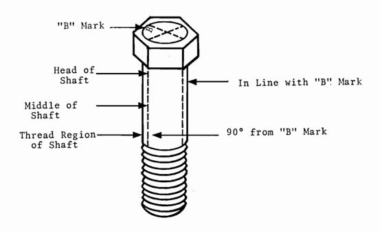
FIGURE 13. DIAGRAM OF CONNECTING BOLT
