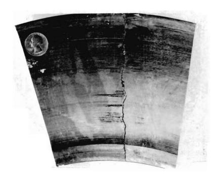
FIGURE 2. KNORR DISC BRAKE WITH HEAT CHECKS (minor cracks) AND MAJOR CRACKS. THE CRACK RUNS FROM THE INNER RADIAL EDGE (lower part of photograph) TO THE OUTER RADIAL EDGE (upper part of photograph).
