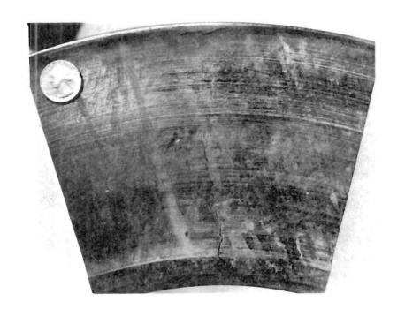
FIGURE 3. KNORR DISC BRAKE WITH MAJOR CRACK WITH OPEN END AT THE INNER RADIAL EDGE.
