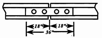
Each rail joins in Classes 3 through 5 track shall be supported by either at least one crossie specified in paragraphs (c) and (d) of this section whose centerline is within 36' shown above, or:
