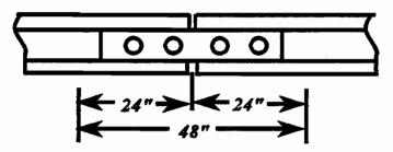
Two crossties, one on each side of the rail joint, whose centerlines are within 24" of the rail joint location shown above.
