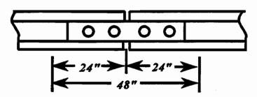
Each rail joins in Classes 1 and 2 track shall be supported by at least one crosstie specified in paragraphs (c) and (d) of this section whose centerline is within 48" shown above.
