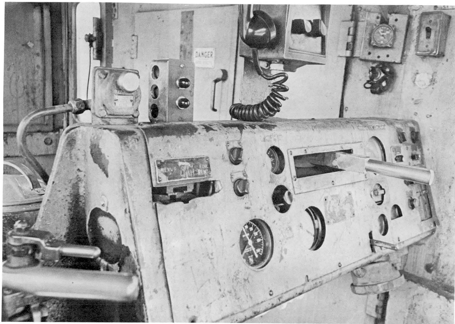
Fig. 2.33 Control stand in an EMD S-90 switcher, manufactured in 1943 but still in operation
