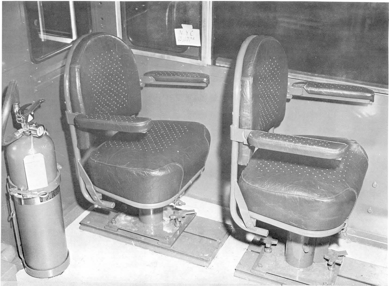
Fig. 1.12 Two auxiliary floor-mounted arm chairs on a U28B GE Locomotive of New York Central Railroad
