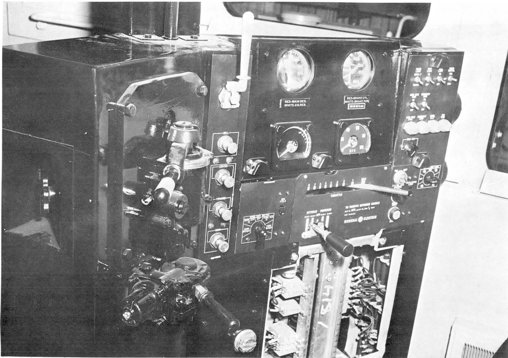
Fig. 2.13 Two-lever control stand was used on U23, U33 GE locomotives
