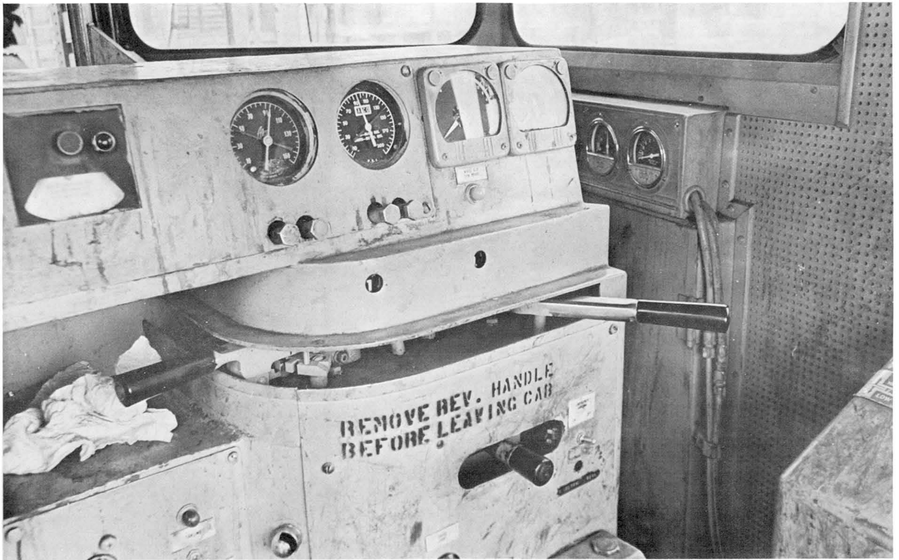
Fig. 2.26 Late model ALCO control stand (C630, 1966 production) Note indicator gauges behind control stand on front wall.
