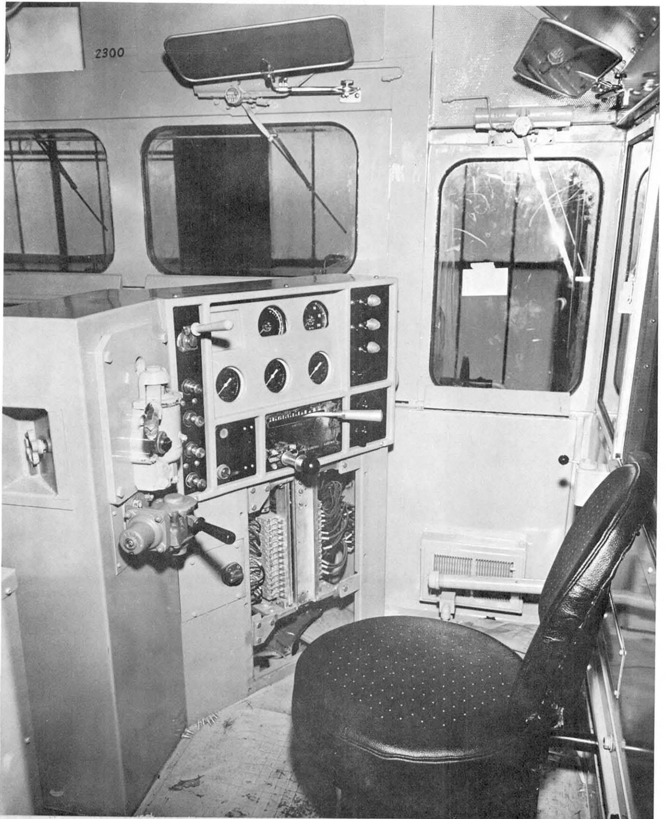
Fig. 2.23 Modification of the two level GE control stand (U23 model, Lake Superior & Ishpeming Railroad)
