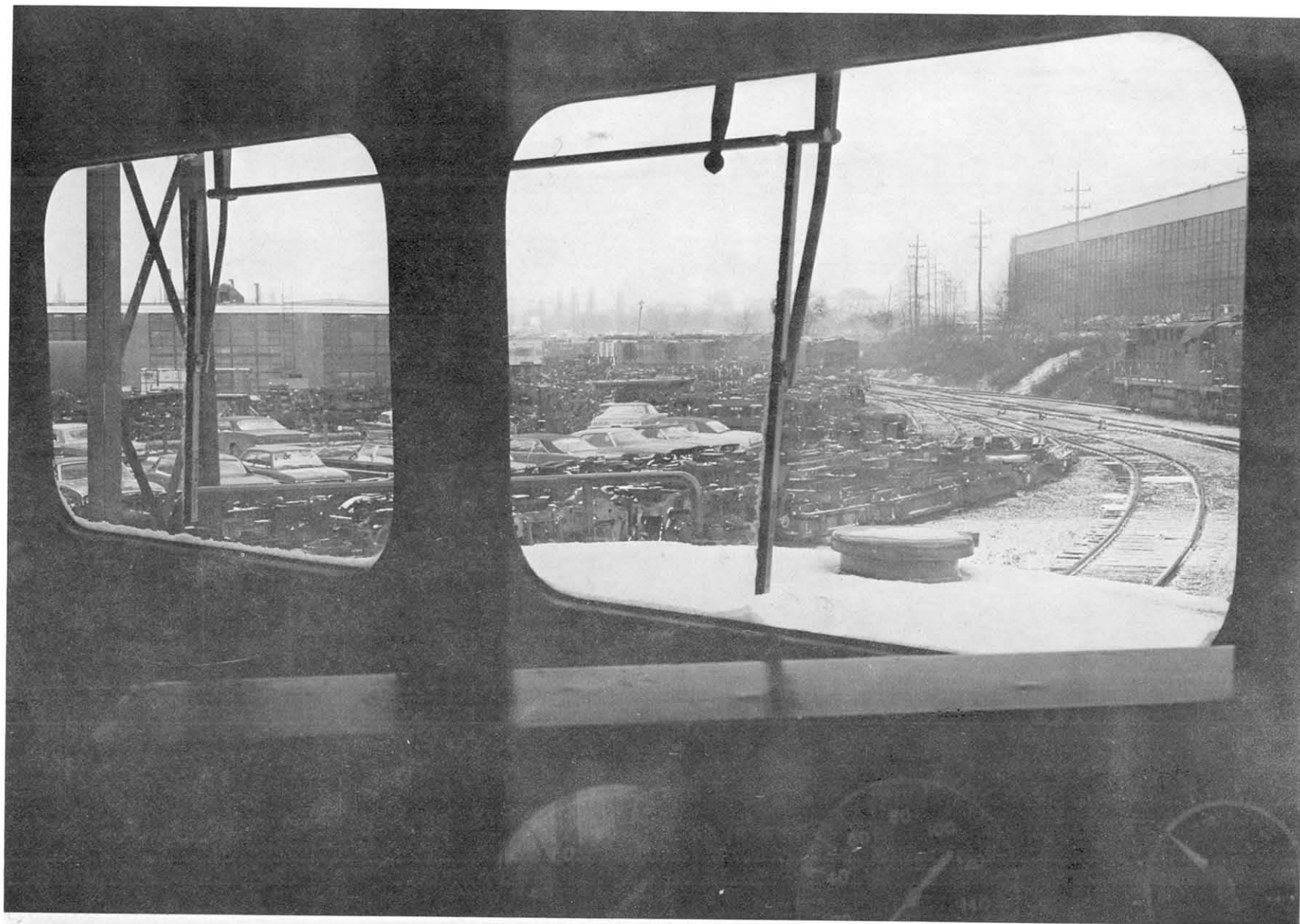
Fig. 1.18 View through the two horizontal front windows above the short hood from the engineer's seat on a U30C GE locomotive
