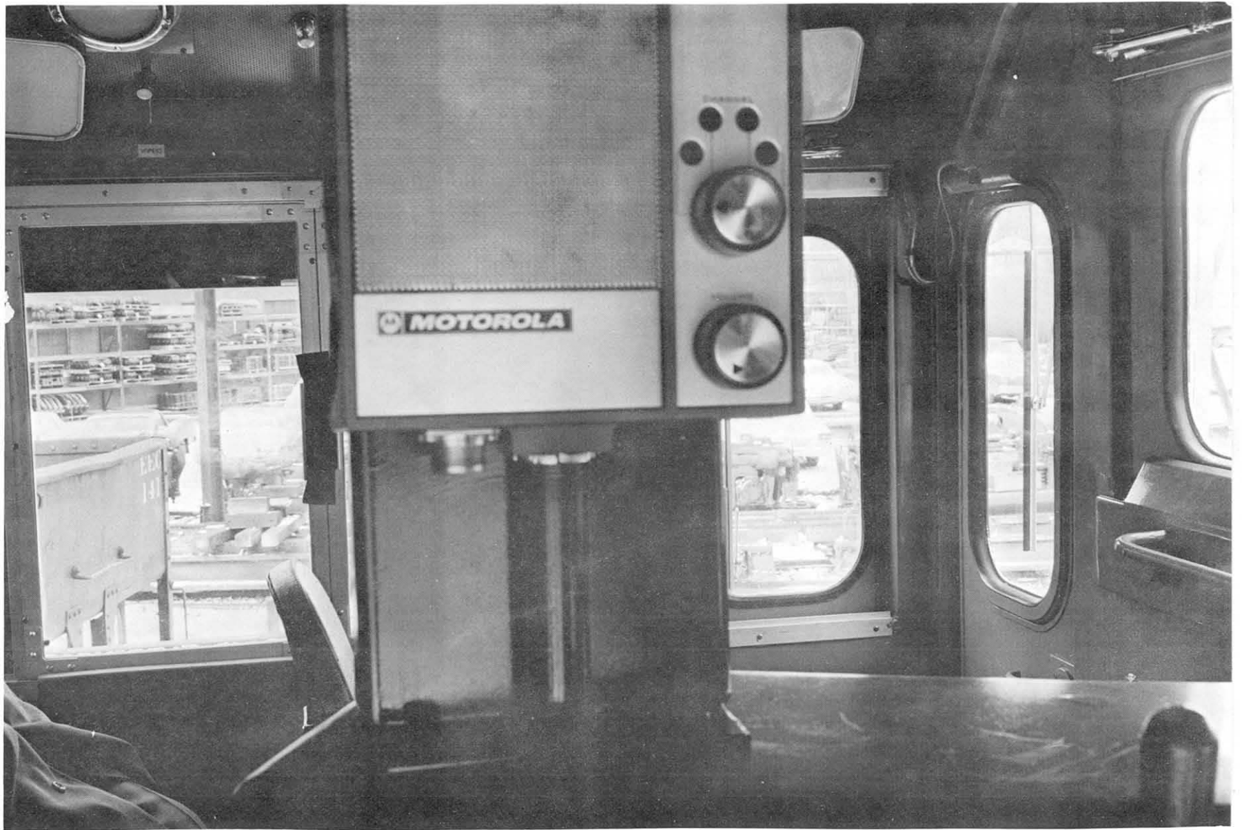
Fig. 1.19 View to the left side from the engineer's seat with the radio obstructing the visual field above the control stand
