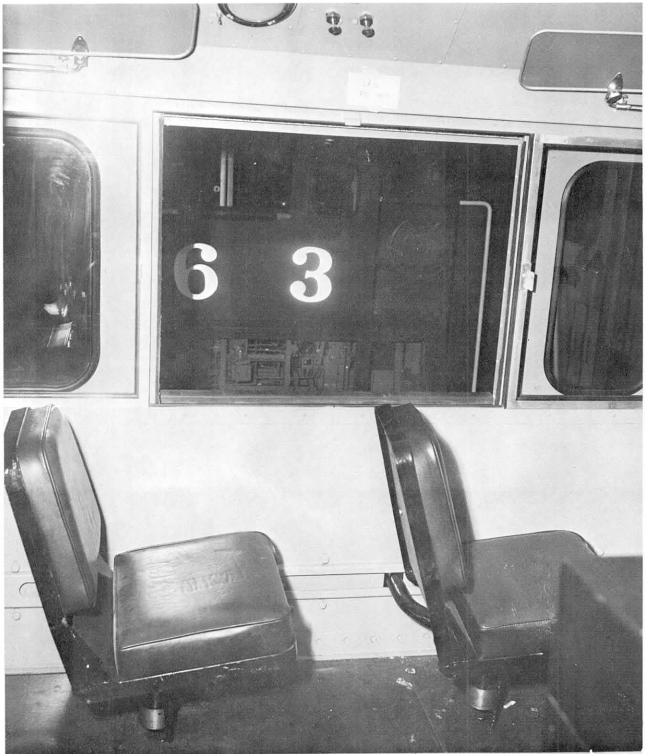
Fig. 1.11 Two auxiliary special seats on a GE U30 locomotive of Louisville and Nashville Railroad
