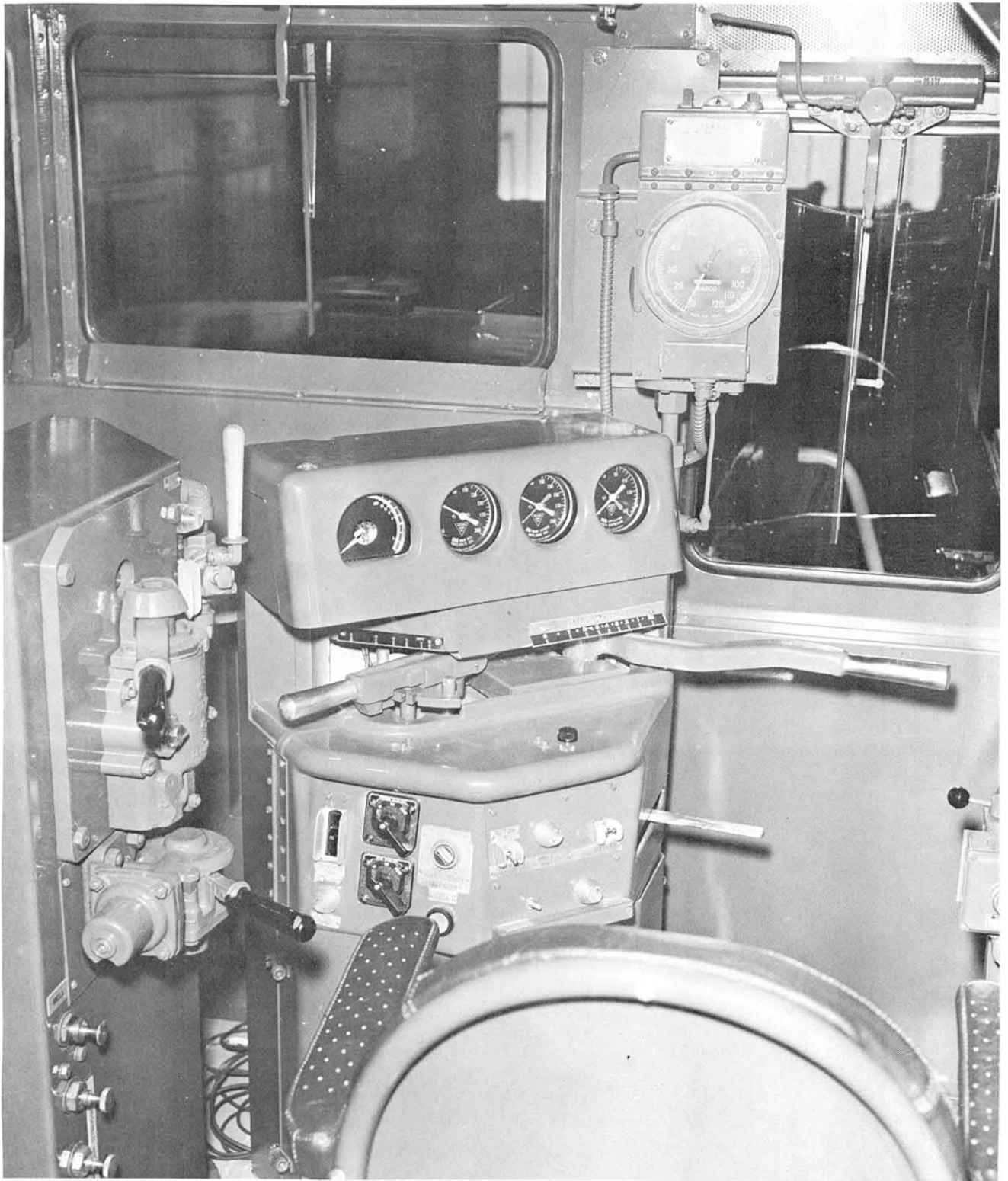
Fig. 2.12 Three-lever control stand was used on U25, U28, U30 GE locomotives
