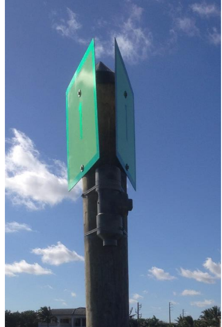
Figure 4. Installed camera housing
