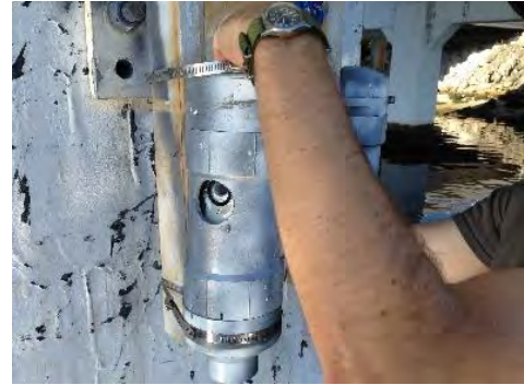
Figure 2. Custom 4" PVC housing
