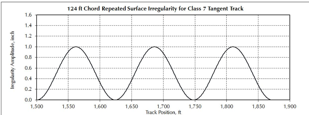
**Figure 8. Repeated Surface Irregularity Profiles**
