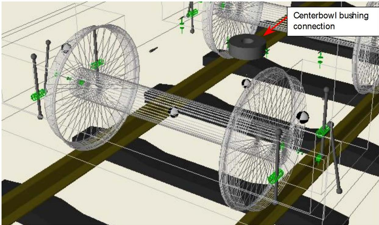
**Figure 5. Vehicle dynamics model of truck showing connections**
