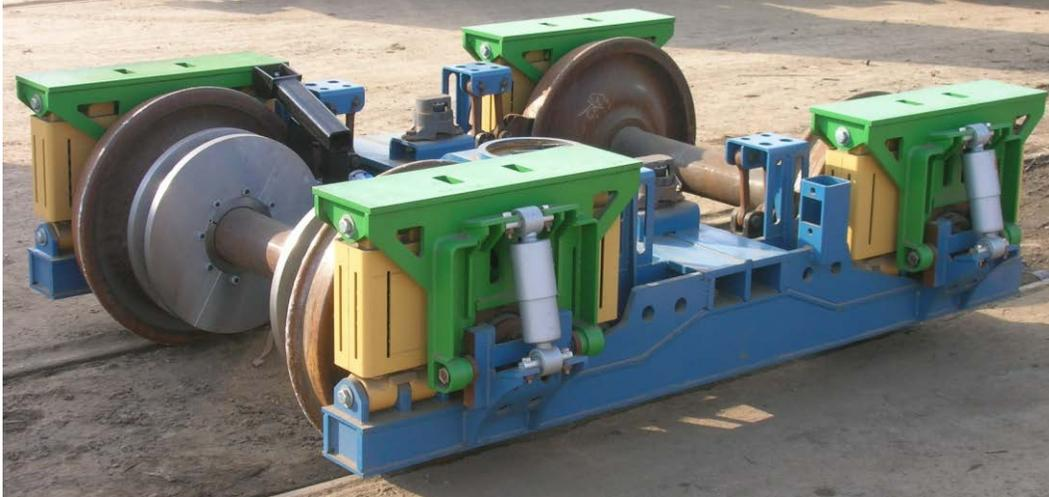
**Figure 2. Prototype HST Used for Fitment and Yard On-Track Testing**
