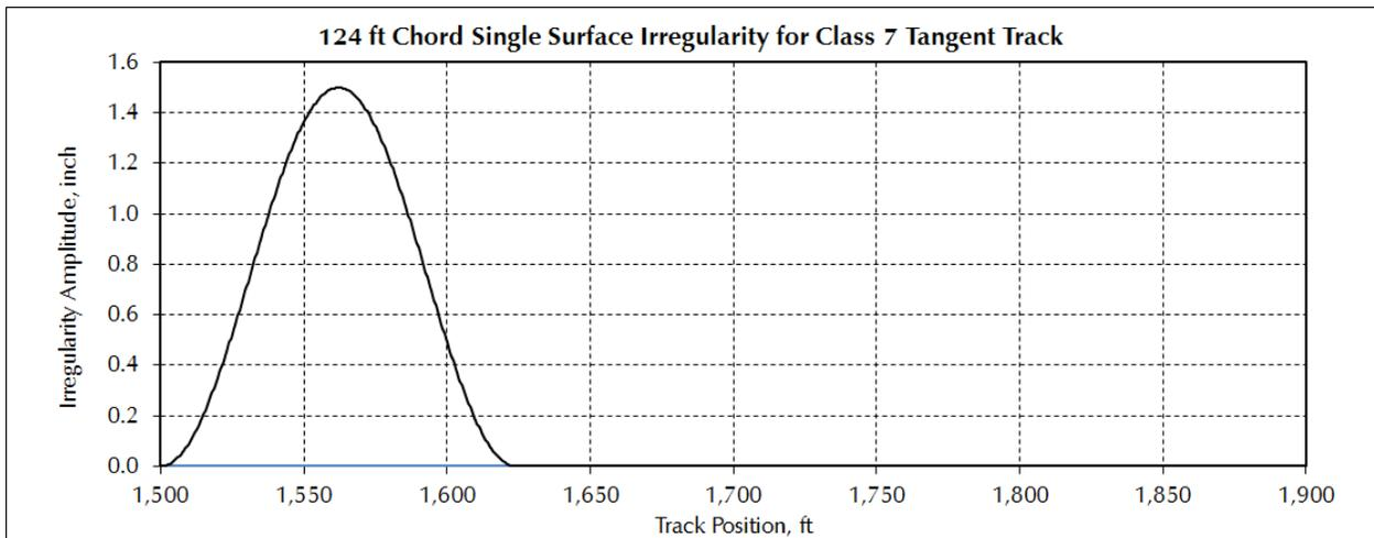
**Figure 7. Single Surface Irregularity Profiles**
