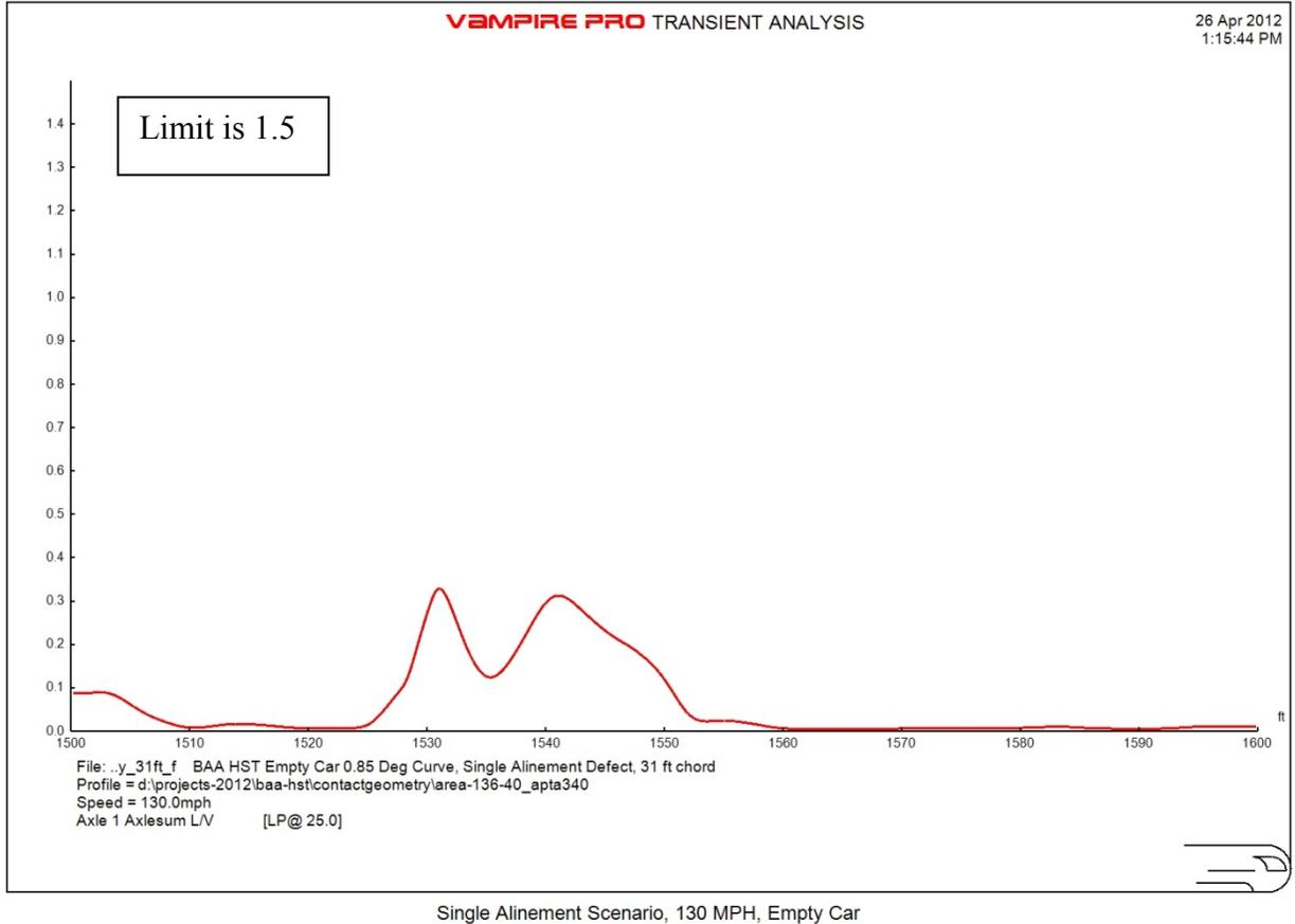
**Figure 10. Axle sum L/V ratio on axle 1, left wheel**
