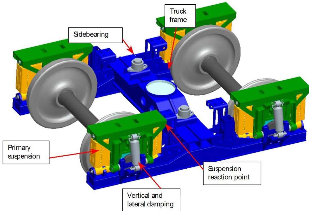
**Figure 4. 3D CAD Model showing the key structural components of the truck**
