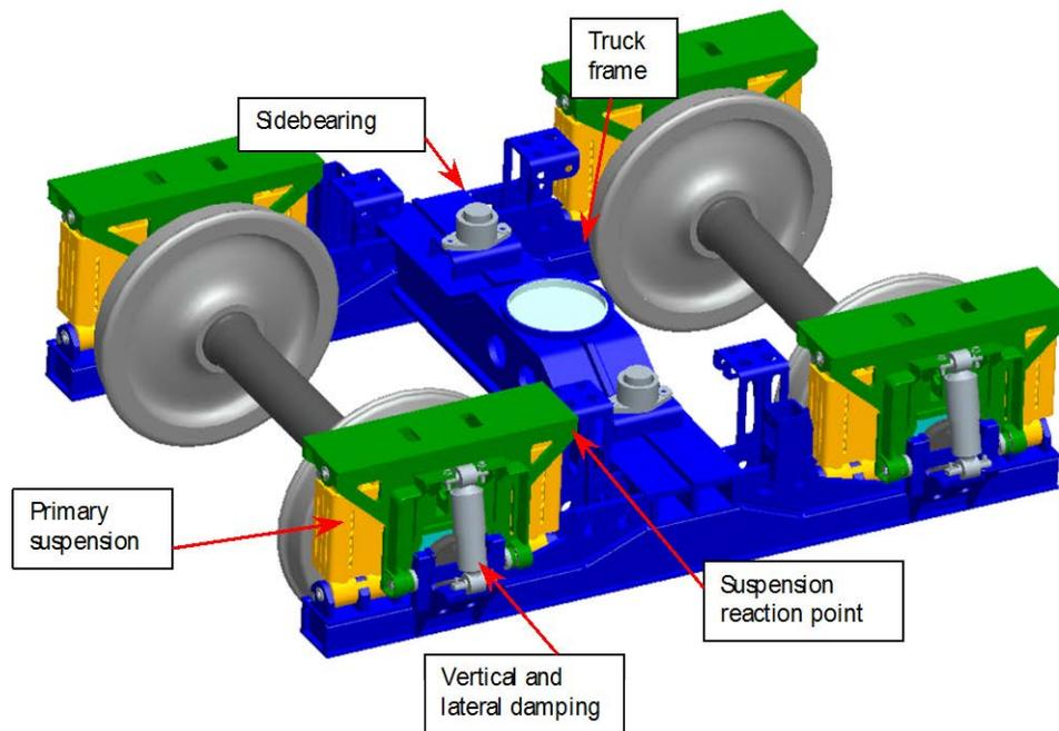
**Figure 1 CAD Model of the Prototype HST**
