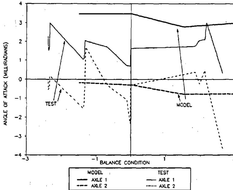
**Figure 104. Axle Angles of Attack for the Empty Car in the 4-Degree Curve**
