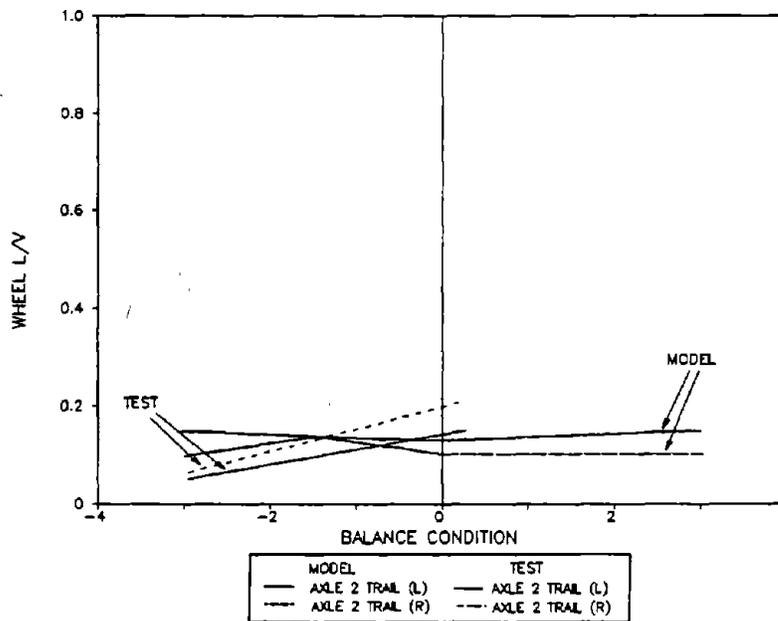
**Figure 122. Maximum Wheel L/V Ratios for Axle 2 of the Loaded Car in the Bunched Entry Spiral to the 12-Degree Curve**
