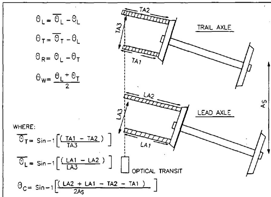
**Figure 25. Diagram Showing Schematic for Determining Axle Alignment Measurement**
