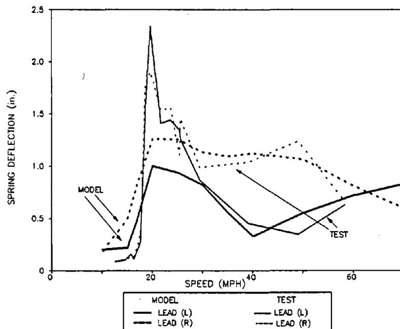
**Figure 97. Maximum Peak to Peak Vertical Spring Deflections for the Lead Truck of the Loaded Car in the Twist and Roll Test Zone**
