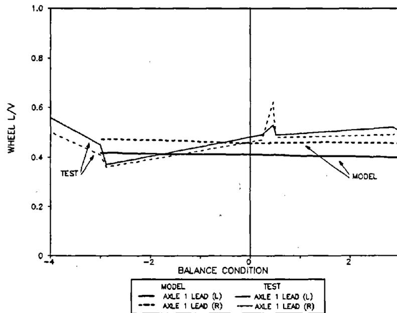
**Figure 125. Maximum Wheel L/V Ratios for Axle 1 of the Loaded Car in the Bunched Exit Spiral of the 12-Degree Curve**
