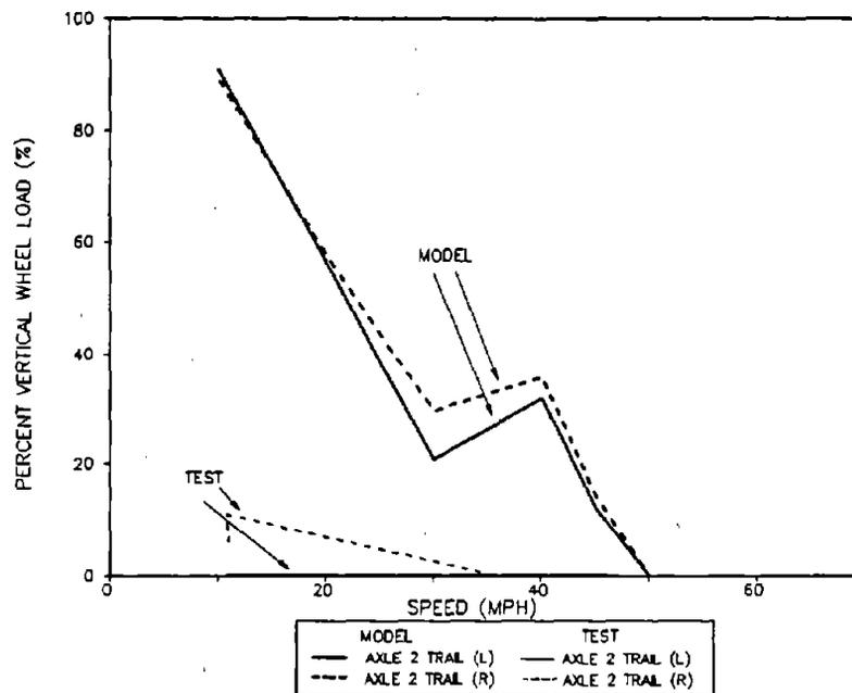
**Figure 83. Minimum Percent Vertical Wheel Loads for Axle 2 of the Empty Car Passing over the Single Bump**
