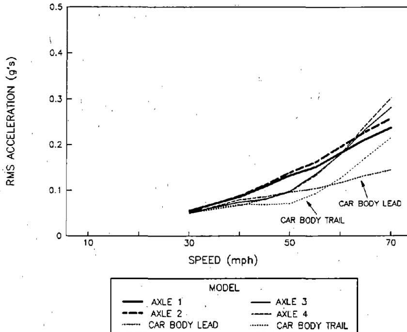
**Figure 74. Predicted RMS Lateral Accelerations for the Loaded Car while Hunting on a 50-Minute Curve**
