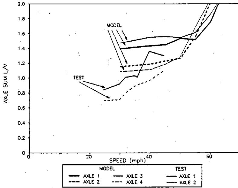
**Figure 102. Maximum Axle Sum L/V Ratios for the Loaded Car in the Yaw and Sway Test Zone**
