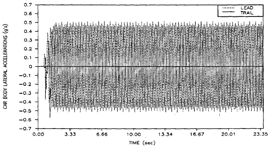
**Figure 26. Pre-test Predictions of Lateral Car Body Acceleration for the Empty Car While Hunting at a Speed of 57.5 mph Tangent Track**
