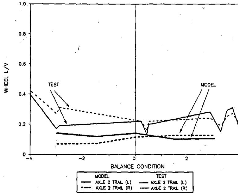
**Figure 126. Maximum Wheel L/V Ratios for Axle 2 of the Loaded Car in the Bunched Exit Spiral of the 12-Degree Curve**
