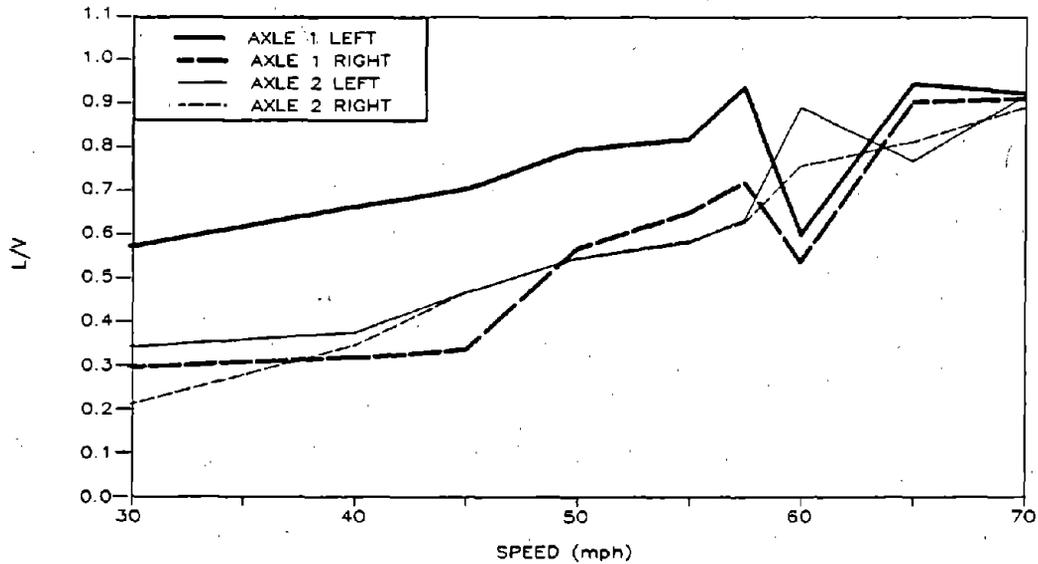
**Figure 28. Pre-test Predictions of Maximum Wheel L/V Ratio Versus Speed for the Empty Car on Tangent Track**
