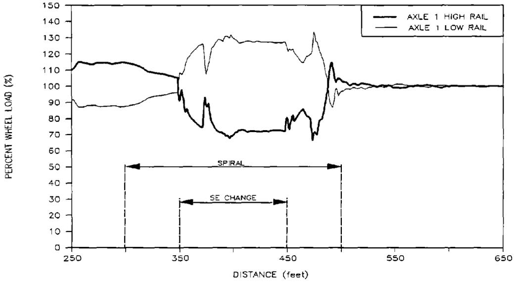
**Figure 52. Pre-test Predictions of Minimum Percent Wheel Vertical Load for the Empty Car Exiting the Bunched Spiral to Tangent Track at 31.1 mph**
