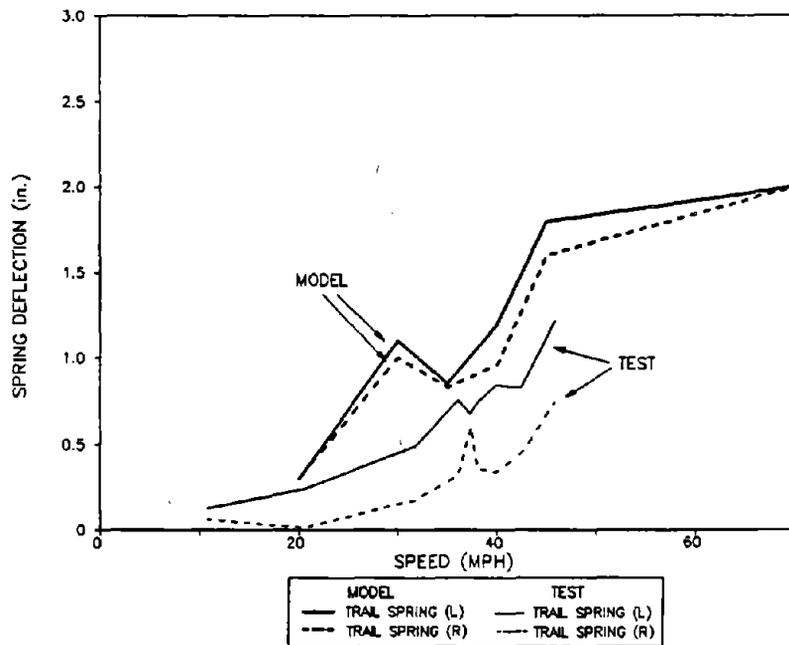
**Figure 89. Maximum Peak to Peak Vertical Spring Deflections for the Trail Truck of the Loaded Car Passing over the Single Bump**
