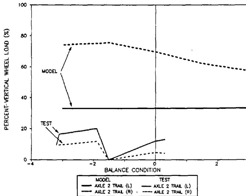
**Figure 116. Minimum Percent Vertical Wheel Load for Axle 2 of the Empty Car in the Bunched Entry Spiral to the 12-Degree Curve**
