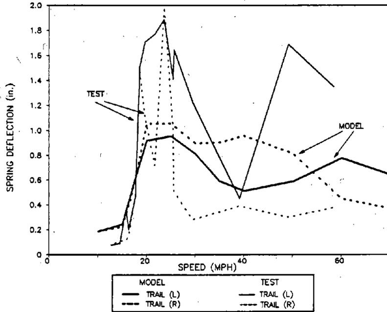
**Figure 98. Maximum Peak to Peak Vertical Spring Deflections for the Trail Truck of the Loaded Car in the Twist and Roll Test Zone**
