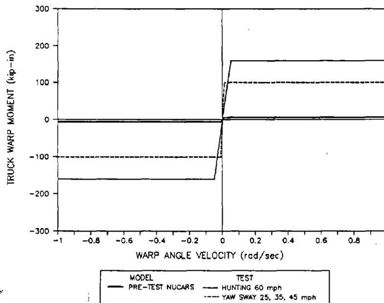
**Figure 64. Extrapolated Average Truck Warp Friction Damping Characteristics for the Loaded Car in Several Different Test Conditions**
