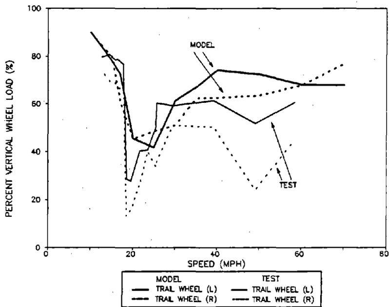
**Figure 96. Minimum Percent Vertical Wheel Loads for Axle 2 of the Loaded Car in the Twist and Roll Test Zone**
