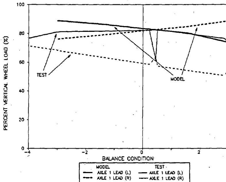
**Figure 127. Minimum Percent Vertical Wheel Load for Axle 1 of the Loaded Car in the Bunched Exit Spiral of the 12-Degree Curve**
