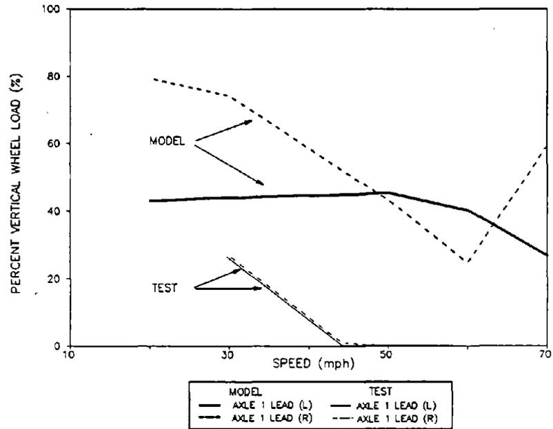
**Figure 76. Minimum Percent Vertical Wheel Load for Axle 2 of the Empty Car in the Pitch and Bounce Test Zone**
