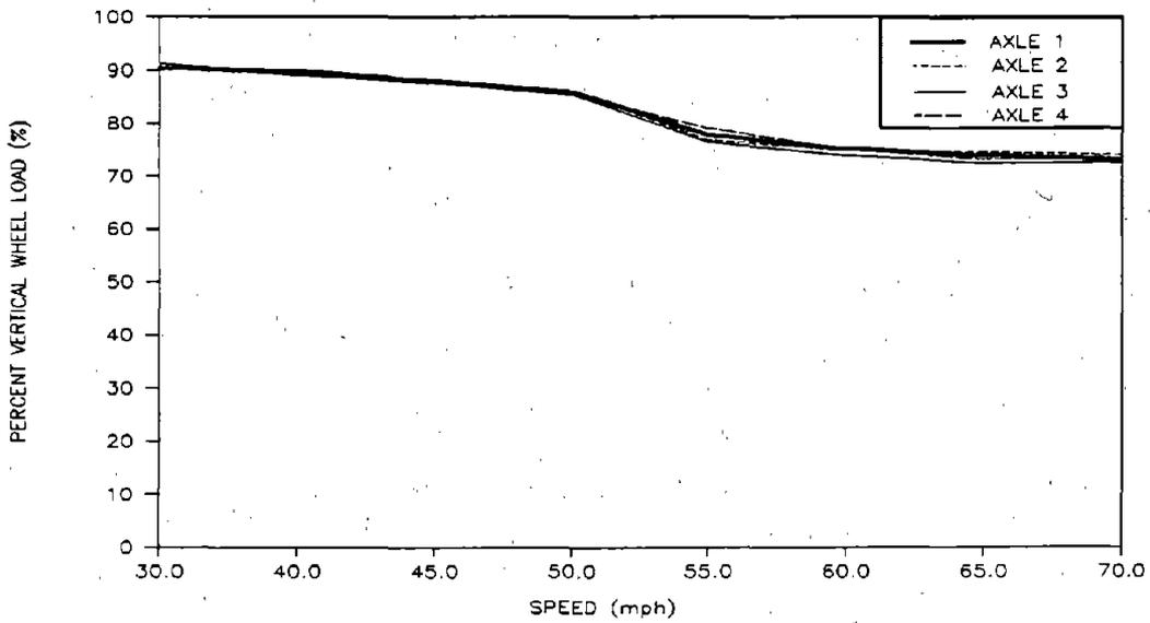
**Figure 38. Pre-test Predictions of Minimum Percent of Vertical Wheel Load for the Loaded Car with Respect to Static Load in the Pitch and Bounce Test Zone**
