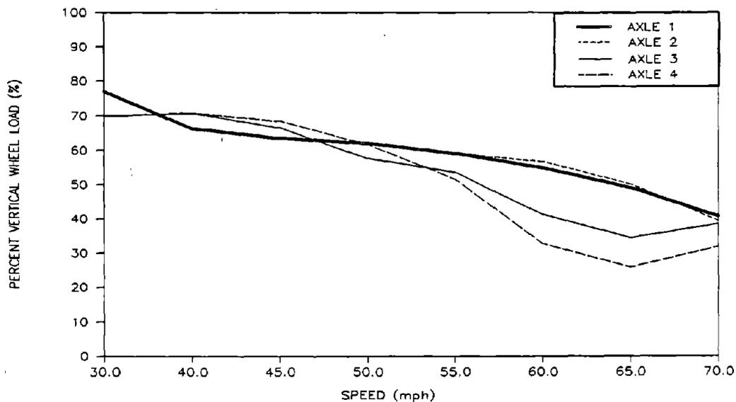
**Figure 42. Pre-test Predictions of Minimum Percent Vertical Wheel Load for the Loaded Car Passing Over the Single Bump**
