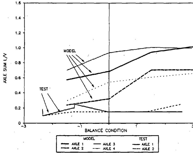
**Figure 108. Maximum Axle Sum L/V Ratios for the Loaded Car in the 4-Degree Curve**
