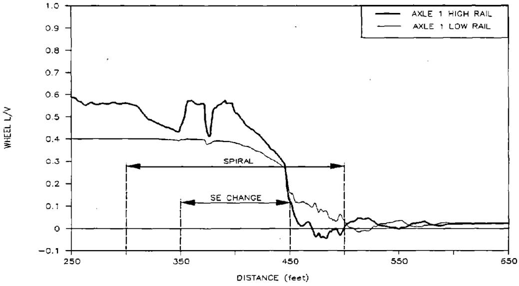
**Figure 51. Pre-test Predictions of Maximum of Wheel L/V for the Empty Car Exiting the Bunched Spiral to Tangent Track at 31.1 mph**
