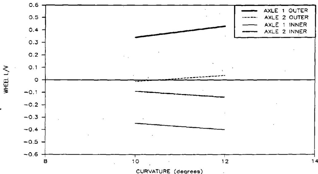
Figure 47. Pre-test Predictions of Maximum Wheel L/V at -3 Inches Cant Deficiency
