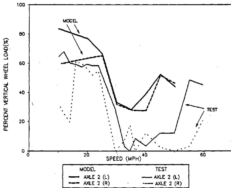
**Figure 91. Minimum Percent Vertical Wheel Loads for Axle 2 of the Empty Car in the Twist and Roll Test Zone**
