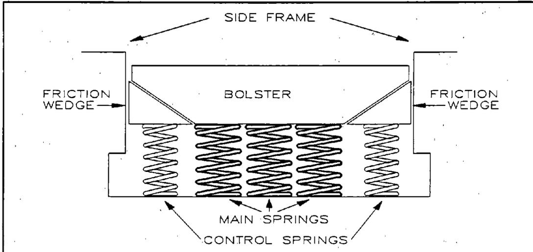
**Figure 9. Diagram of Secondary Vertical Suspension
