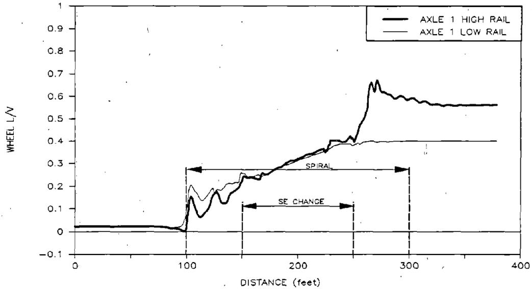
**Figure 49. Pre-test Predictions of Maximum Wheel L/V for the Empty Car Entering the Bunched Spiral from Tangent Track at 31.1 mph**
