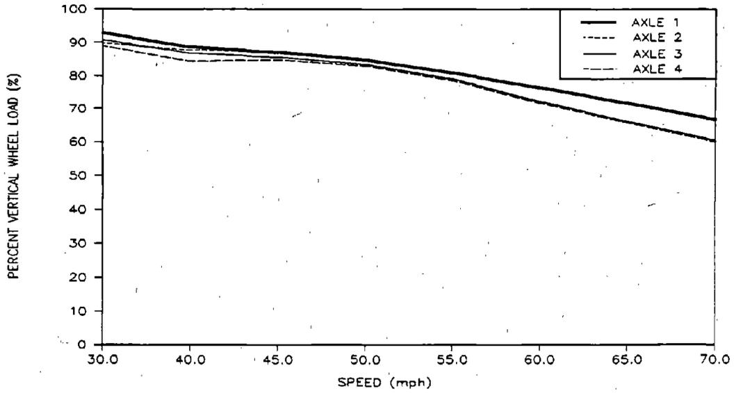
**Figure 37. Pre-test Predictions of Minimum Percent of Vertical Wheel Load for the Empty Car with Respect to Static Load in the Pitch and Bounce Test Zone**
