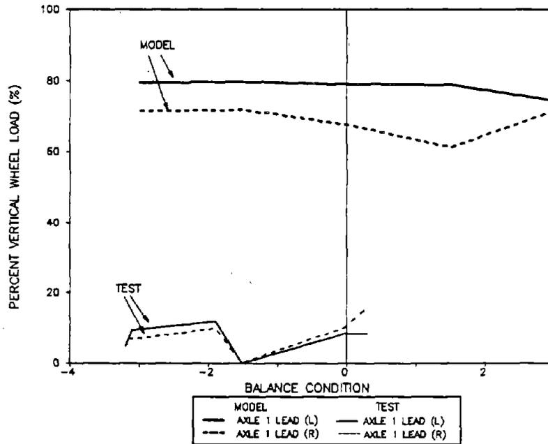
**Figure 115. Minimum Percent Vertical Wheel Load for Axle 1 of the Empty Car in the Bunched Entry Spiral to the 12-Degree Curve**
