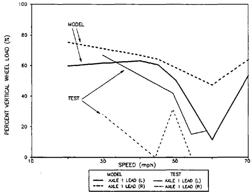
**Figure 75. Minimum Percent Vertical Wheel Load for Axle 1 of the Empty Car in the Pitch and Bounce Test Zone**
