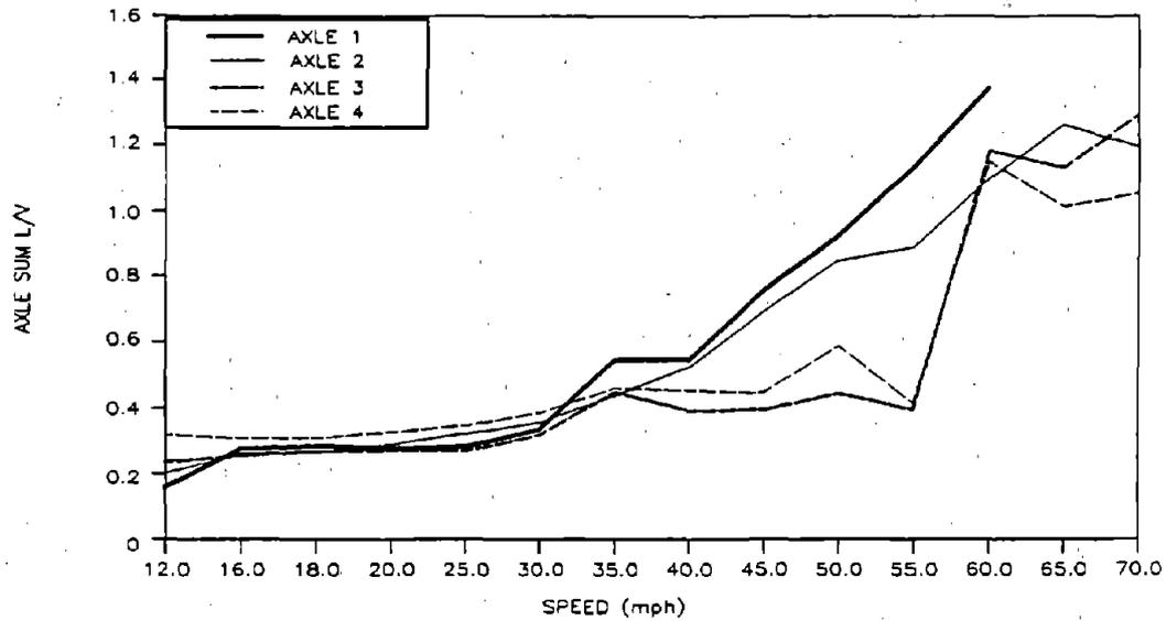
**Figure 33. Pre-test Predictions of Maximum Axle Sum L/V Ratio for the Empty Car in the Twist and Roll Test Zone**
