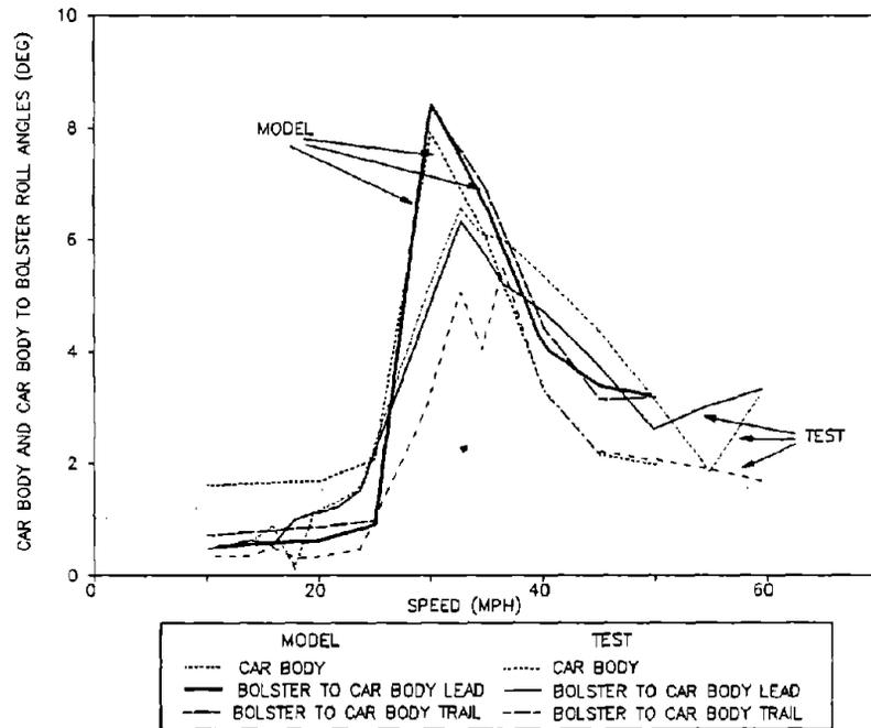
**Figure 94. Maximum Peak to Peak Car Body and Car Body to Bolster Roll Angles of the Empty Car in the Twist and Roll Test Zone**
