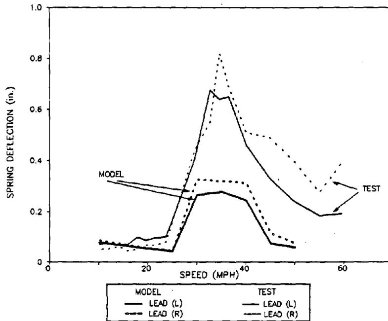
**Figure 92. Maximum Peak to Peak Vertical Spring Deflections for the Lead Truck of the Empty Car in the Twist and Roll Test Zone**
