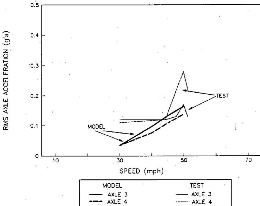
**Figure 72. RMS Lateral Axle Accelerations for the Trail Truck of the Empty Car while Hunting on a 50-Minute Curve**
