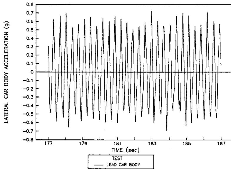
**Figure 68. Measured Lateral Car Body Accelerations for the Empty Car while Hunting at 55 mph on Tangent Track**
