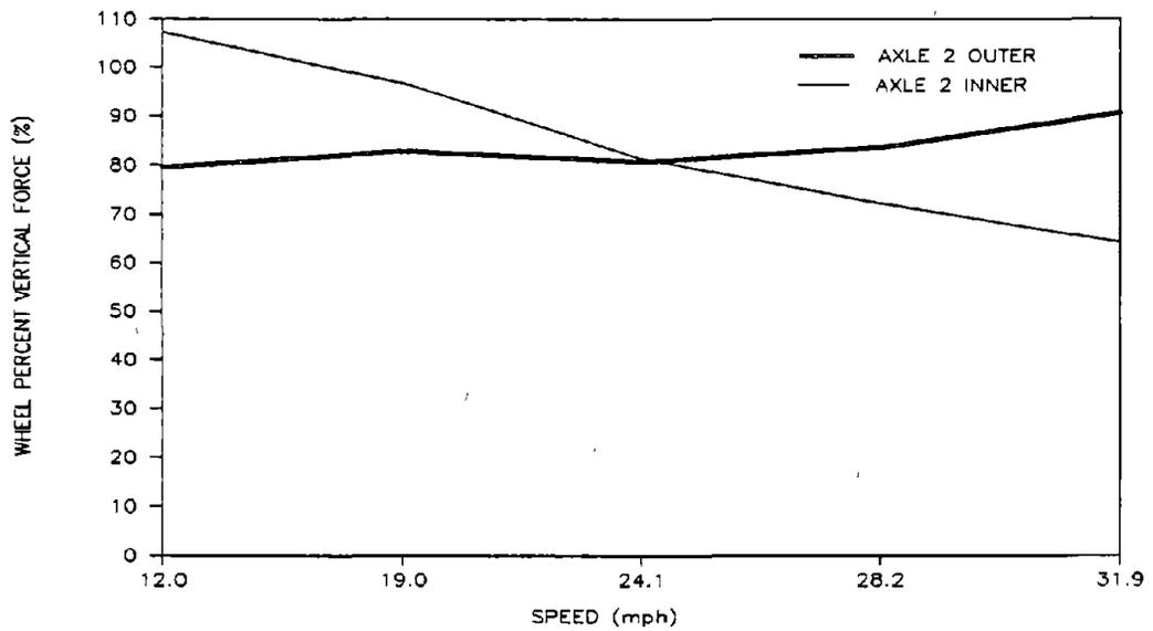
**Figure 59. Pre-test Predictions of Minimum Percent Wheel Vertical Load for the Loaded Car in the Dynamic Curve**
