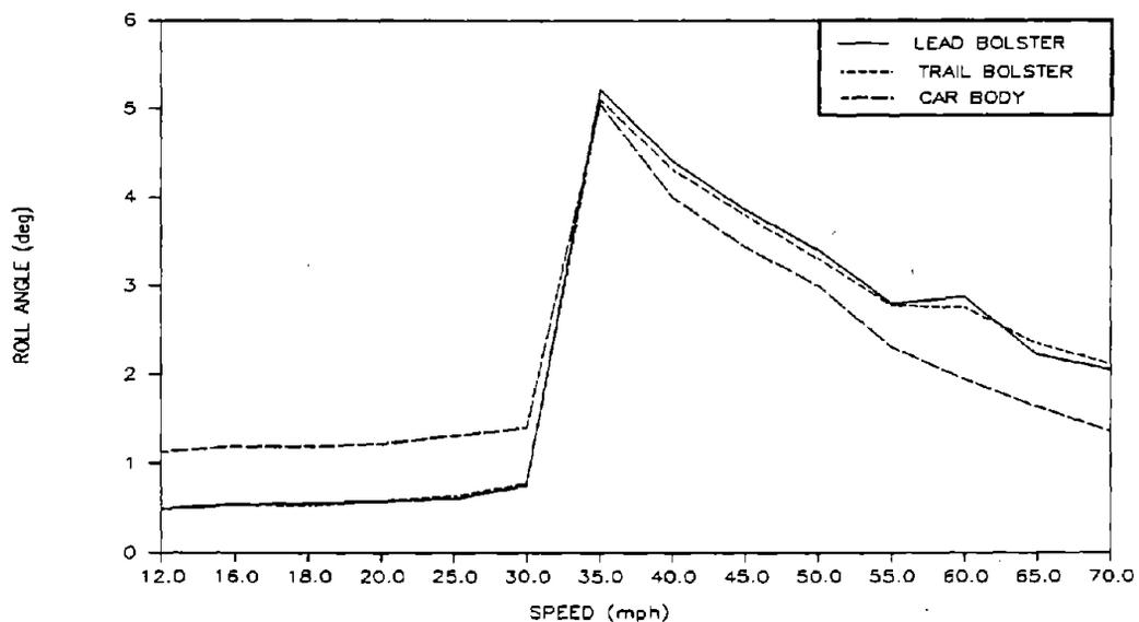
**Figure 32. Pre-test Predictions of Maximum Car Body and Bolster Roll Angles for the Empty Car in the Twist and Roll Test Zone**
