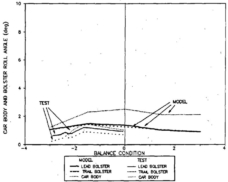
**Figure 135. Maximum Peak to Peak Roll Angles for the Car Body and Bolsters of the Loaded Car in the 10-Degree Dynamic Curve**
