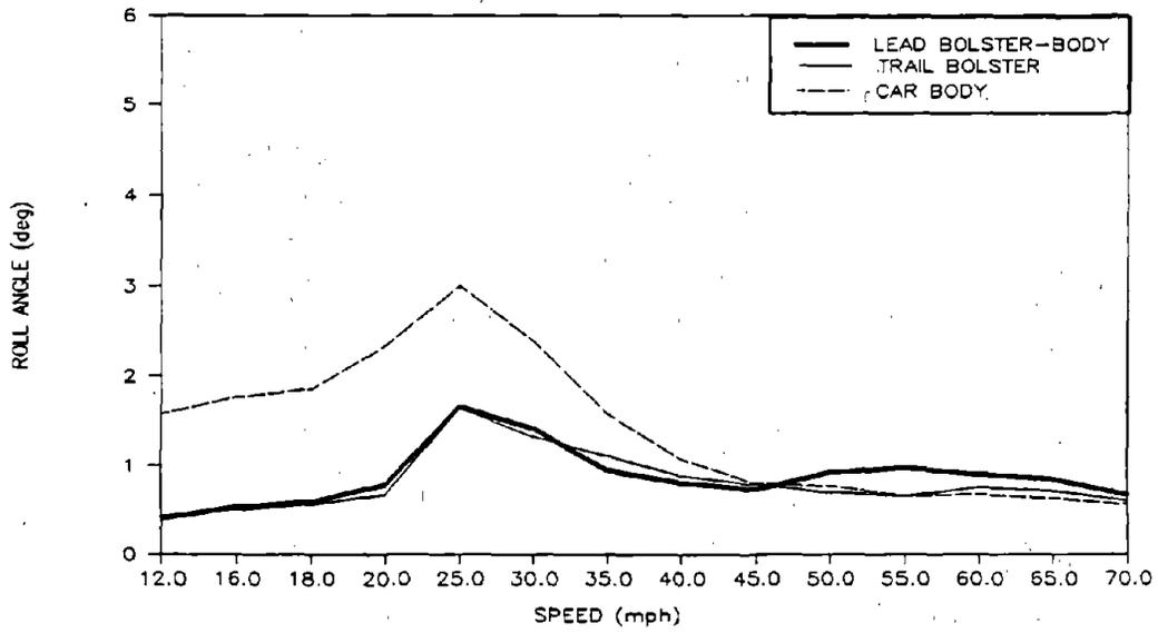
**Figure 35. Pre-test Predictions of Maximum Car Body and Bolster Roll Angles for the Loaded Car in the Twist and Roll Test Zone**
