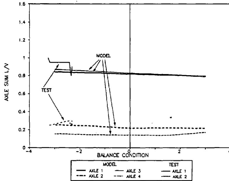
**Figure 110. Maximum Axle Sum L/V Ratios for the Loaded Car in the 10-Degree Curve**
