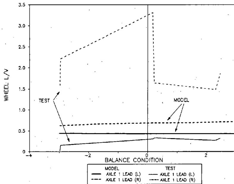
**Figure 117. Maximum Wheel L/V Ratios for Axle 1 of the Empty Car in the Bunched Exit Spiral of the 12-Degree Curve**
