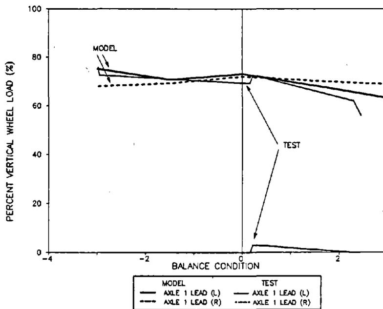
**Figure 119. Minimum Percent Vertical Wheel Load for Axle 1 of the Empty Car in the Bunched Exit Spiral of the 12-Degree Curve**
