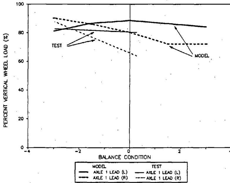
**Figure 123. Minimum Percent Vertical Wheel Load for Axle 1 of the Loaded Car in the Bunched Entry Spiral to the 12-Degree Curve**
