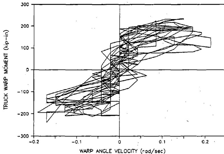
**Figure 63. Measured Average Truck Warp Friction Damping Characteristic for the Loaded Car at 60 mph**
