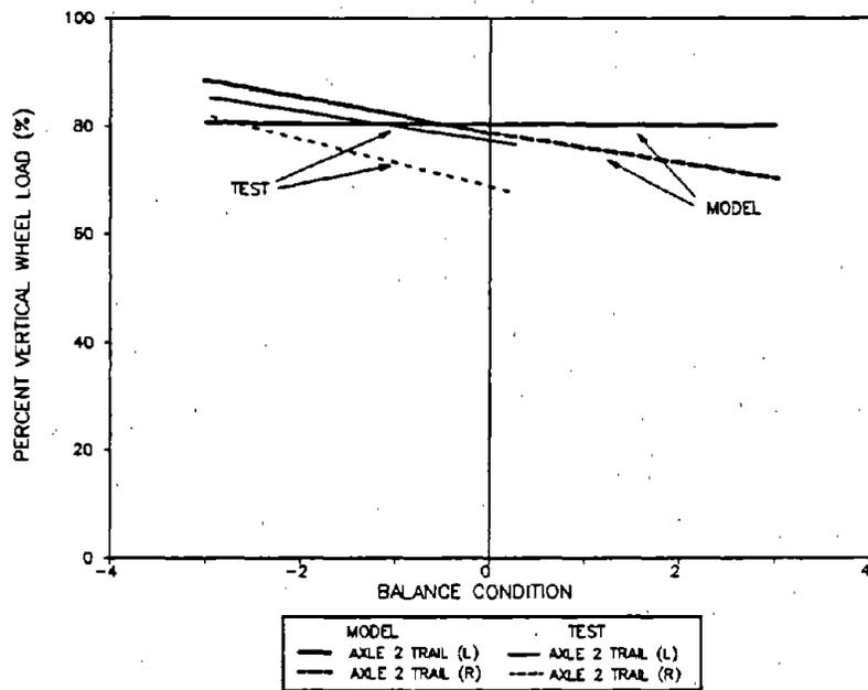
**Figure 124. Minimum Percent Vertical Wheel Load for Axle 2 of the Loaded Car in the Bunched Entry Spiral to the 12-Degree Curve**
