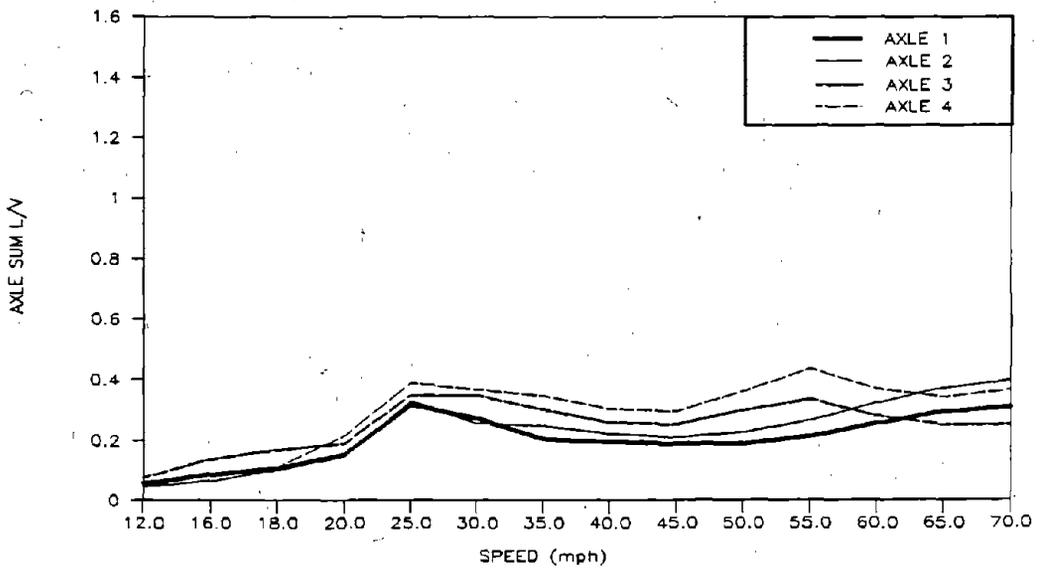
**Figure 36. Pre-test Predictions of Maximum Axle Sum L/V Ratios for the Loaded Car in the Twist and Roll Test Zone**
