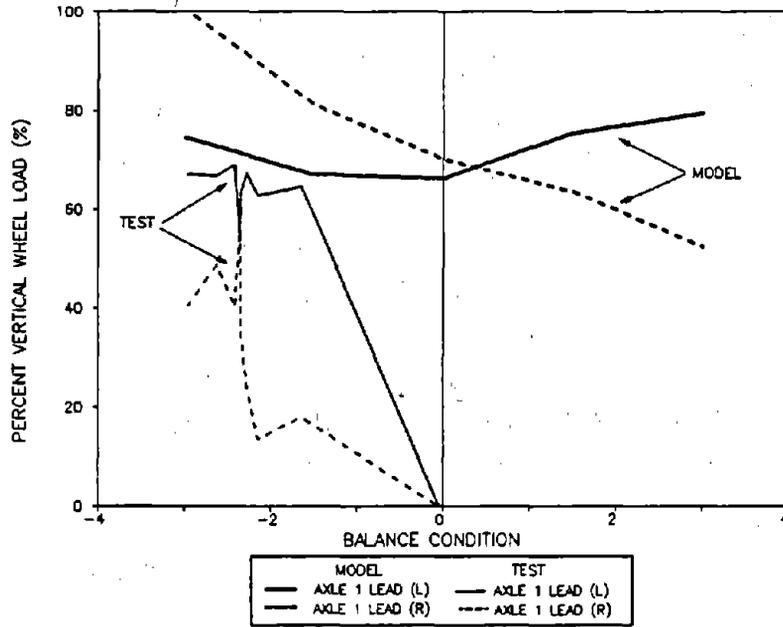
**Figure 131. Minimum Percent Vertical Wheel Load for Axle 1 of the Loaded Car in the 10-Degree Dynamic Curve**
