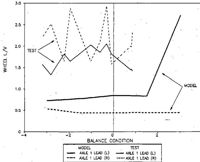
**Figure 129. Maximum Wheel L/V Ratios for Axle 1 of the Empty Car in the 10-Degree Dynamic Curve**
