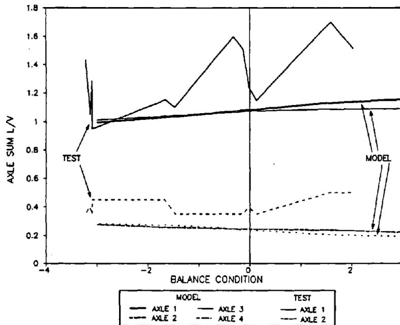
Figure 107. Maximum Axle Sum L/V Ratios for the Empty Car in the 12-Degree Curve
