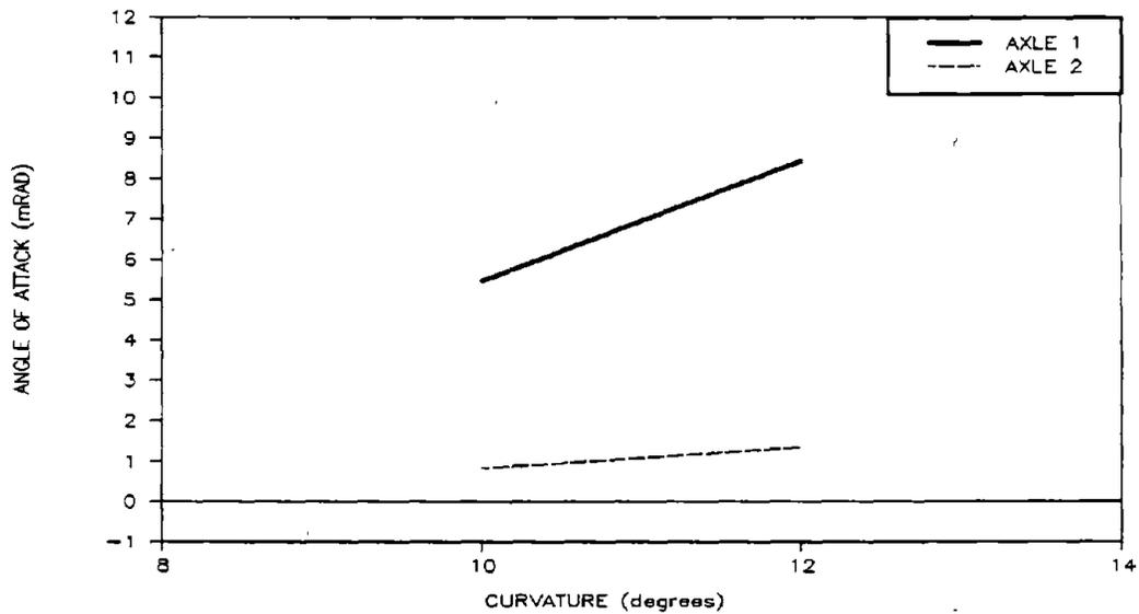
**Figure 48. Pre-test Predictions of Angle of Attack of Axles 1 and 2 for the Loaded Car at -3 Inches Cant Deficiency**
