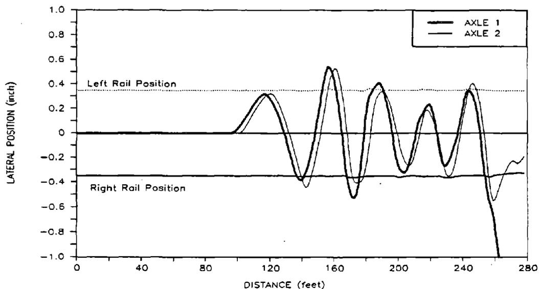
**Figure 34. Pre-test Predictions of Time History of Axle Lateral Motion of the Empty Car at 70 mph in the Twist and Roll Test Zone**
