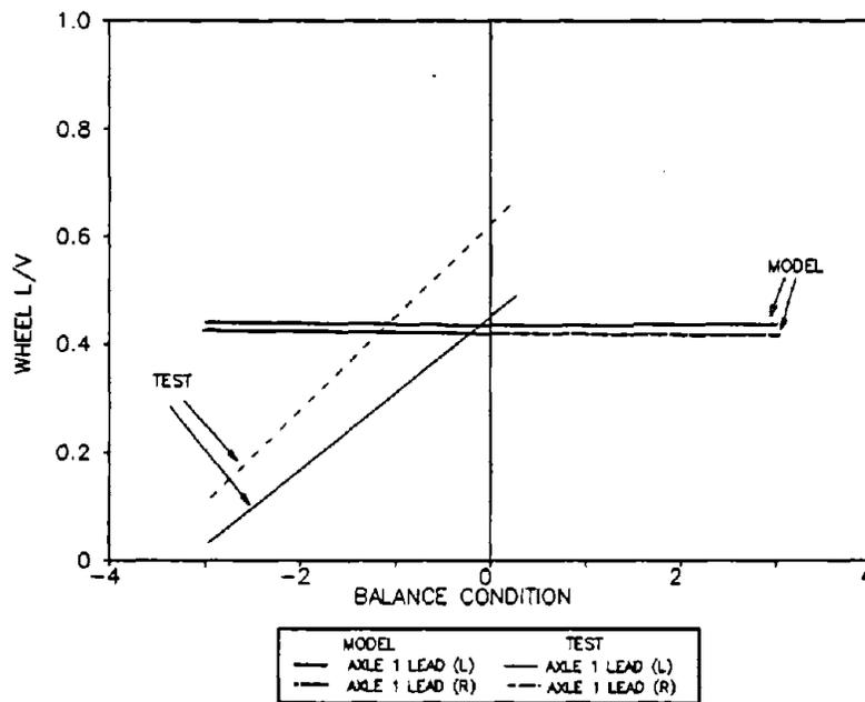
**Figure 121. Maximum Wheel L/V Ratios for Axle 1 of the Loaded Car in the Bunched Entry Spiral to the 12-Degree Curve**
