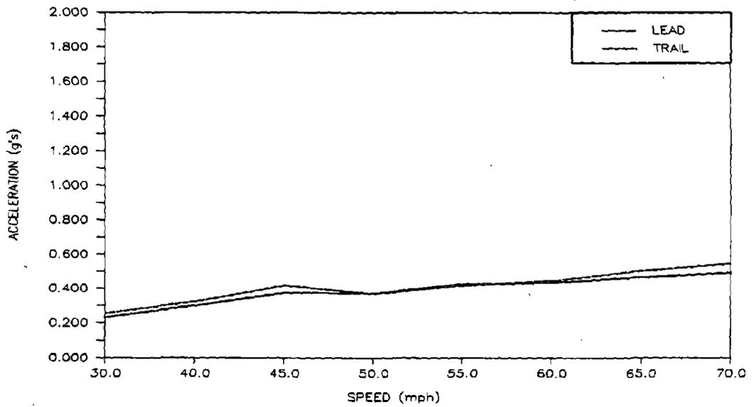
**Figure 29. Pre-test Predictions of Lateral Acceleration of the Empty Car on 50-Minute-Curved Track**
