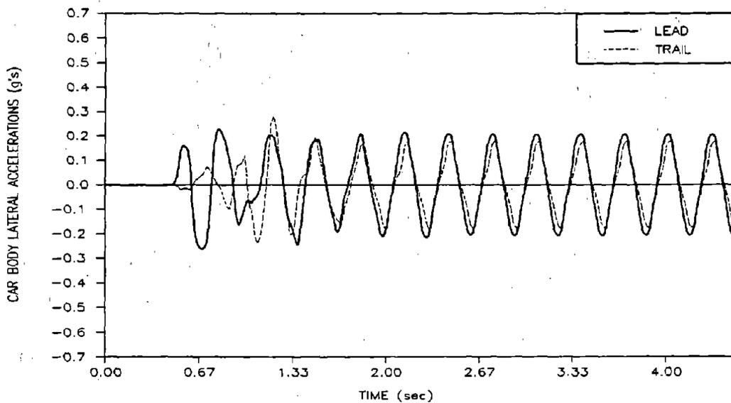
Figure 31. Pre-test Predictions of Lateral Car Body Acceleration for the Loaded Car at 70 mph on Tangent Track
