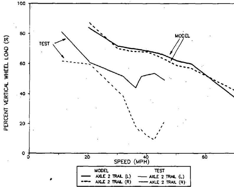
**Figure 87. Minimum Percent Vertical Wheel Loads for Axle 2 of the Loaded Car Passing over the Single Bump**
