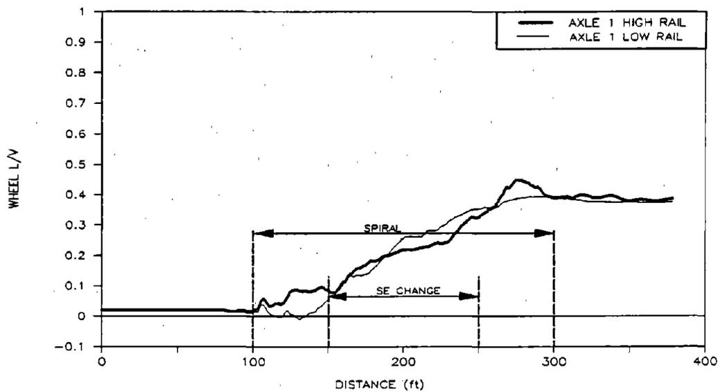
**Figure 53. Pre-test Predictions of Maximum Wheel L/V for the Loaded Car Entering the Bunched Spiral from Tangent Track at 31.1 mph**
