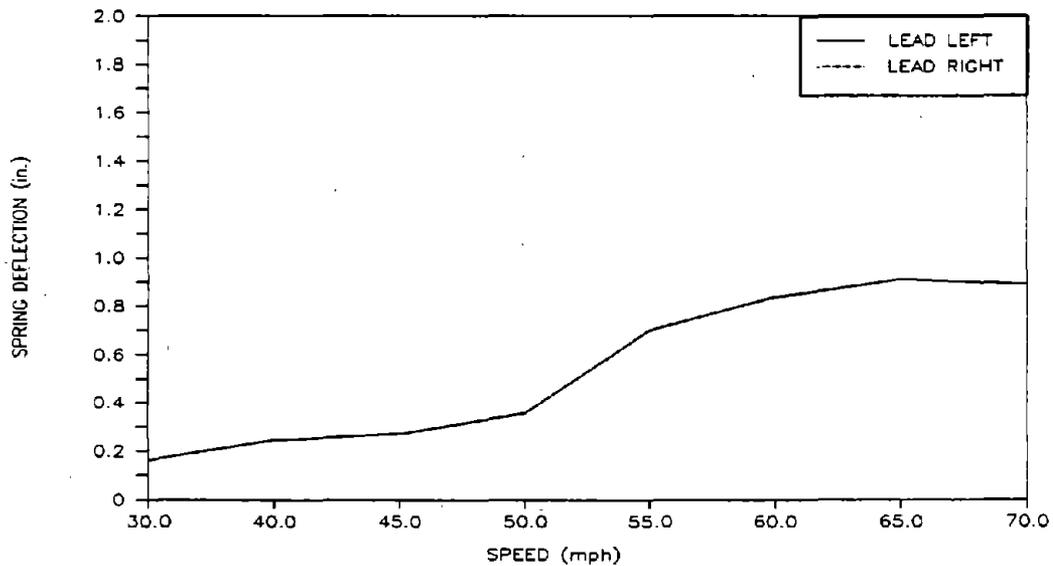
**Figure 39. Pre-test Predictions of Maximum Vertical Spring Deflections for the Loaded Car in the Pitch and Bounce Test Zone**
