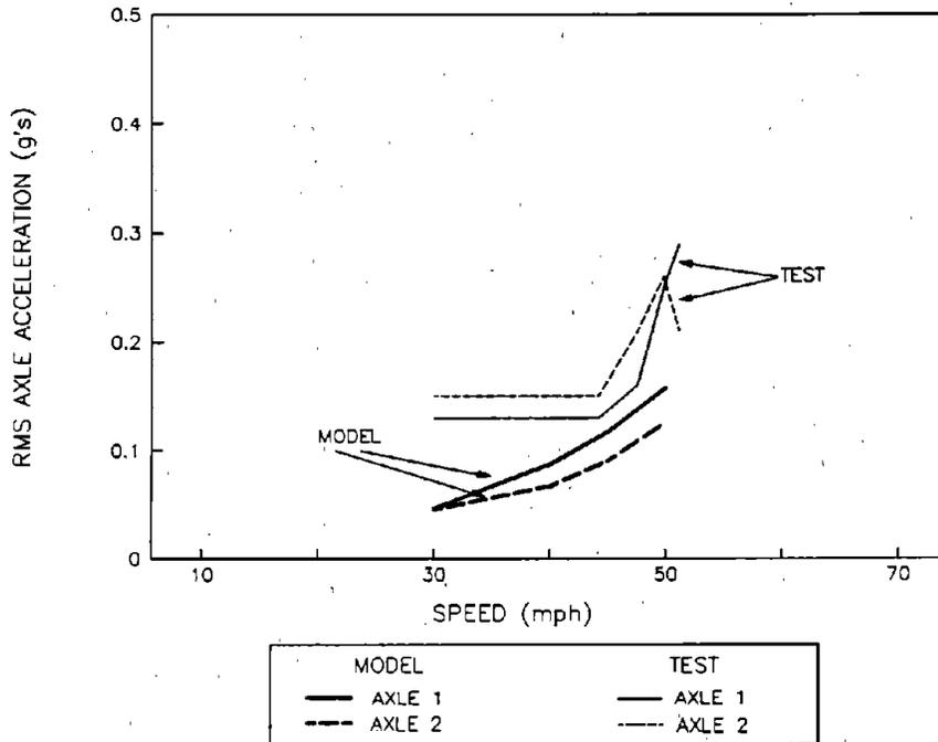
**Figure 71. RMS Lateral Axle Accelerations for the Lead Truck of the Empty Car while Hunting on a 50-Minute Curve**
