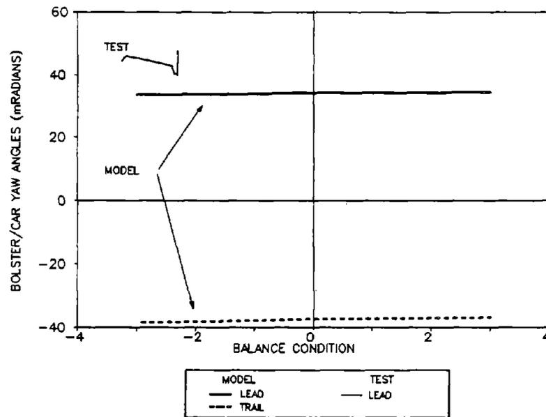
Figure 112. Average Bolster to Car Body Yaw Angles for the Loaded Car in the 10-Degree Curve
