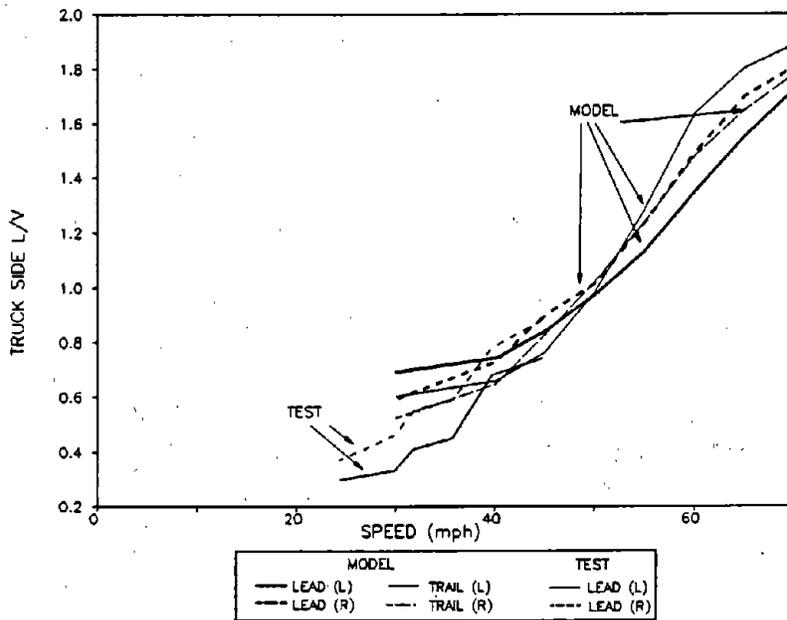
**Figure 103. Maximum Truck Side L/V Ratios for the Loaded Car in the Yaw and Sway Test Zone**
