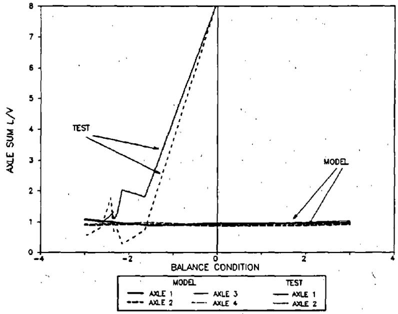
**Figure 134. Maximum Axle Sum L/V Ratios for the Loaded Car in the 10-Degree Dynamic Curve**
