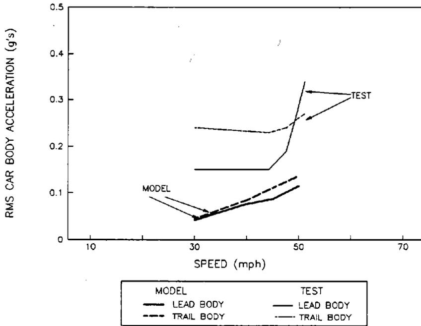
**Figure 73. RMS Lateral Car Body Accelerations for the Empty Car while Hunting on a 50-Minute Curve**
