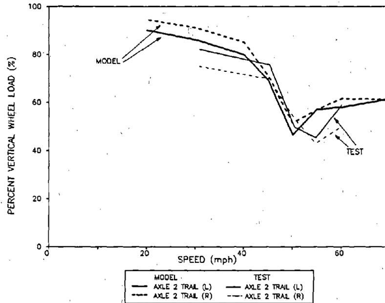
**Figure 79. Minimum Percent Vertical Wheel Loads for Axle 2 of the Loaded Car in the Pitch and Bounce Test Zone**
