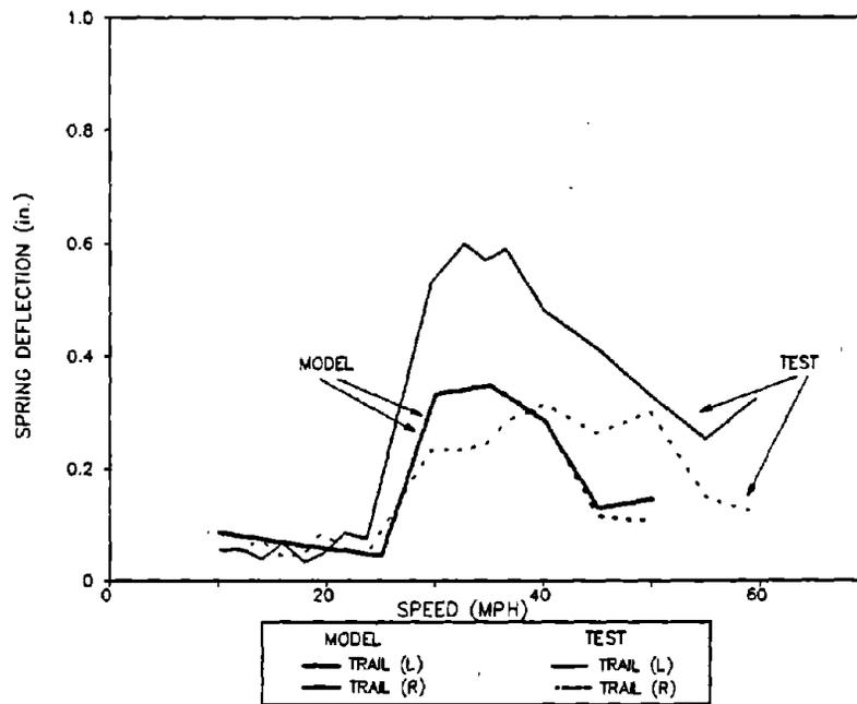
**Figure 93. Maximum Peak to Peak Vertical Spring Deflections for the Trail Truck of the Empty Car in the Twist and Roll Test Zone**
