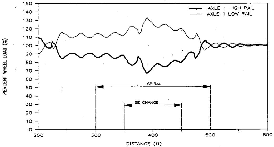
**Figure 56. Pre-test Predictions of Minimum Percent Wheel Vertical Load for the Loaded Car Exiting the Bunched Spiral to Tangent Track at 15.5 mph**
