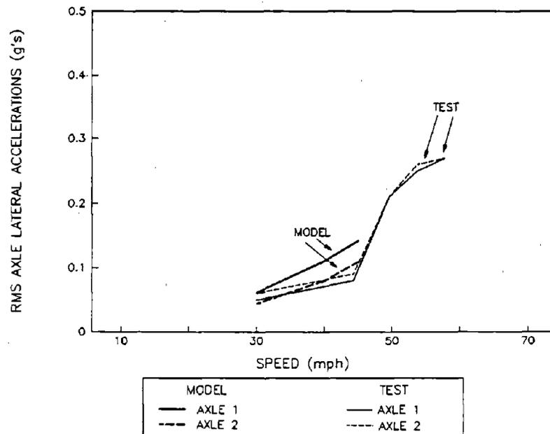
Figure 65. RMS Lateral Axle Accelerations for the Lead Truck of the Empty Car while Hunting on Tangent Track
