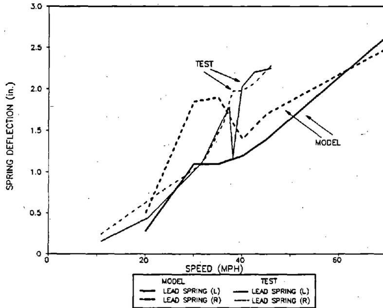
**Figure 88. Maximum Peak to Peak Vertical Spring Deflections for the Lead Truck of the Loaded Car Passing over the Single Bump**
