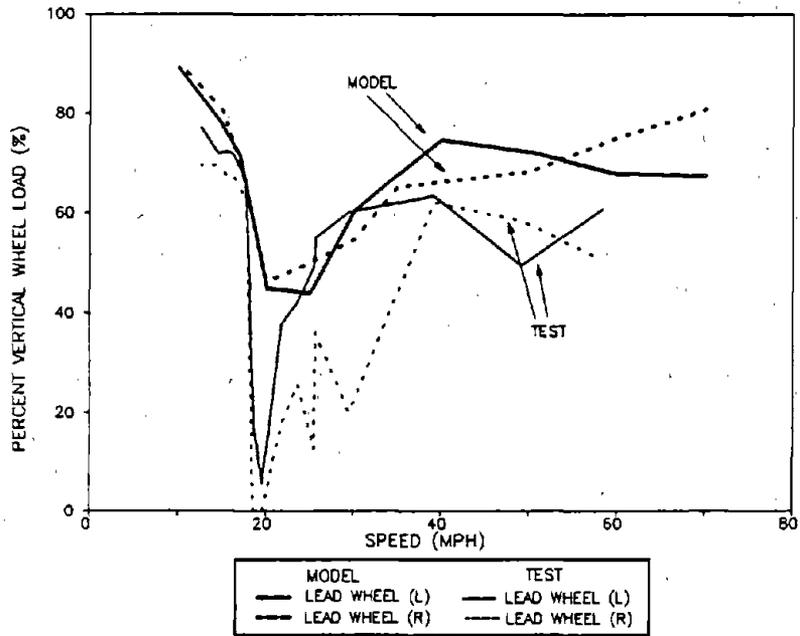
**Figure 95. Minimum Percent Vertical Wheel Loads for Axle 1 of the Loaded Car in the Twist and Roll Test Zone**
