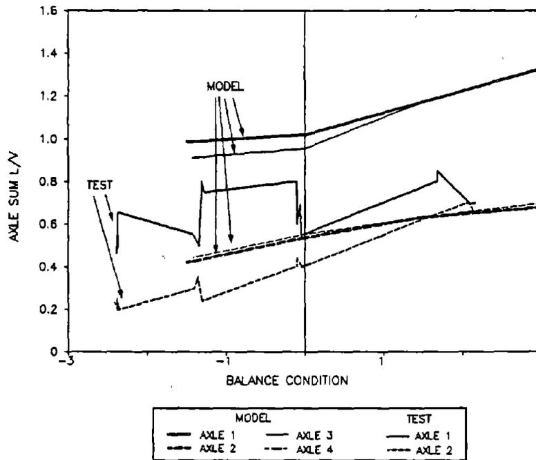
**Figure 105. Maximum Axle Sum L/V Ratios for the Empty Car in the 4-Degree Curve**
