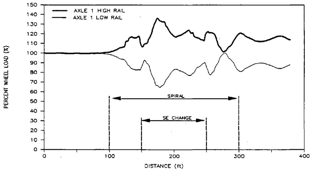
**Figure 54. Pre-test Predictions of Minimum Percent Wheel Vertical Load for the Loaded Car Entering the Bunched Spiral from Tangent Track at 31.1 mph**
