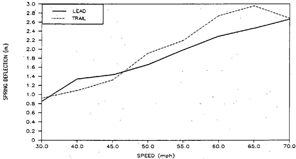
**Figure 43. Pre-test Predictions of Maximum Vertical Spring Deflection for the Loaded Car Passing Over the Single Bump**
