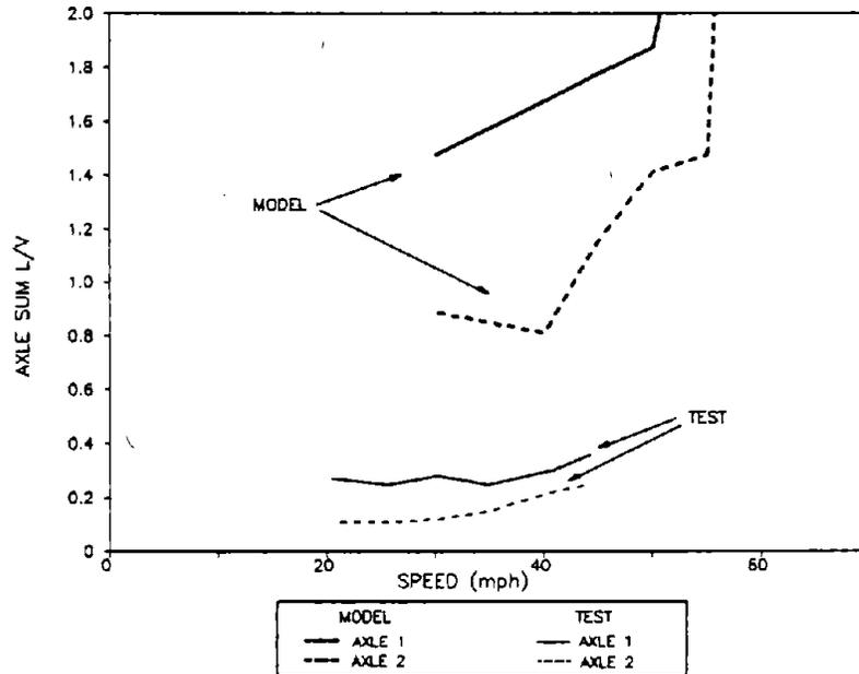
Figure 100. Maximum Axle Sum L/V Ratios for the Empty Car in the Yaw and Sway Test Zone
