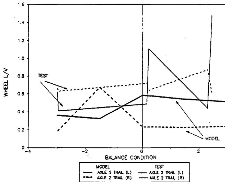
**Figure 118. Maximum Wheel L/V Ratios for Axle 2 of the Empty Car in the Bunched Exit Spiral of the 12-Degree Curve**
