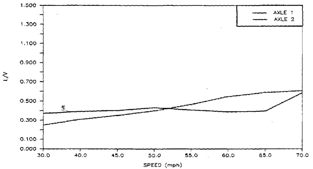
**Figure 30. Pre-test Predictions of Maximum Axle Sum L/V Ratios Versus Speed for the Empty Car on 50-Minute-Curved Track**
