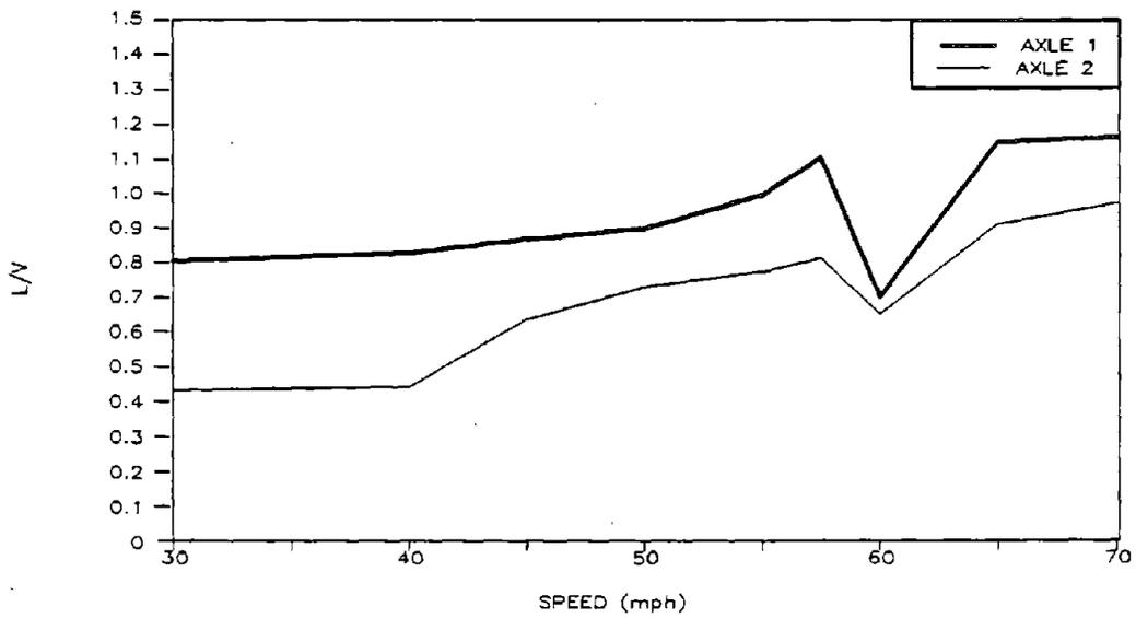
**Figure 27. Pre-test Predictions of Maximum Axle Sum L/V Ratio Versus Speed of Empty Car on Tangent Track**
