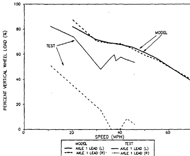
Figure 86. Minimum Percent Vertical Wheel Loads for Axle 1 of the Loaded Car Passing over the Single Bump
