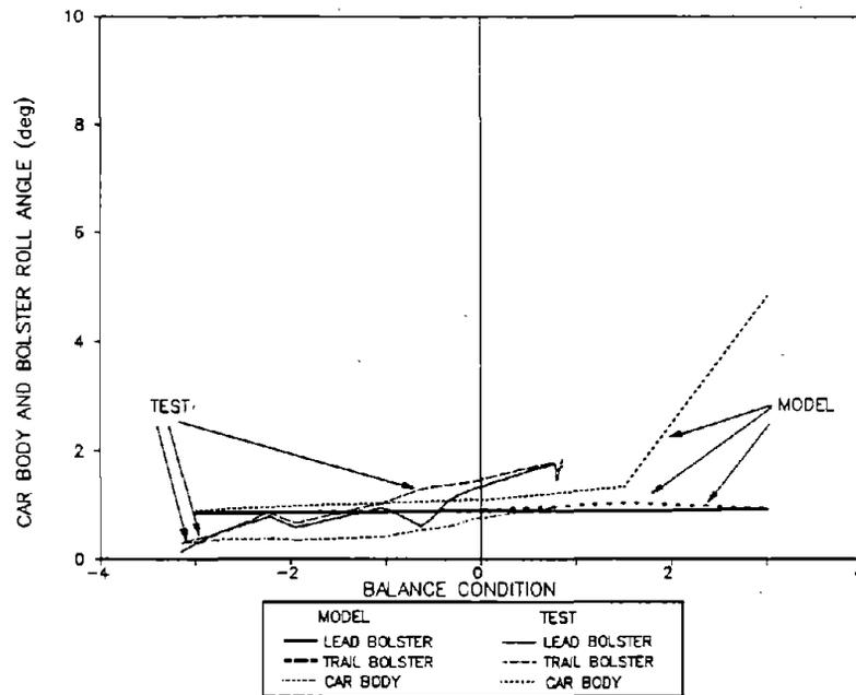
**Figure 130. Maximum Peak to Peak Car Body and Bolster Roll Angles of the Empty Car in the 10-Degree Dynamic Curve**
