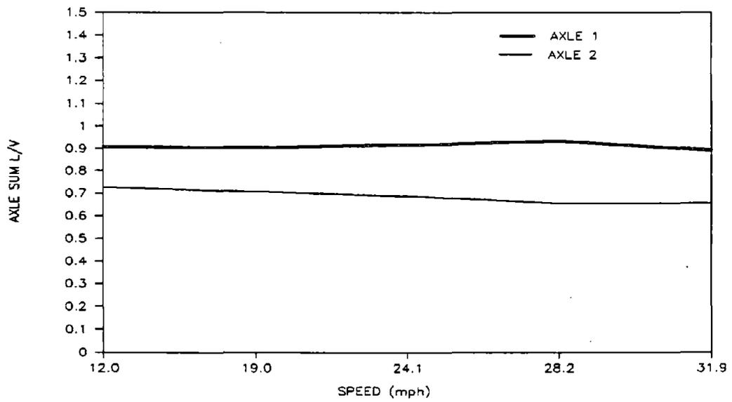
**Figure 58. Pre-test Predictions of Maximum Axle Sum L/V Ratios for the Loaded Car Negotiating the Dynamic Curve**
