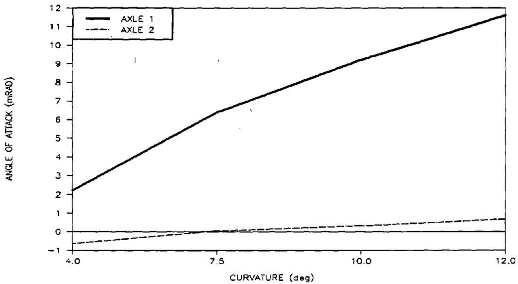
**Figure 46. Pre-test Predictions of Angle of Attack of Axles 1 and 2 at +3 Inches Cant Deficiency**
