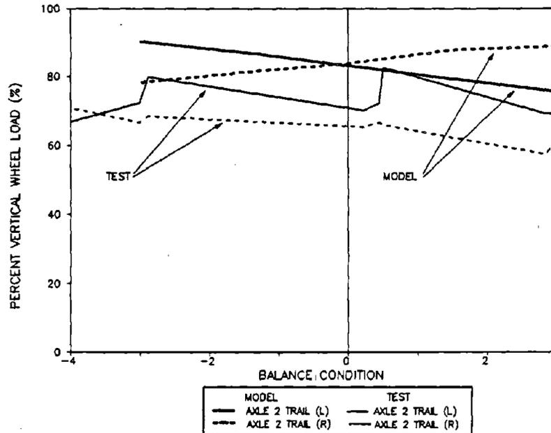
Figure 128. Minimum Percent Vertical Wheel Load for Axle 2 of the Loaded Car in the Bunched Exit Spiral of the 12-Degree Curve
