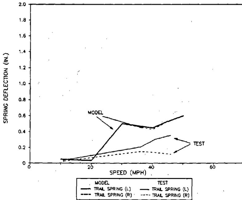
**Figure 85. Maximum Peak to Peak Vertical Spring Deflections for the Trail Truck of the Empty Car Passing over the Single Bump**
