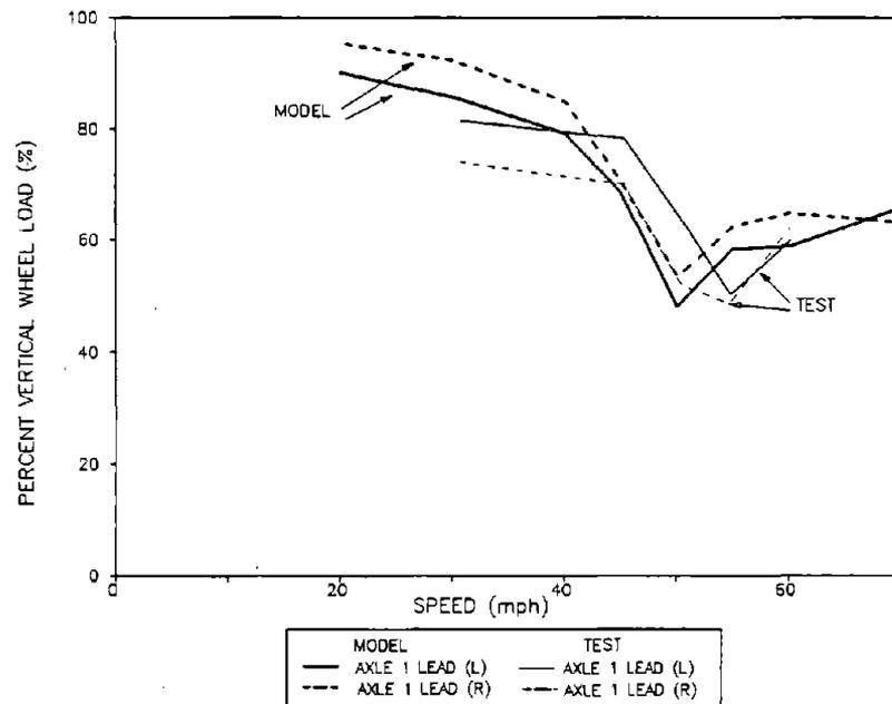
**Figure 78. Minimum Percent Vertical Wheel Loads for Axle 1 of the Loaded Car in the Pitch and Bounce Test Zone**
