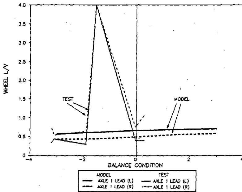
**Figure 113. Maximum Wheel L/V Ratios for Axle 1 of the Empty Car in the Bunched Entry Spiral to the 12-Degree Curve**
