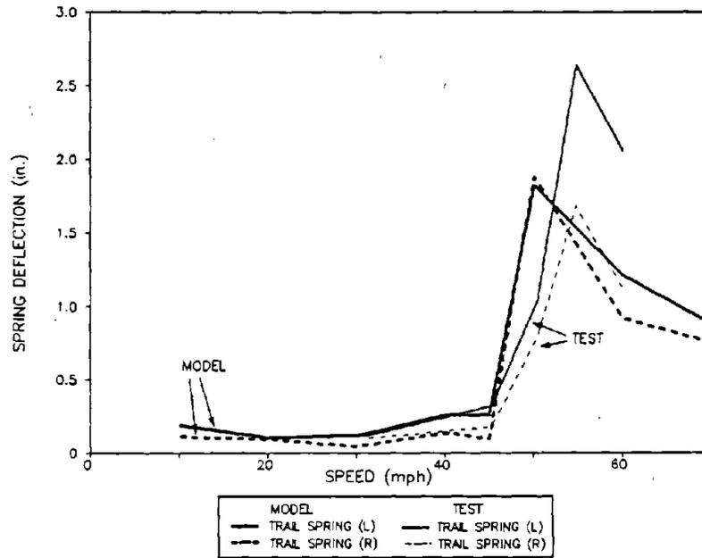
**Figure 81. Maximum Peak to Peak Vertical Spring Deflections for the Trail Truck of the Loaded Car in the Pitch and Bounce Test Zone**
