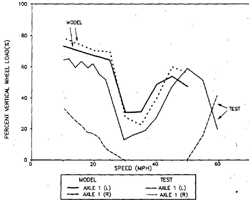
**Figure 90. Minimum Percent Vertical Wheel Loads for Axle 1 of the Empty Car in the Twist and Roll Test Zone**
