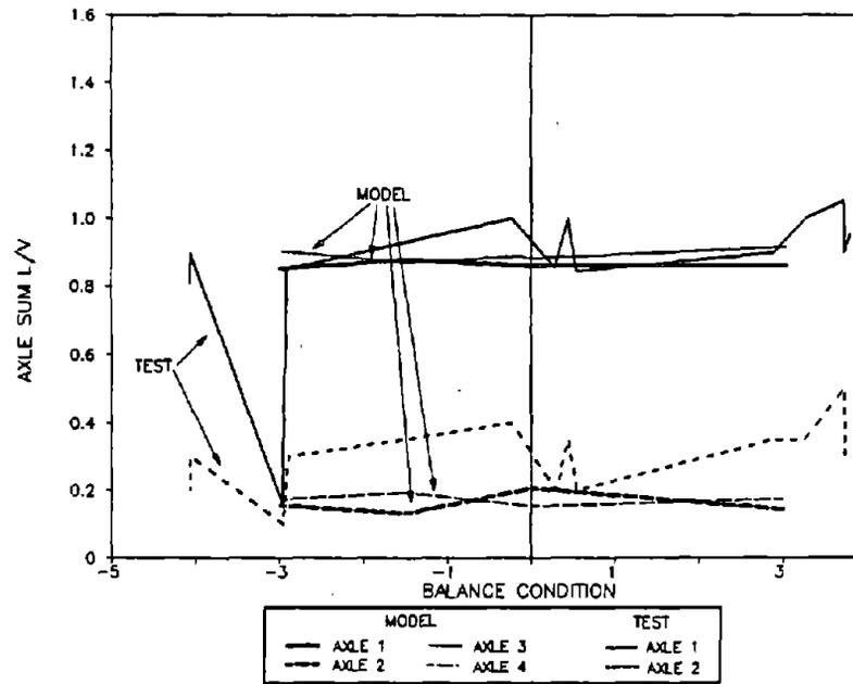
**Figure 111. Maximum Axle Sum L/V Ratios for the Loaded Car in the 12-Degree Curve**
