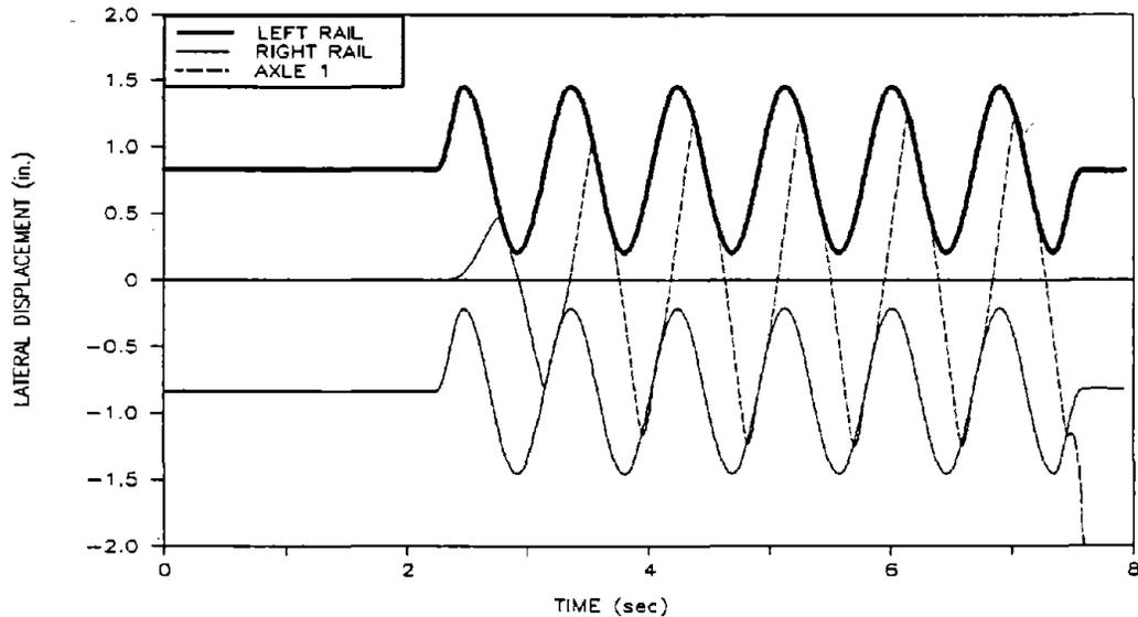
**Figure 44. Pre-test Predictions of Lateral Position of Axle 1 for the Empty Car in Relation to the Lateral Rail Position in the Yaw Sway Test Zone at 30 mph**
