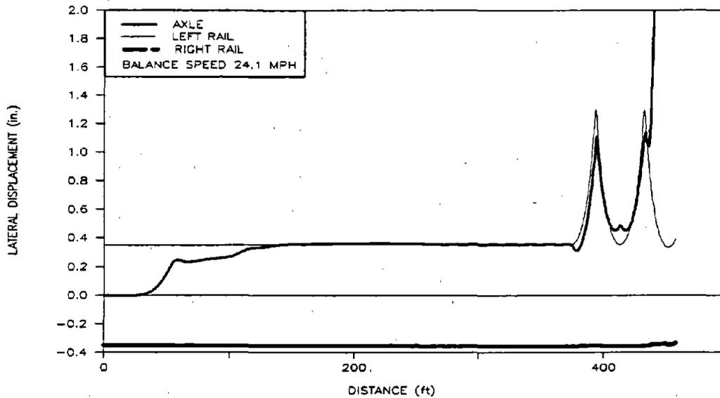
**Figure 57. Pre-test Predictions of Lateral Position of Axle 1, Left and Right Rails as the Empty Car Negotiates the Dynamic Curve at Balance Speed**
