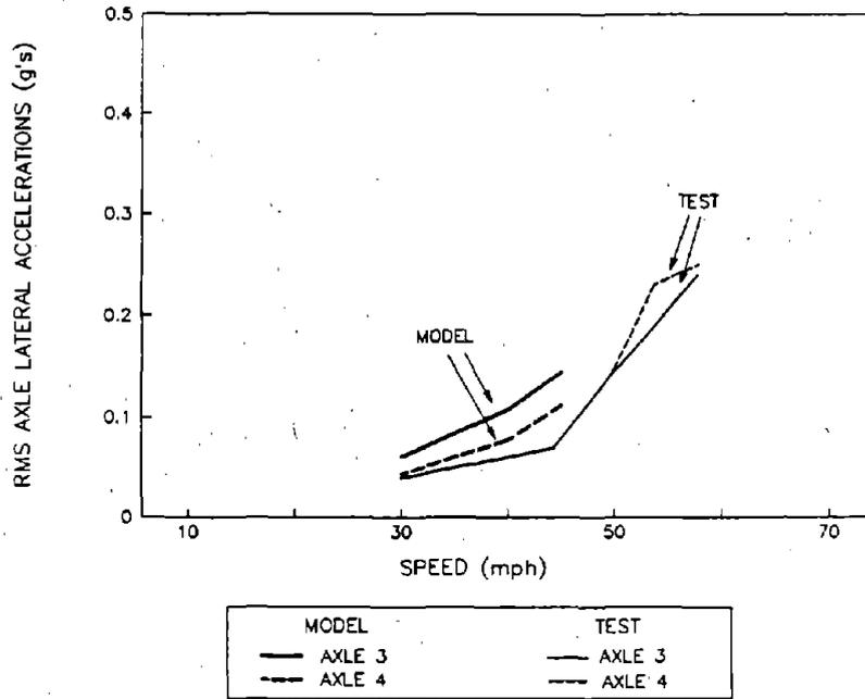
**Figure 66. RMS Lateral Axle Accelerations for the Trail Truck of the Empty Car while Hunting on Tangent Track**
