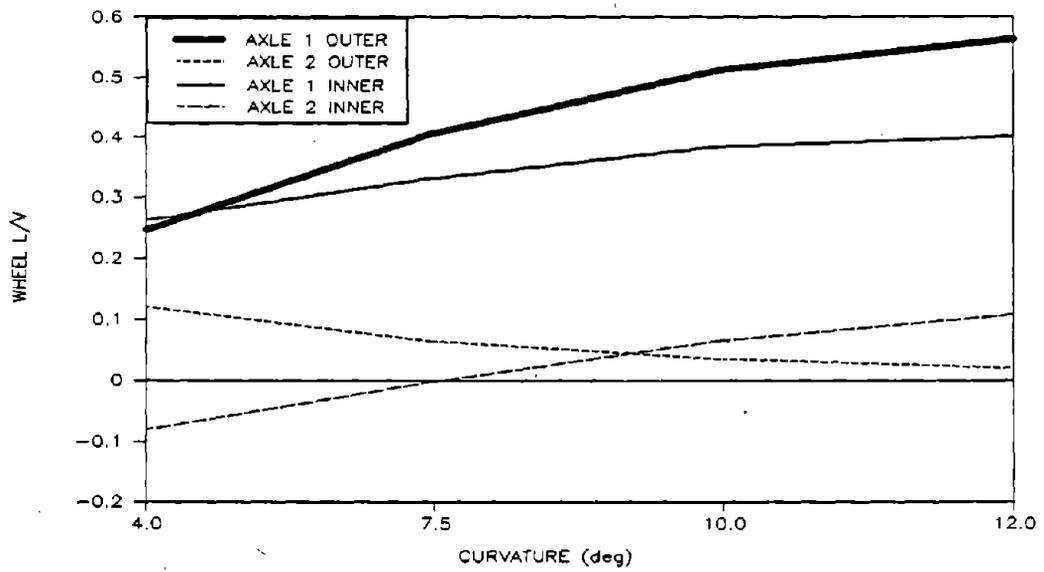
**Figure 45. Pre-test Predictions of Maximum Individual Wheel L/V Ratio at +3 Inches Cant Deficiency**
