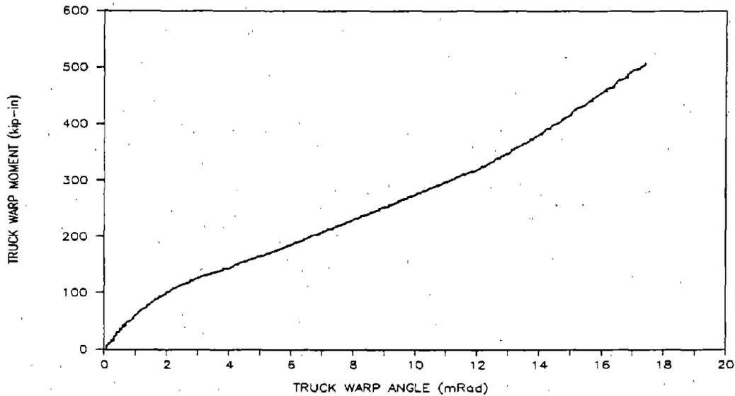
**Figure 24. Truck Warp Moment Versus Warp Angle Characteristic**
