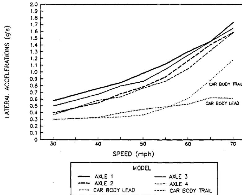
**Figure 70. Predicted RMS Lateral Accelerations for the Loaded Car while Hunting on Tangent Track**
