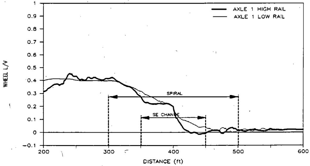
**Figure 55. Pre-test Predictions of Maximum Wheel L/V for the Loaded Car Exiting the Bunched Spiral to Tangent Track at 15.5 mph**
