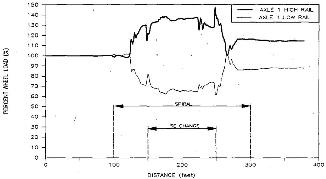
**Figure 50. Pre-test Predictions of Minimum Percent Vertical Load of Individual Wheels for the Empty Car Entering the Bunched Spiral from Tangent Track at 31.1 mph**
