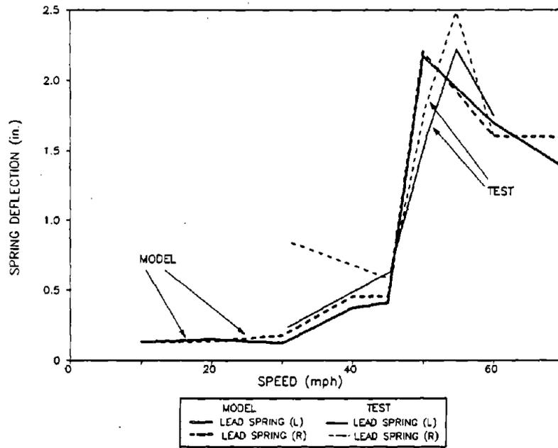
**Figure 80. Maximum Peak to Peak Vertical Spring Deflections for the Lead Truck of the Loaded Car in the Pitch and Bounce Test Zone**
