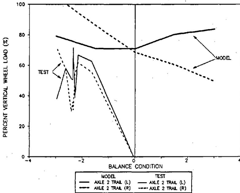
**Figure 132. Minimum Percent Vertical Wheel Load for Axle 2 of the Loaded Car in the 10-Degree Dynamic Curve**
