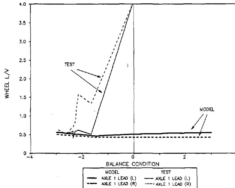
**Figure 133. Maximum Wheel L/V Ratios for Axle 1 of the Loaded Car in the 10-Degree Dynamic Curve**
