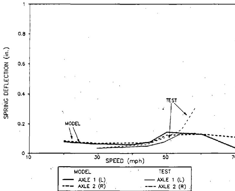
**Figure 77. Maximum Peak to Peak Vertical Spring Deflections for the Lead Truck of the Empty Car in the Pitch and Bounce Test Zone**
