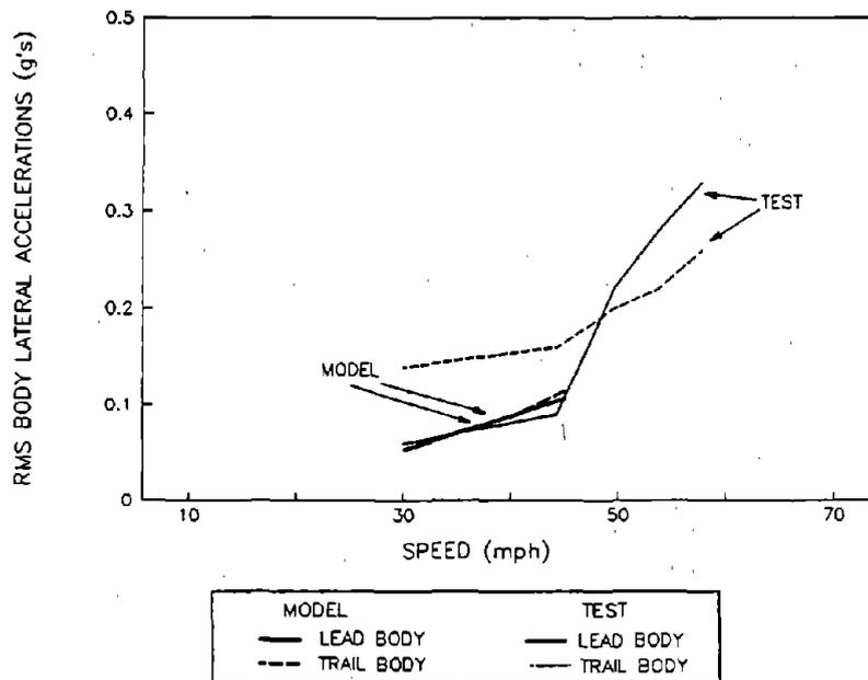
**Figure 67. RMS Lateral Car Body Accelerations for the Empty Car while Hunting on Tangent Track**
