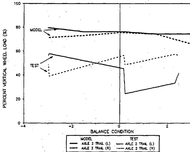
**Figure 120. Minimum Percent Vertical Wheel Load for Axle 2 of the Empty Car in the Bunched Exit Spiral of the 12-Degree Curve**
