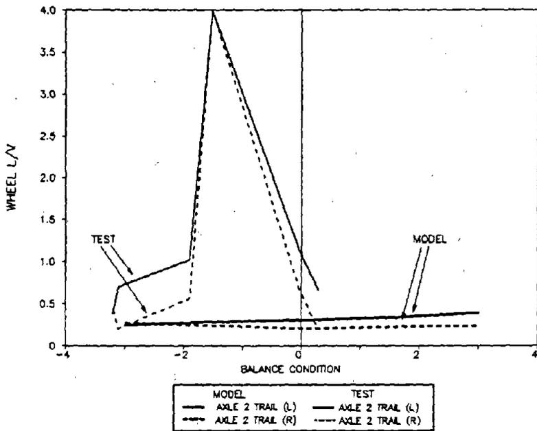
**Figure 114. Maximum Wheel L/V Ratios for Axle 2 of the Empty Car in the Bunched Entry Spiral to the 12-Degree Curve**
