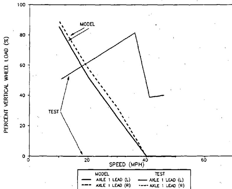
Figure 82. Minimum Percent Vertical Wheel Loads for Axle 1 of the Empty Car Passing over the Single Bump
