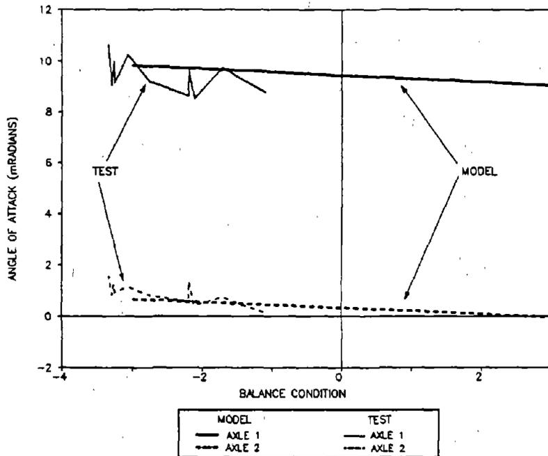
**Figure 106. Axle Angles of Attack for the Empty Car in the 10-Degree Curve**
