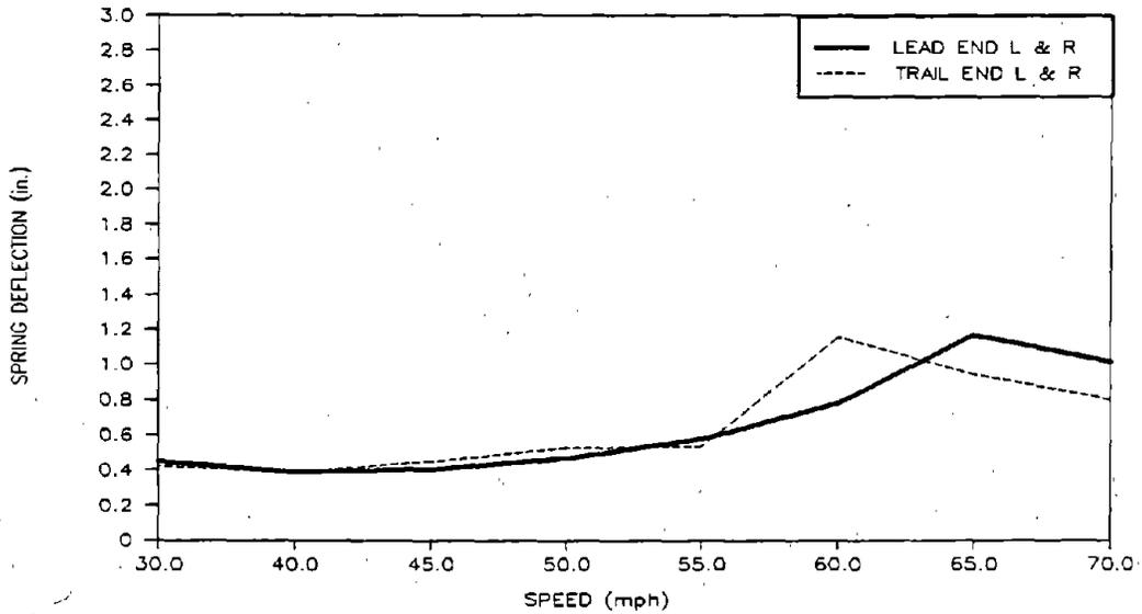
**Figure 41. Pre-test Predictions of Maximum Vertical Spring Deflection for the Empty Car Passing Over the Single Bump**
