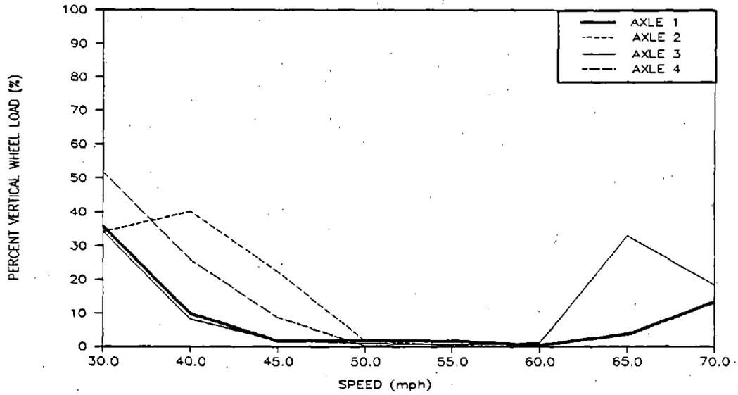
**Figure 40. Pre-test Predictions of Minimum Percent Vertical Wheel Load for the Empty Car Passing Over the Single Bump**
