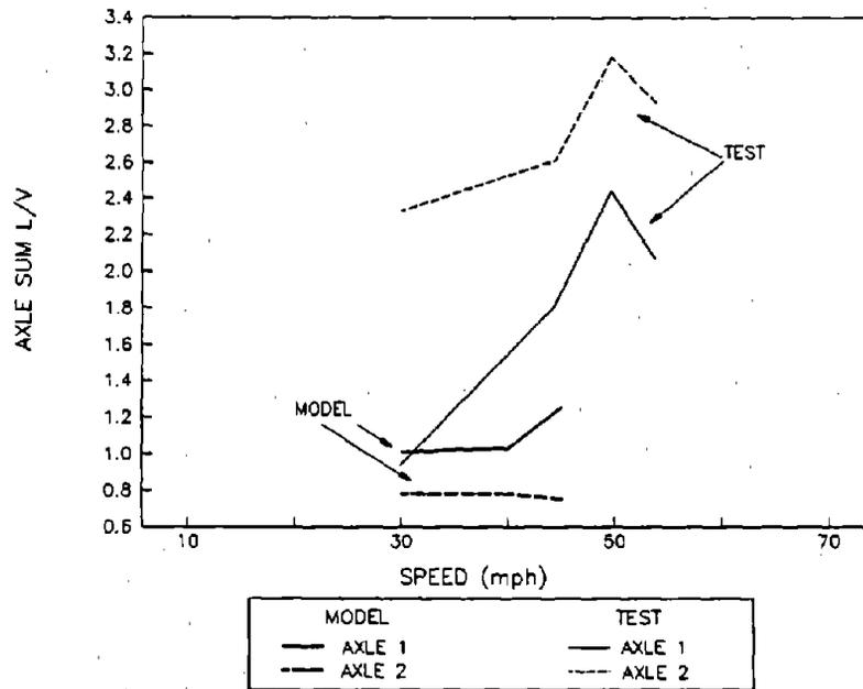
**Figure 69. Axle Sum L/V Ratios for the Empty Car while Hunting on Tangent Track**
