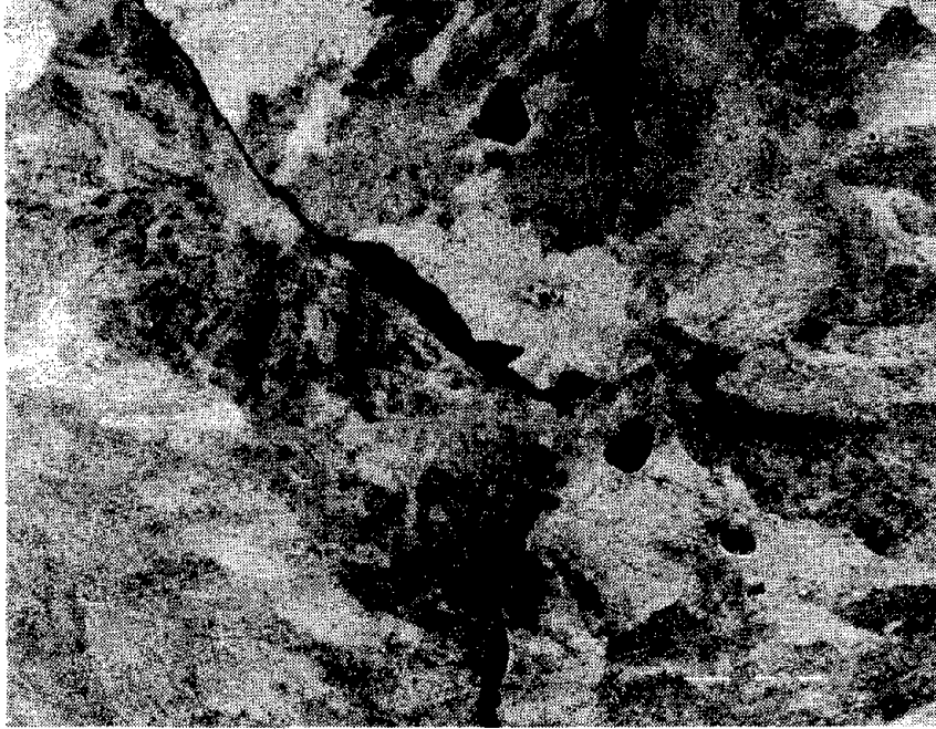
FIGURE 28: PROEUTECTOID FERRITE IN THE WELD METAL OF WELD 6. 450X.
