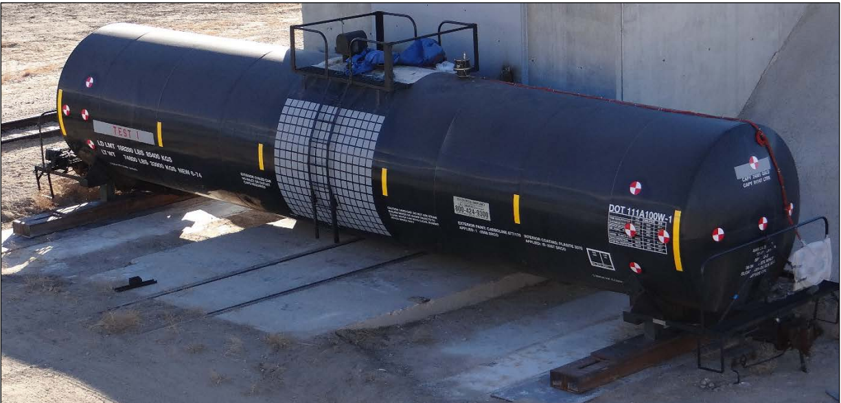
Figure A-2. DOT-111 Tank Car
