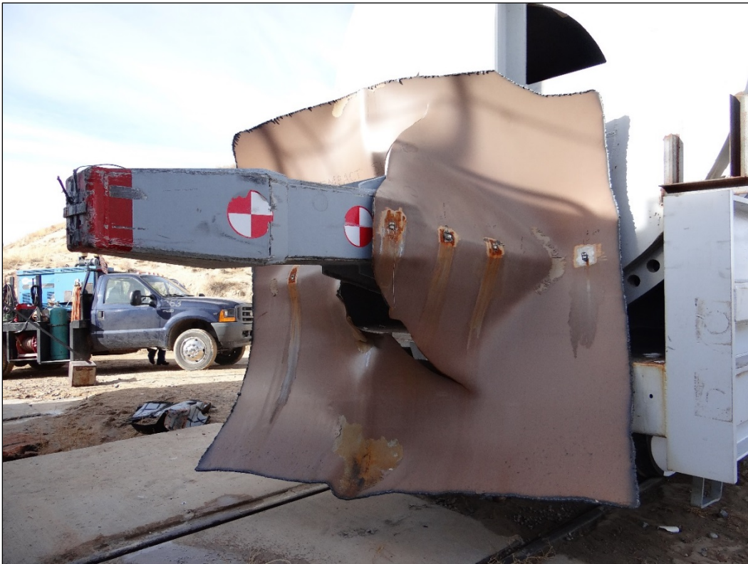
Figure A-8. Punctured Shell Removed from the Tank Car (Interior Side)
