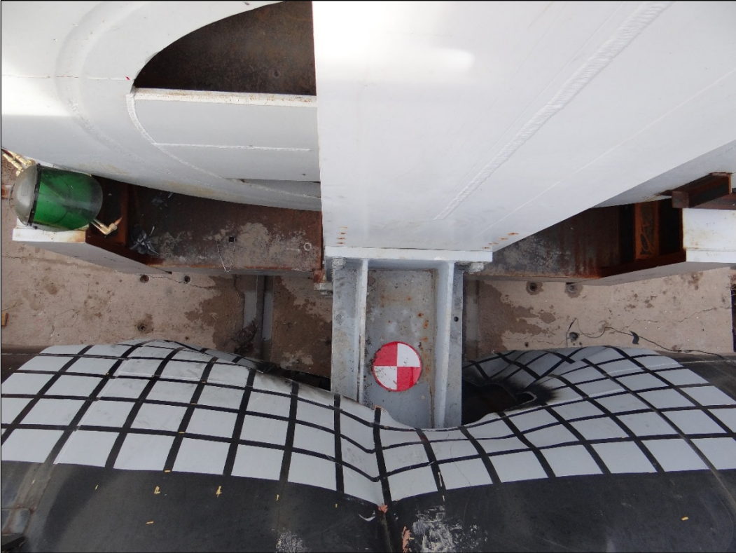
Figure A-6. Punctured Jacket after the Test
