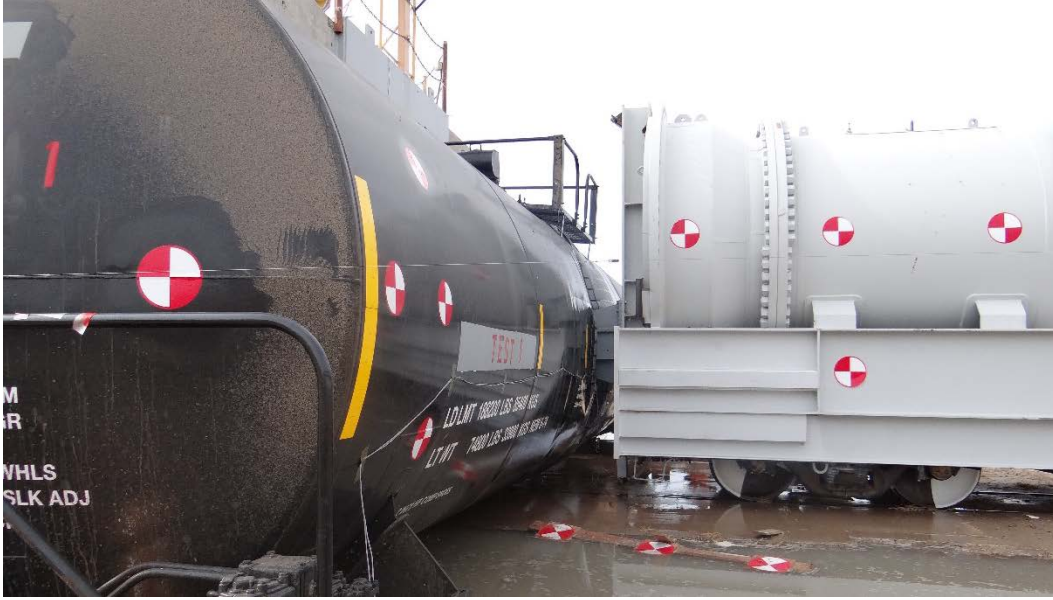
(a) Test tank car and ram car post impact
