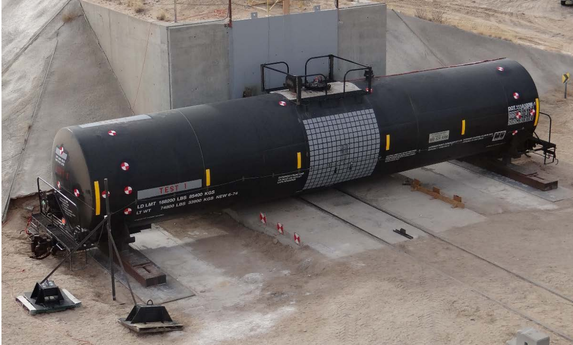
Figure 2. Target tank car mounted on support skids.
