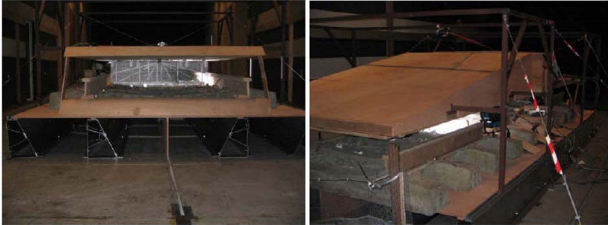
Figure 2.12: Experimental setup of the train underfloor for TGV (left) and ICE-3 (right) (Saussine and Paradot, 2008b)
