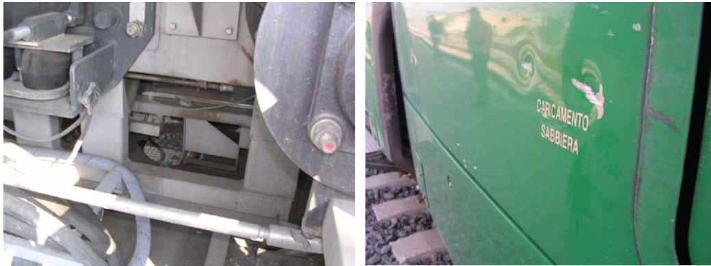
Figure 2.22: Stone embedded in the nose structure (left). Damage visible on the side of the ETR 500 due to flying ballast (right) (Agretti 2012)
