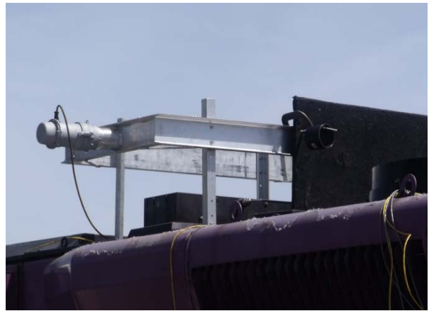
Smoke Opacity Measurement System
