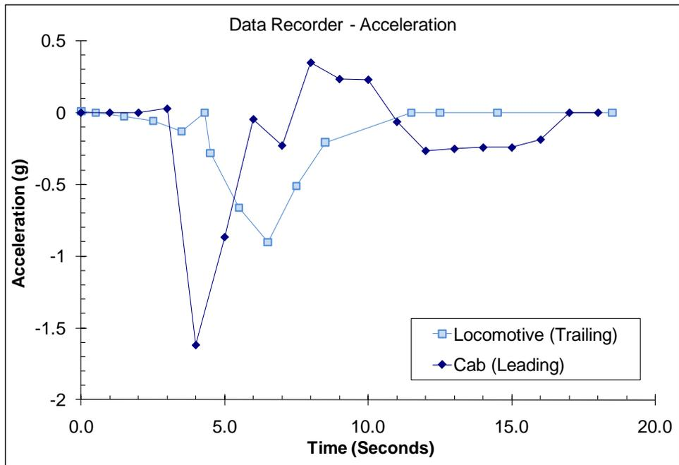
**Figure 27. Acceleration of the Locomotive and Cab Car (8570)**
