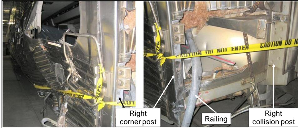
**Figure 10. Front Right of Car 7488, Looking Head-on**
