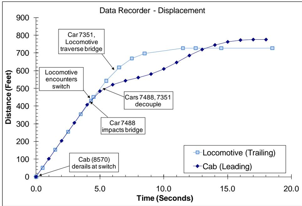
**Figure 26. Displacement of the Locomotive and Cab Car (8570)**
