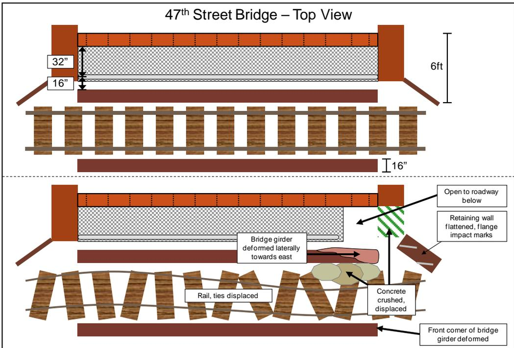
**Figure 21. Top View of the 47th Street Bridge, Showing the Structure Before (Top) and After (Bottom)**
