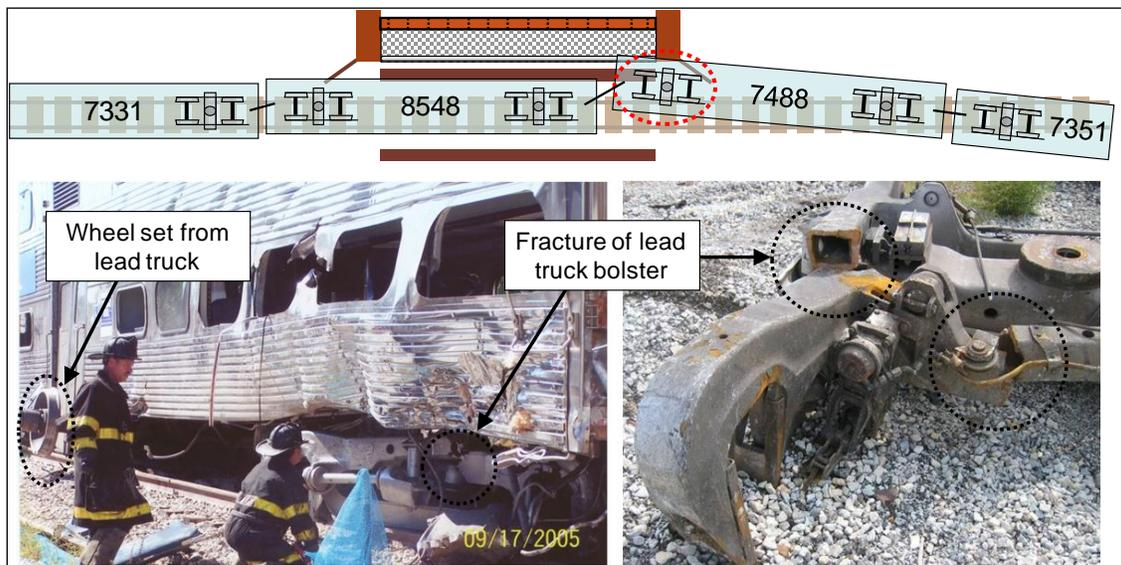
**Figure 9. Front Right Corner of Car 7488, Showing Front Truck When the Car Came to Rest and When It Was Later Removed**
