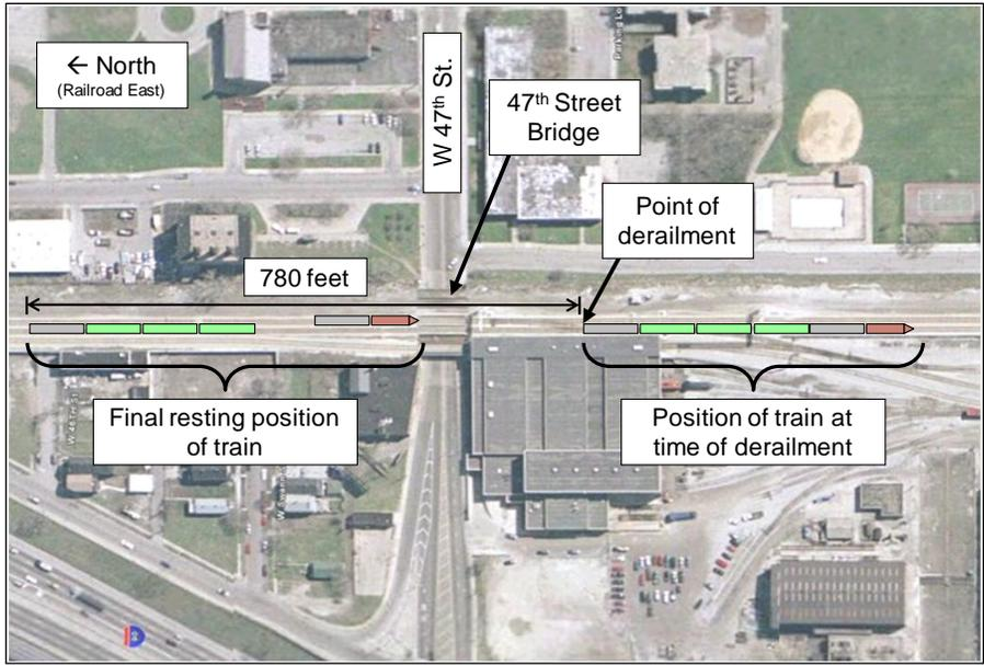
**Figure 14. Overhead View of the Scene, Showing Initial and Final Positions of the Cars**
