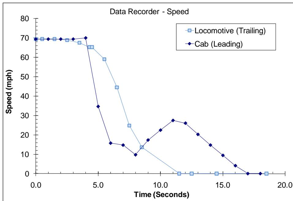
**Figure 25. Velocity-Time History of the Lead Cab Car and Trailing Locomotive, Showing the Sequence of Events**
