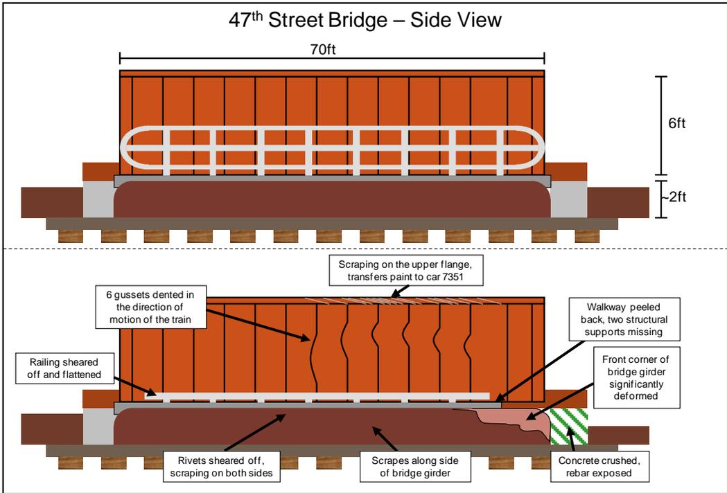
**Figure 20. Side View of the 47th Street Bridge, Showing the Structure Before (Top) and After (Bottom)**
