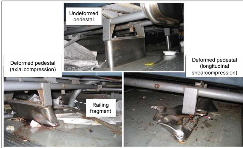
**Figure 24. Seat Pedestals in Various States in Car 7488**
