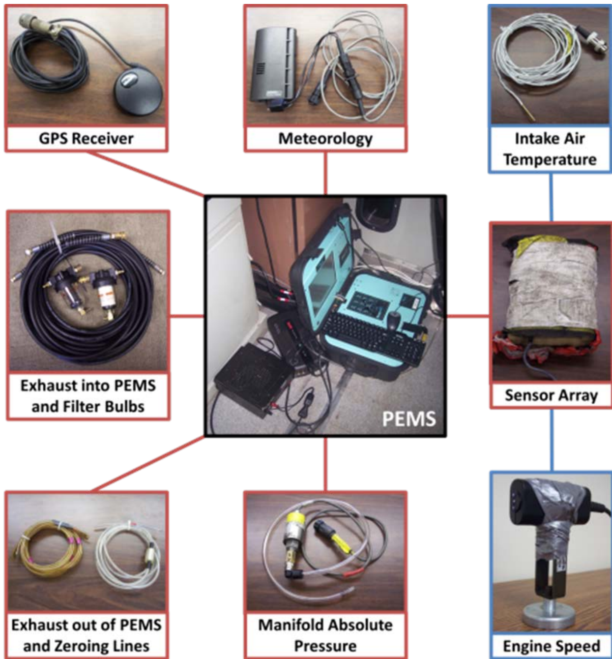
Figure 3-2. Components of the Portable Emissions Measurement System (PEMS) and Engine Sensor Array.
