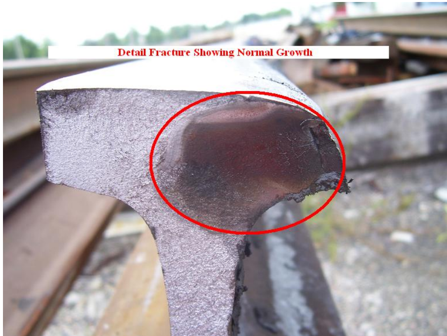
Figure 4: Detail Fracture Showing Normal Growth pattern
