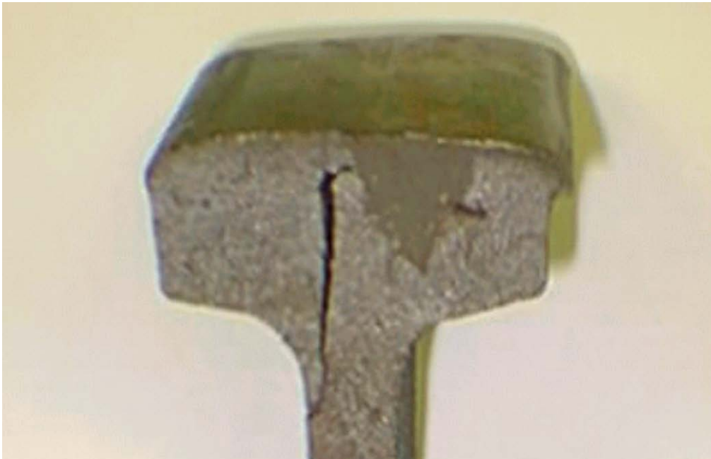
Figure 24: Vertical Split Head Defect Breaking Out in Head/Web Fillet Area
