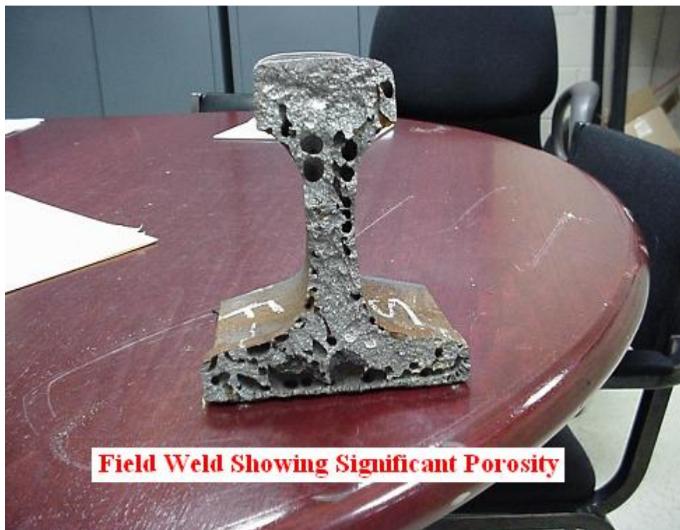
Figure 38: Thermite Weld Showing Severe Porosity
