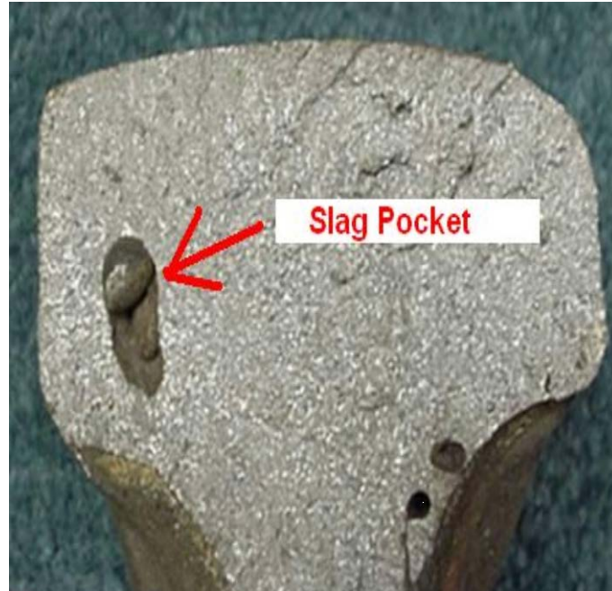
Figure 37: Thermite Weld with Slag Entrapment
