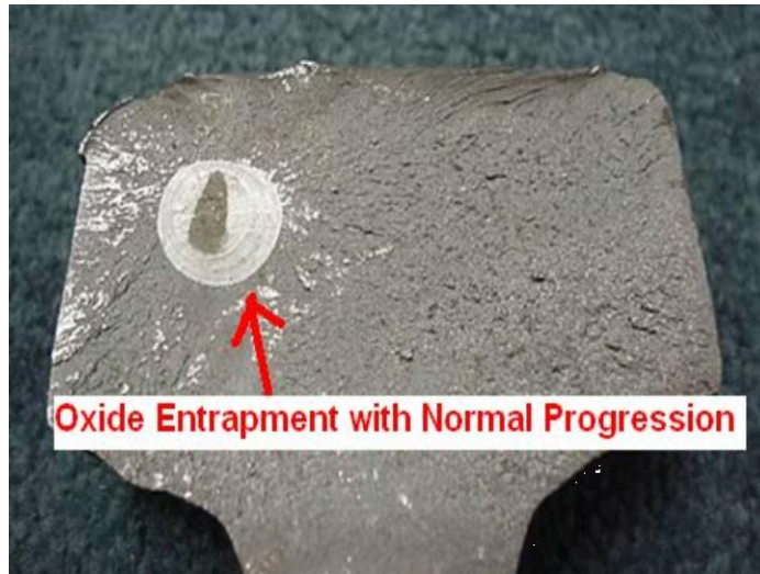
Figure 36: Electric Flash Butt Weld Showing Oxide Entrapment and Progression
