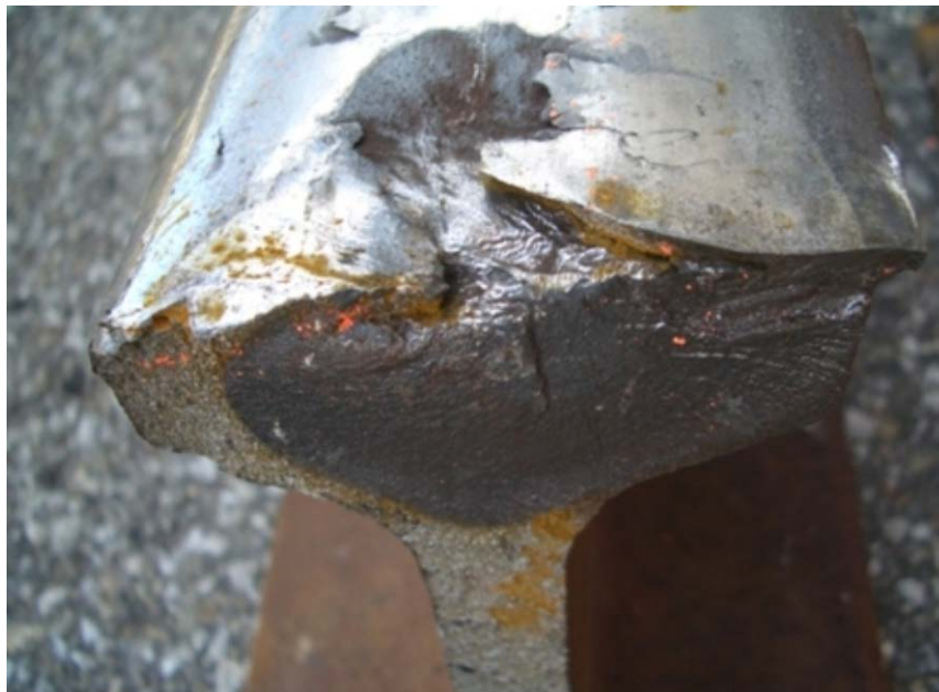
Figure 20: Engine Burn Fracture Showing Significant Growth
