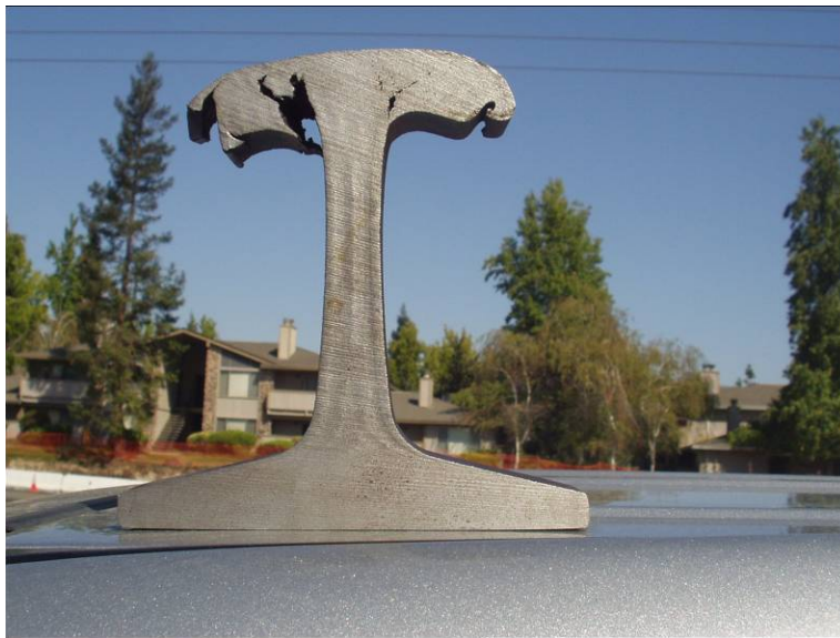
Figure 26: Vertical Split Head (Shear Break)
