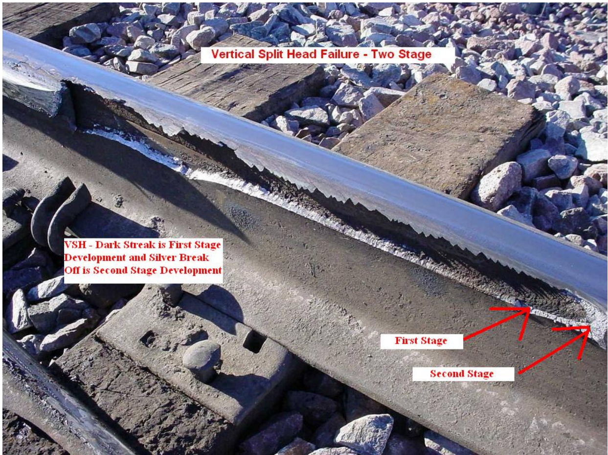
Figure 8: Vertical Split Head Showing Two-Stage Development
