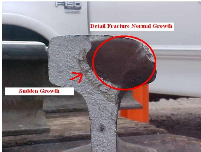
Figure 6: Detail Fracture Showing Normal and Sudden Growth Patterns
