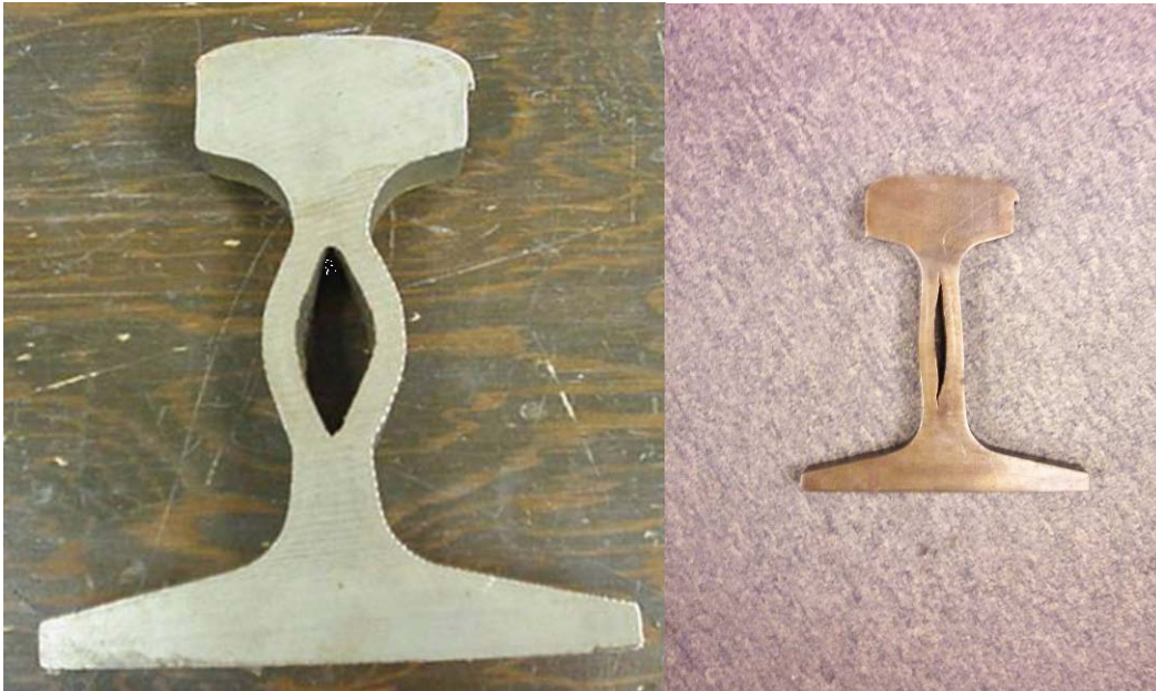
Figure 32: Piped Rail Showing Significant Rail Collapse
