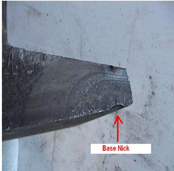
Figure 35: Base Fracture Showing Nick with Transverse Development
