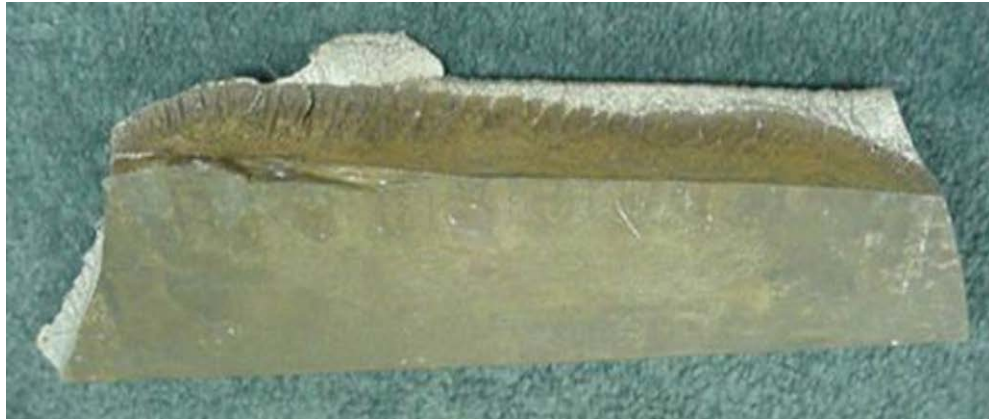
Figure 33: Base Defect Originating from an Identifiable Nick on Bottom of Rail
