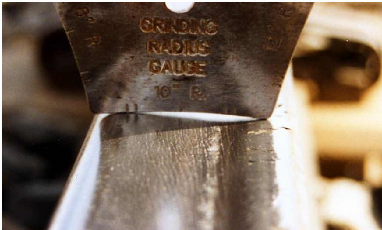
Figure 61: Worn Low Rail Profile
