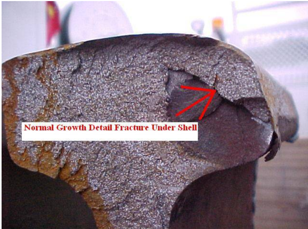
Figure 15: Detail Fracture Originating from a Visible Shell
