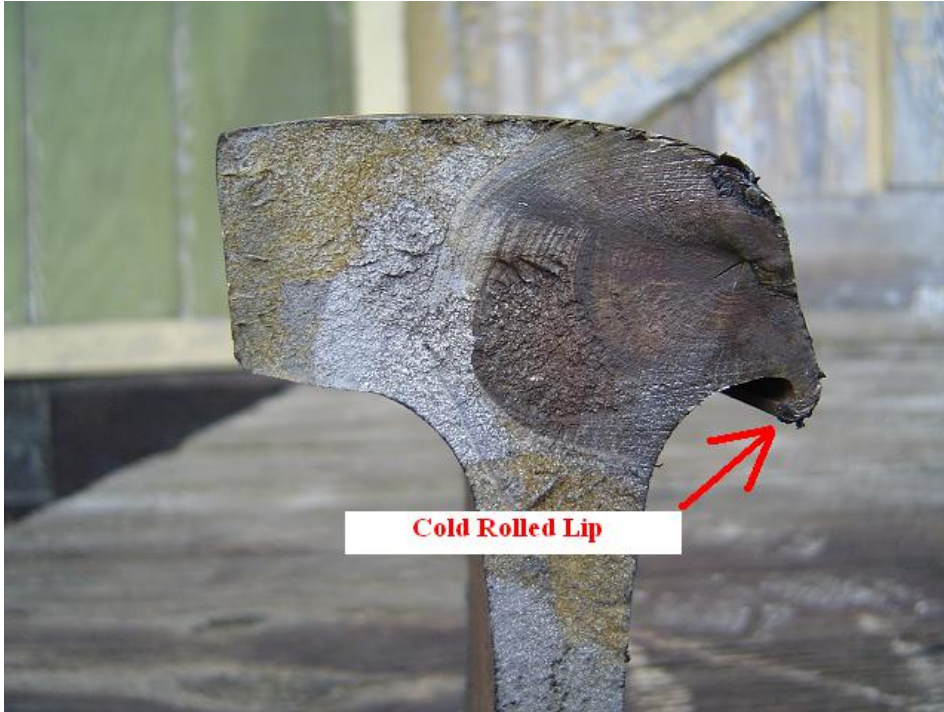
Figure 19: Reverse Detail Fracture Showing Significant Development
