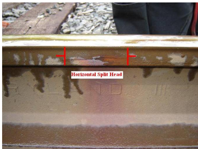
Figure 23: Side View of Horizontal Split Head
