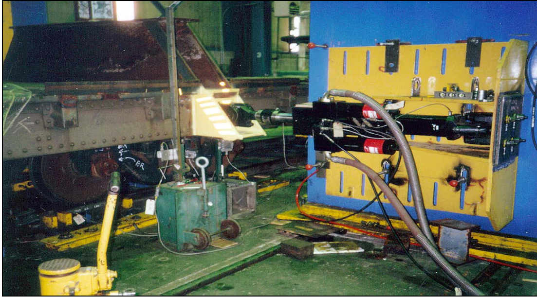
Figure 38. Mini-Shaker Unit Attached to Flat Car
