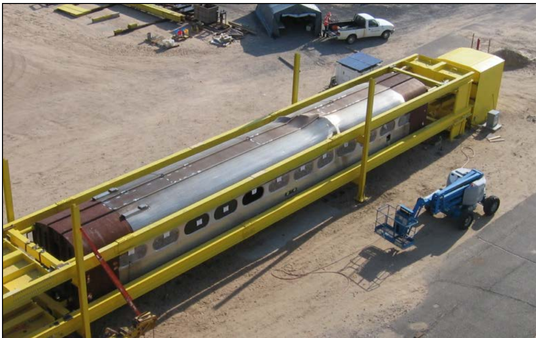
Figure 47. Squeeze Test Fixture
