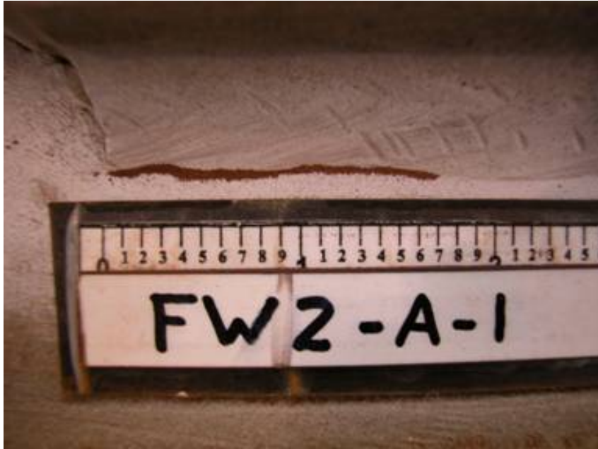
Figure 92. Fillet Weld Termination — MT
