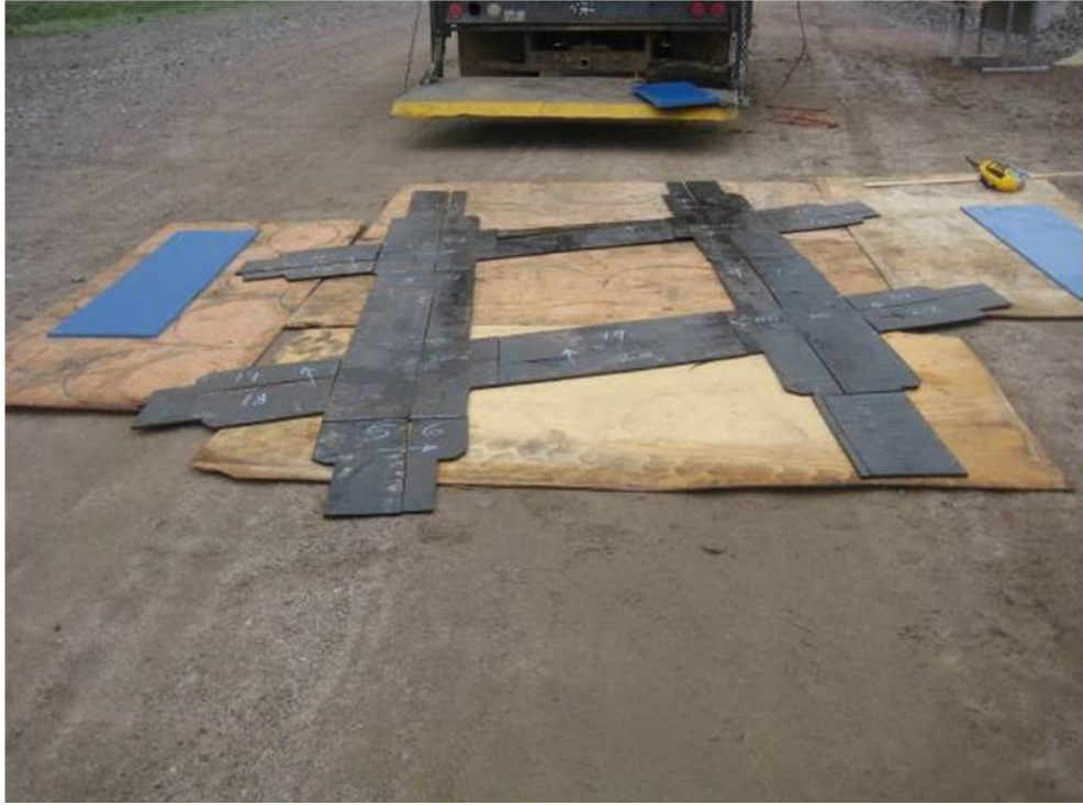
Figure 15. Getzner Type A pad intended for under-tie use was tested as a full-coverage rail seat pad
