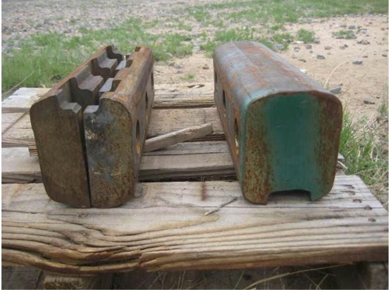
Figure 12. Split flangeway spacer on the left. Solid spacer for use with through bolts on the right (upside down in the photo)
