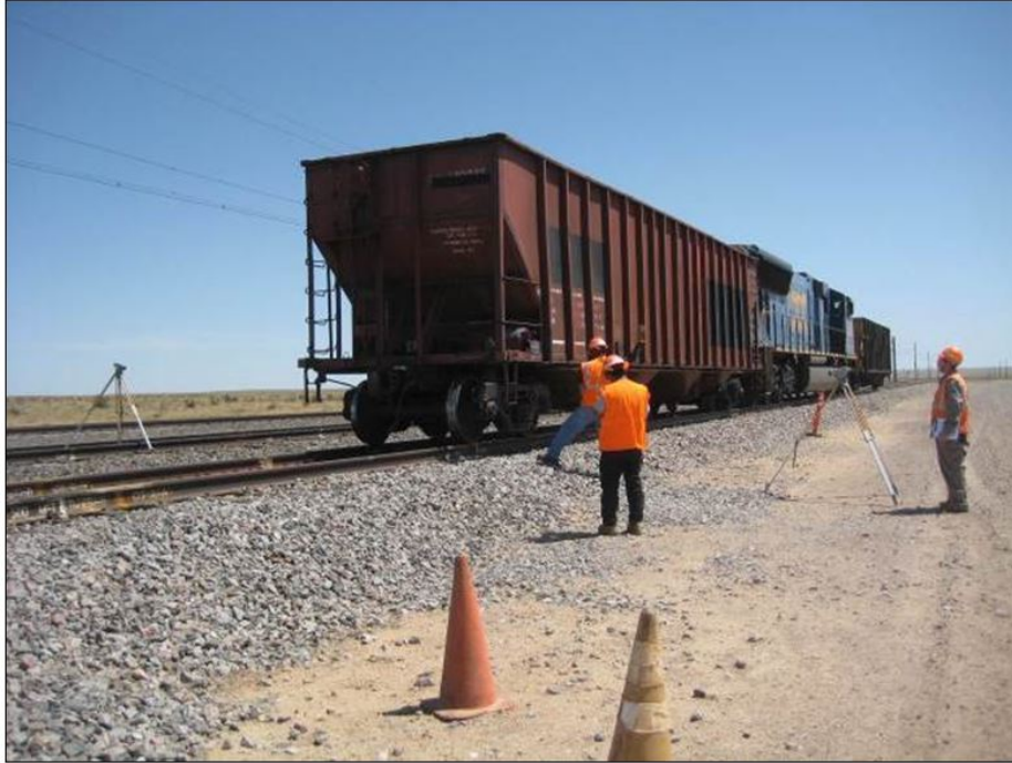
Figure 26. Vertical stiffness: light and heavy cars used to load the track vertically. The survey equipment is used to measure the resulting track deflection.
