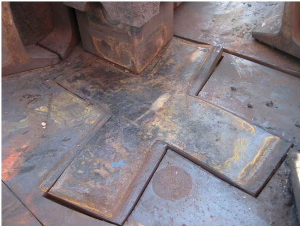
Figure 96. Getzner Type B full-coverage pad with separate under-tile piece performing well after 27 MGT
