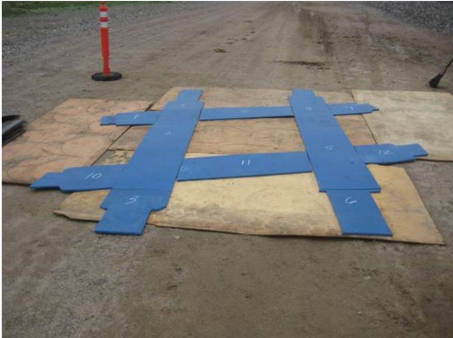
Figure 17. Getzner pad Type B cut to size. This is the Getzner pad type intended for use in the full-coverage rail seat configuration
