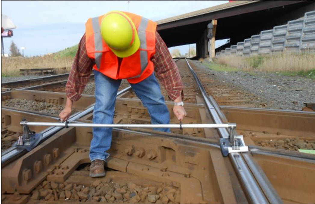
Figure 30. TTCI's prototype Effective Flangeway Gap and Wheel Drop gage in wheel gap measurement mode at a revenue service crossing diamond
