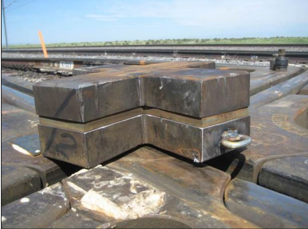
Figure 20. The steel flangeway spacer tile was cut in half and \frac{1}{4} in of material was milled from each half to accommodate a layer of the \frac{1}{2} -in Getzner Type C pad material
