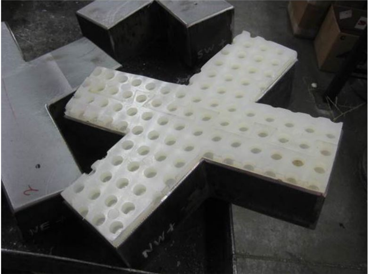
Figure 14. Nortrak pad material was cut and placed under the flangeway spacer tile to evaluate the effect of double padding
