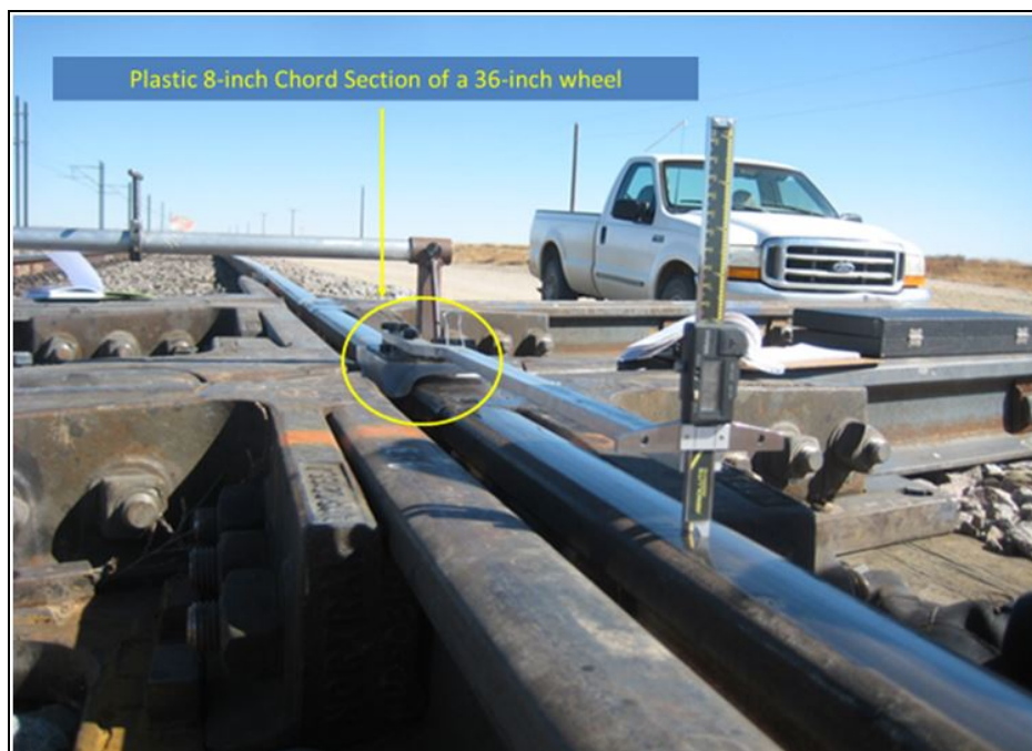
Figure 29. TTCI's prototype Effective Flangeway Gap and Wheel Drop gage in wheel drop measurement mode
