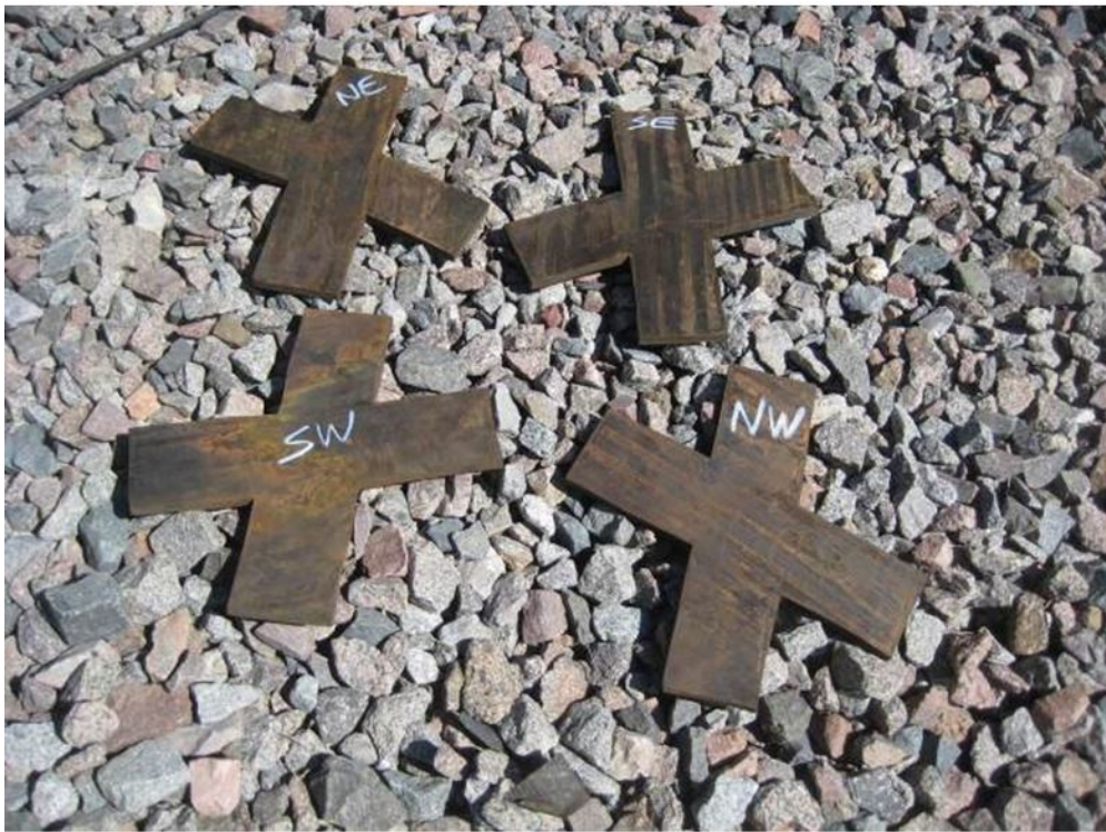
Figure 16. The Getzner Type C pad designed for the layered configuration of Test Case 9 was used to evaluate the effect of double padding under the flangeway spacer tile
