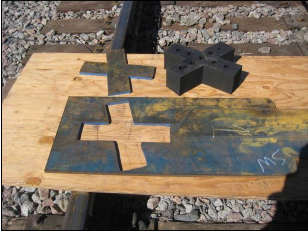
Figure 21. The solid rubber flangeway spacer tile and its shape cut out of the full-coverage rail seat section of Getzner Type B pad that fits directly under the tile
