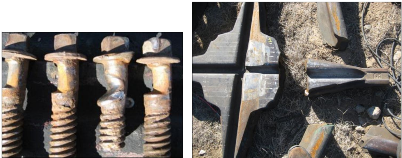
Figure 4. Components Failures in Cast Crossing
