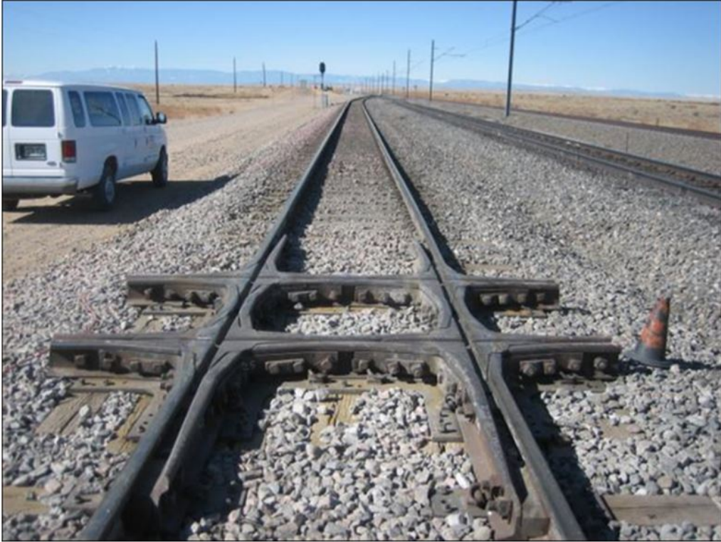
Figure 2. Cast Diamond Crossing Tested at FAST
