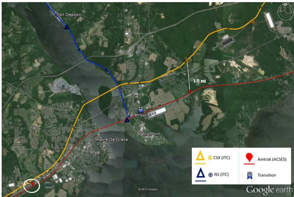
Figure 24. Typical Transition Case between NS and Amtrak
