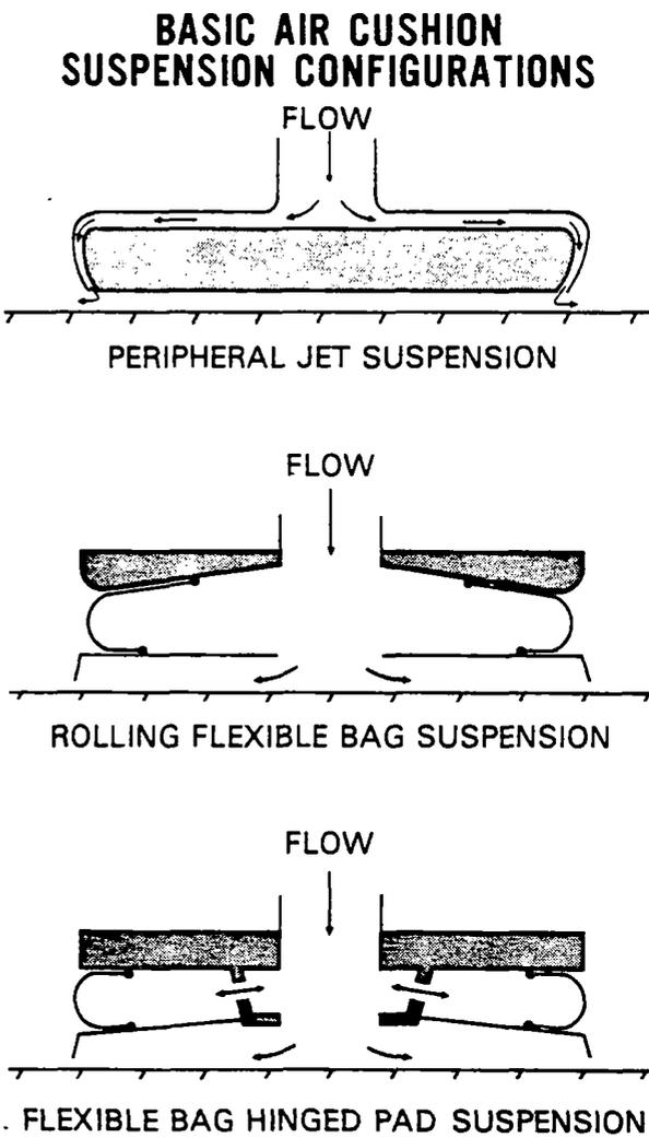
Figure 2. Different Designs of Air Cushion
