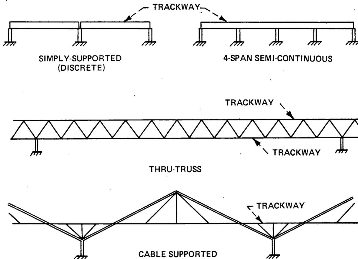
Figure 14. Elevated Guideway Design Concepts
