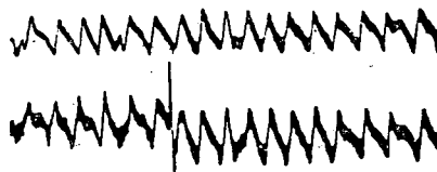
Fig. 127 Sample of a record of surface damage in the metal of the rail head.
