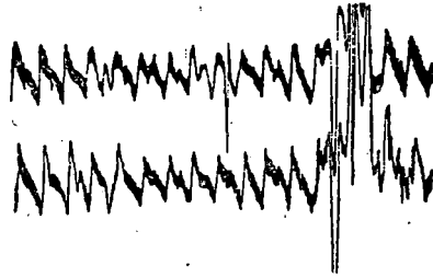
Fig. 128 A record of the 21.2 flaw on film.
