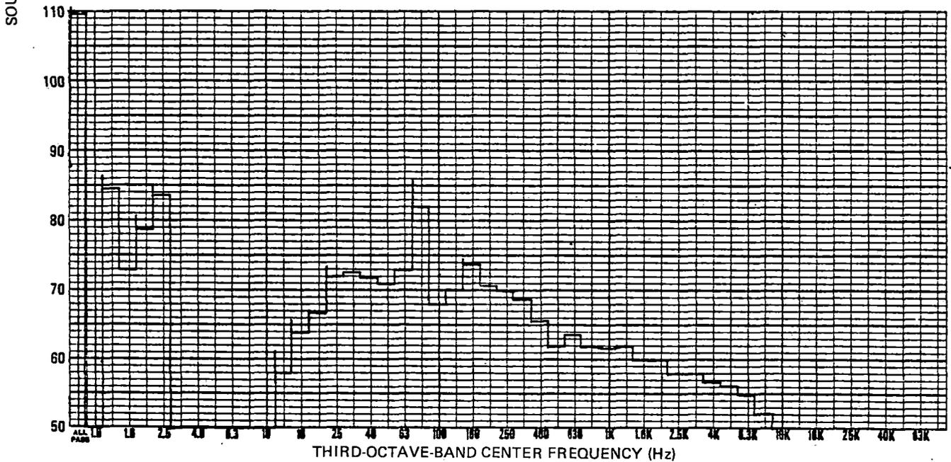
Figure 3-17. Third-Octave-Band Analysis of SFMR Interior Noise, AWO, 15 mph
