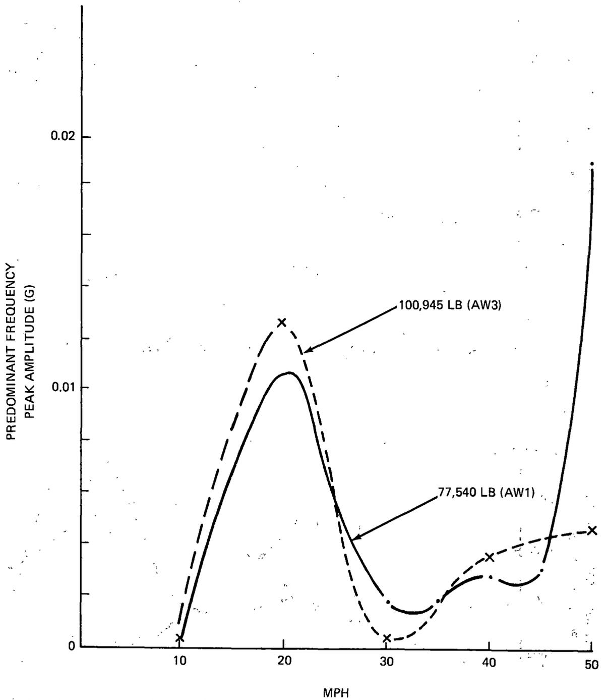
Figure 2-6. Effect of Speed and Weight on Longitudinal Ride Roughness, End Car
