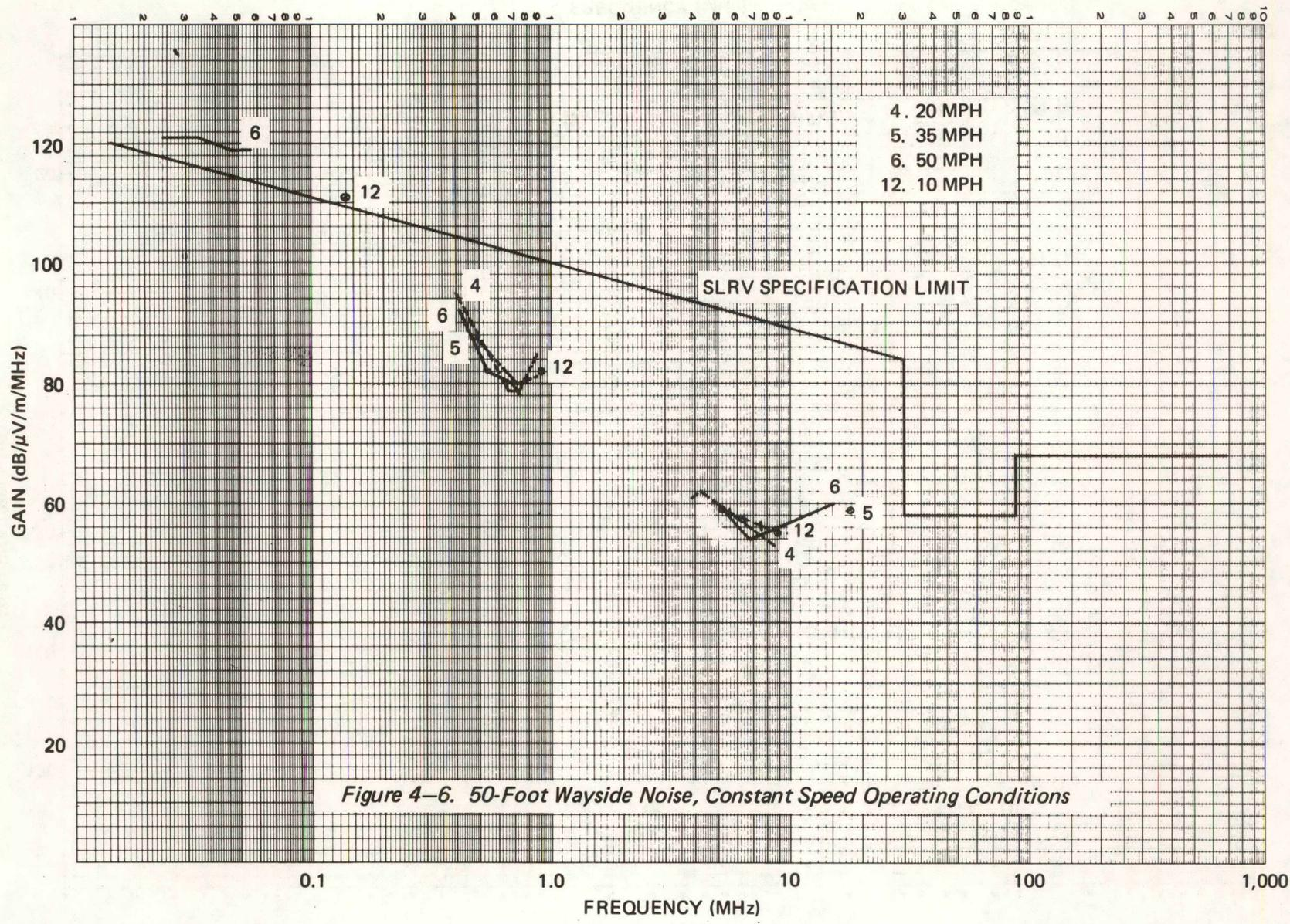
Figure 4-6. 50-Foot Wayside Noise, Constant Speed Operating Conditions
