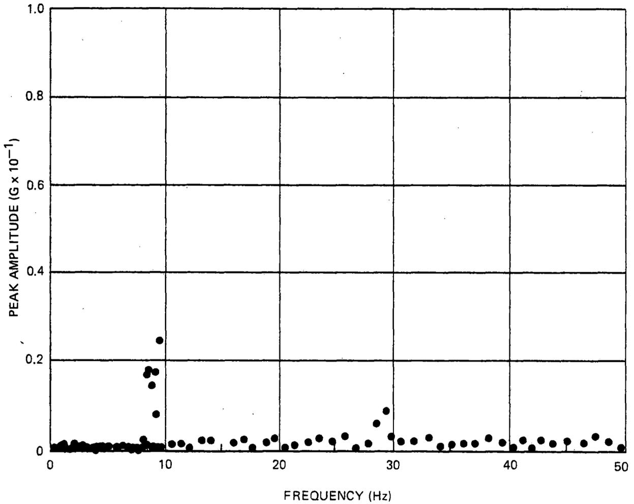
Figure A-4. Narrow-Band Spectrum Analysis – Mid Car, Vertical
