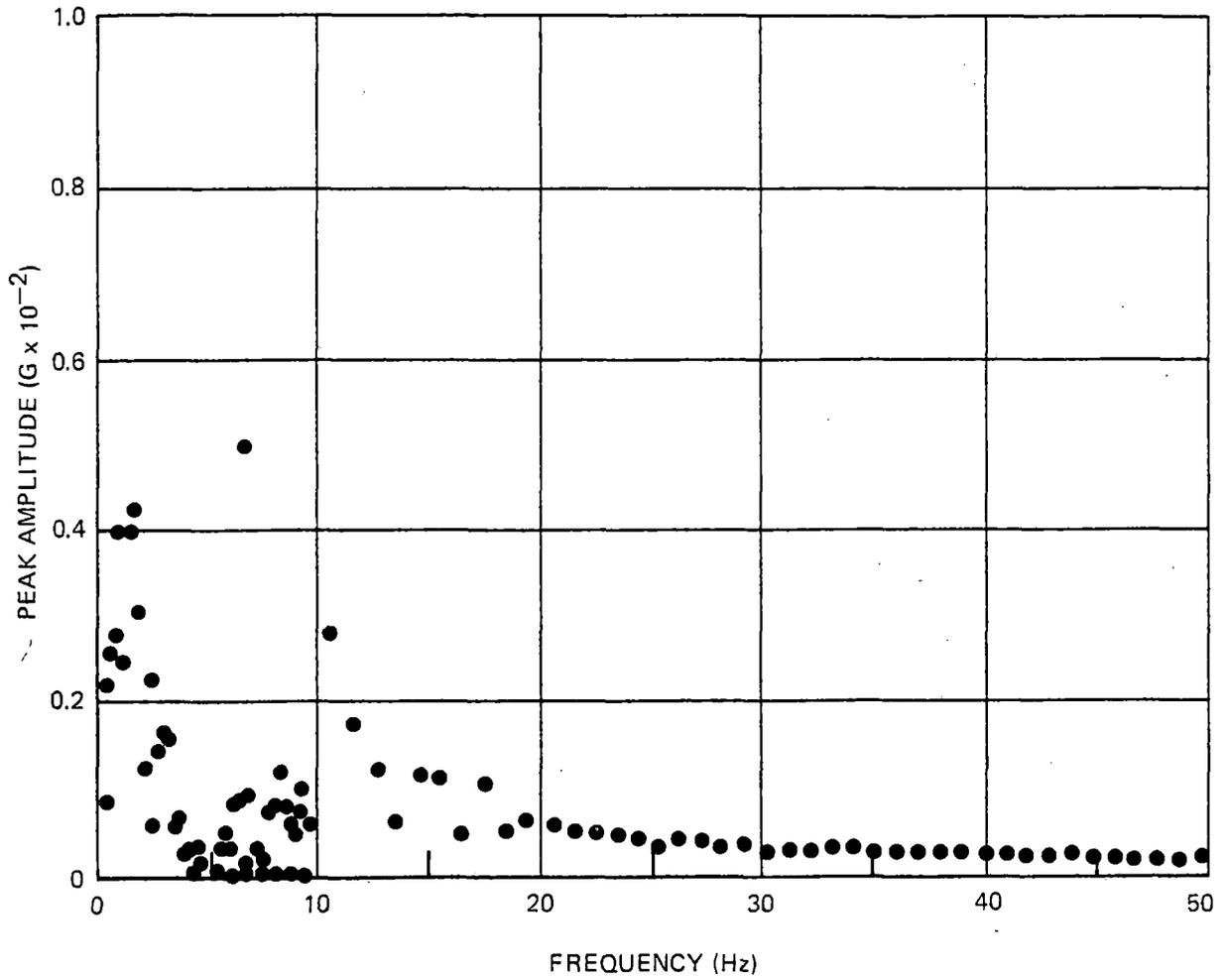
Figure A-31. Narrow-Band Spectrum Analysis – End Car, Vertical
