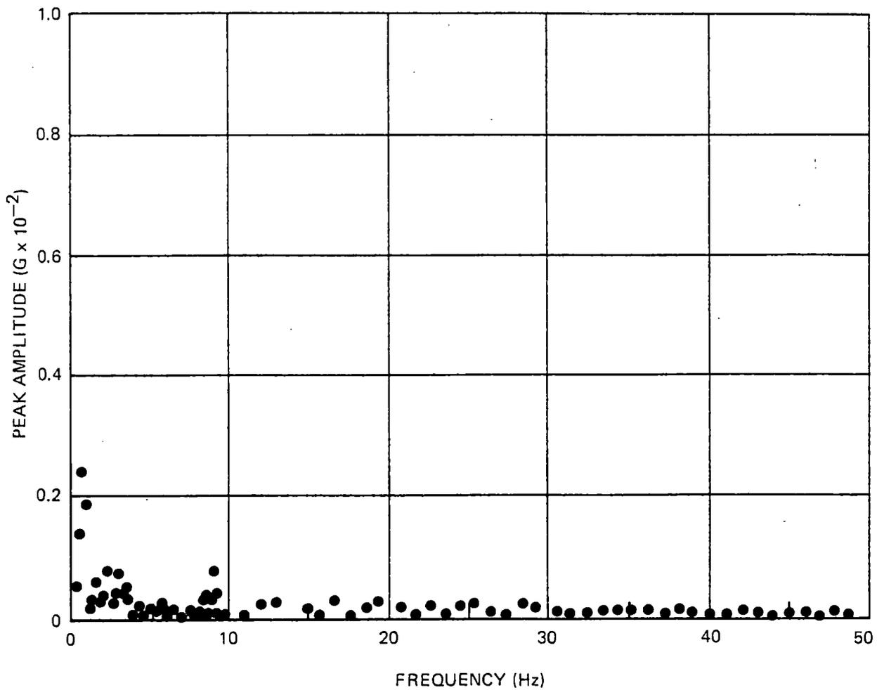
Figure A-37. Narrow-Band Spectrum Analysis — End Car, Lateral
