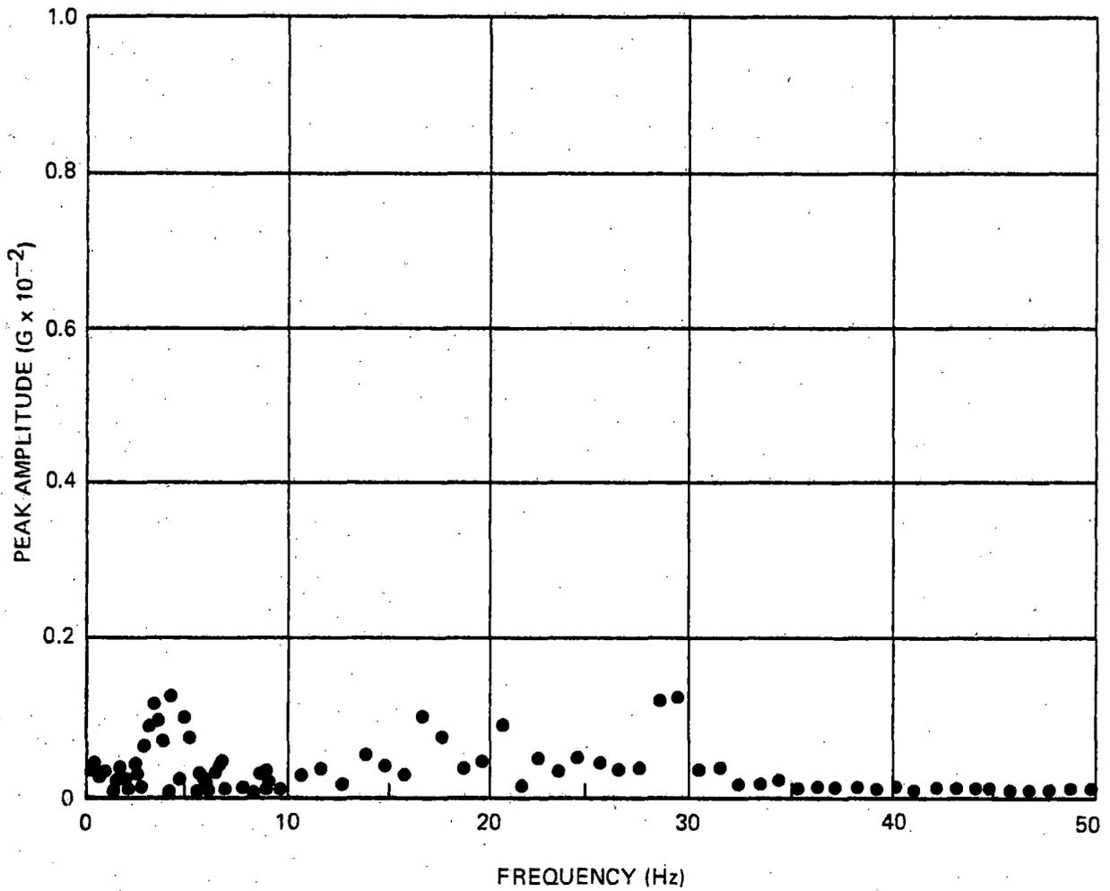
Figure A-10. Narrow-Band Spectrum Analysis - Mid Car, Lateral
