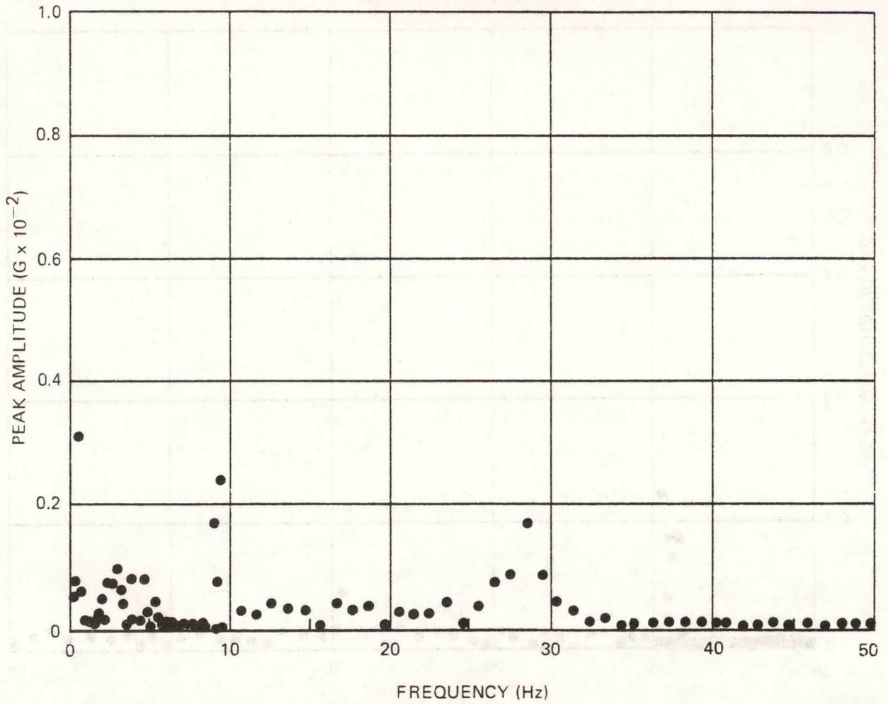
Figure A-5. Narrow-Band Spectrum Analysis — Mid Car, Lateral
