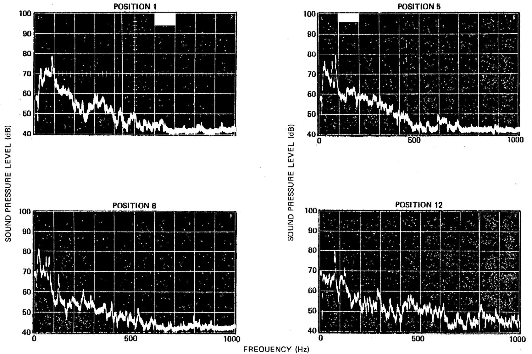
Figure 3-47. Narrowband Analysis of Interior Noise, SFMR, AWD, 50 mph
