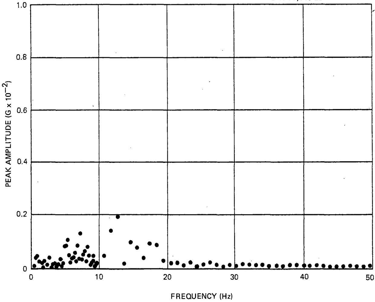
Figure A-18. Narrow-Band Spectrum Analysis – End Car, Longitudinal
