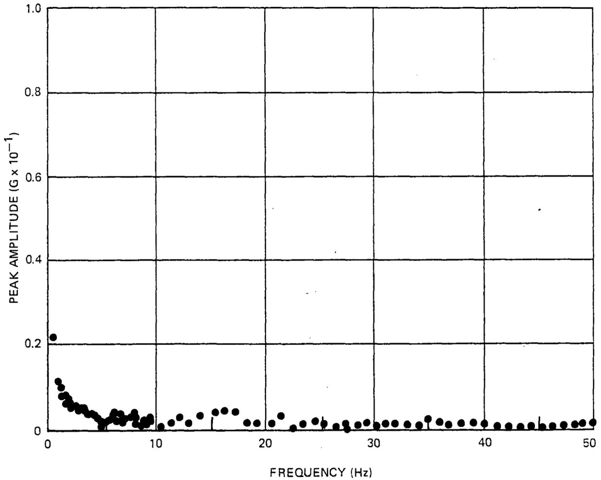
Figure A-33. Narrow-Band Spectrum Analysis — End Car, Longitudinal
