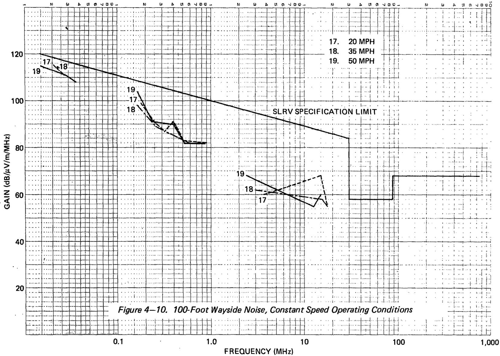
Figure 4-10. 100-Foot Wayside Noise, Constant Speed Operating Conditions
