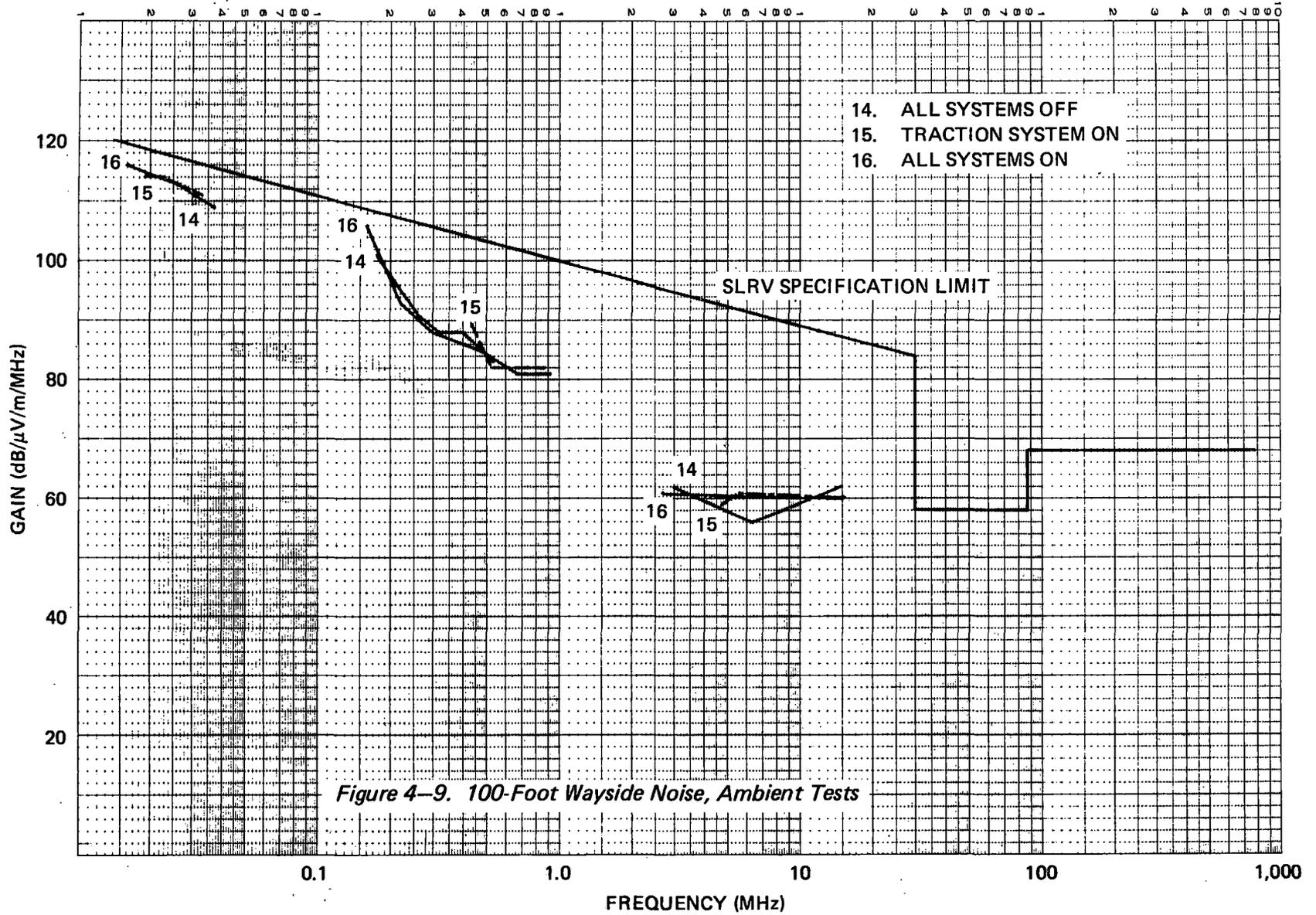
Figure 4-9. 100-Foot Wayside Noise, Ambient Tests
