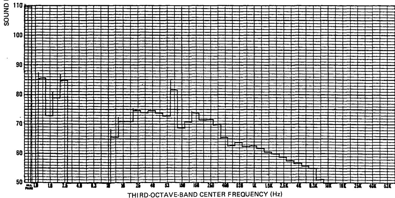
Figure 3-21. Third-Octave-Band Analysis of SFMR Interior Noise, AWO, 35 mph
