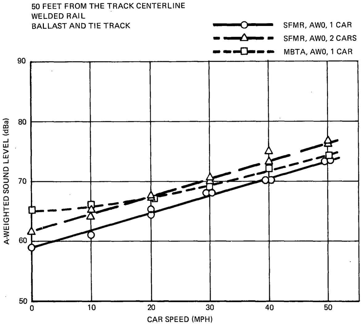
Figure 3-12. SLRV Wayside Passby Noise at Different Speeds
