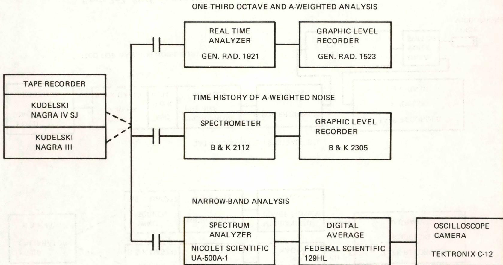
Figure 3-3. Block Diagram for Data Acquisition and Reduction Systems (Sheet 2 of 2)
