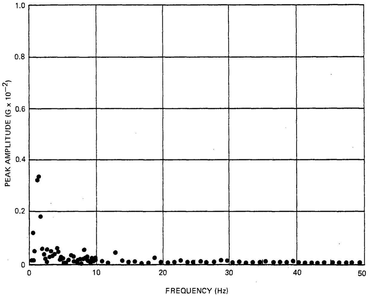
Figure A-6. Narrow-Band Spectrum Analysis – End Car, Vertical
