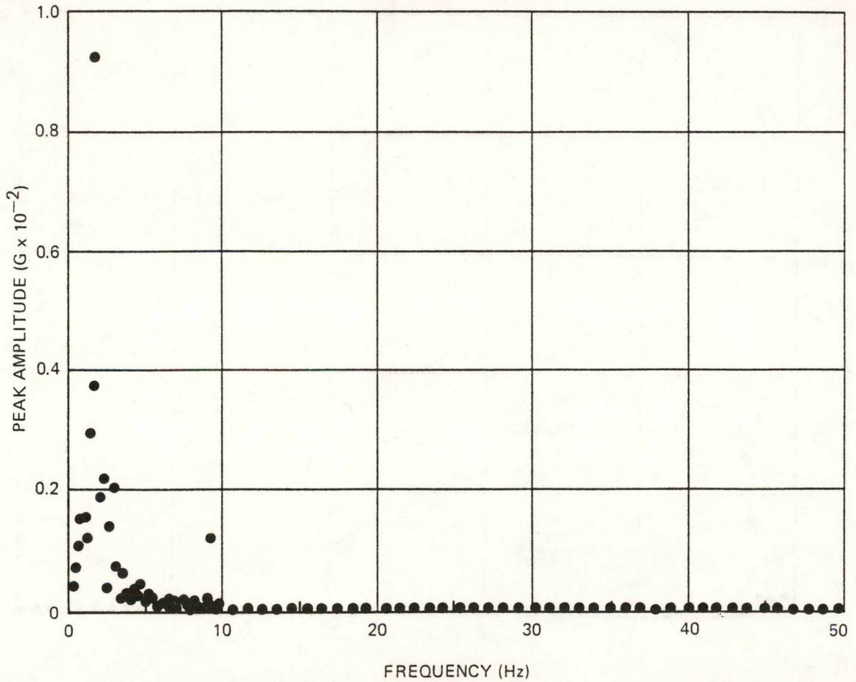
Figure A-27. Narrow-Band Spectrum Analysis – End Car, Lateral
