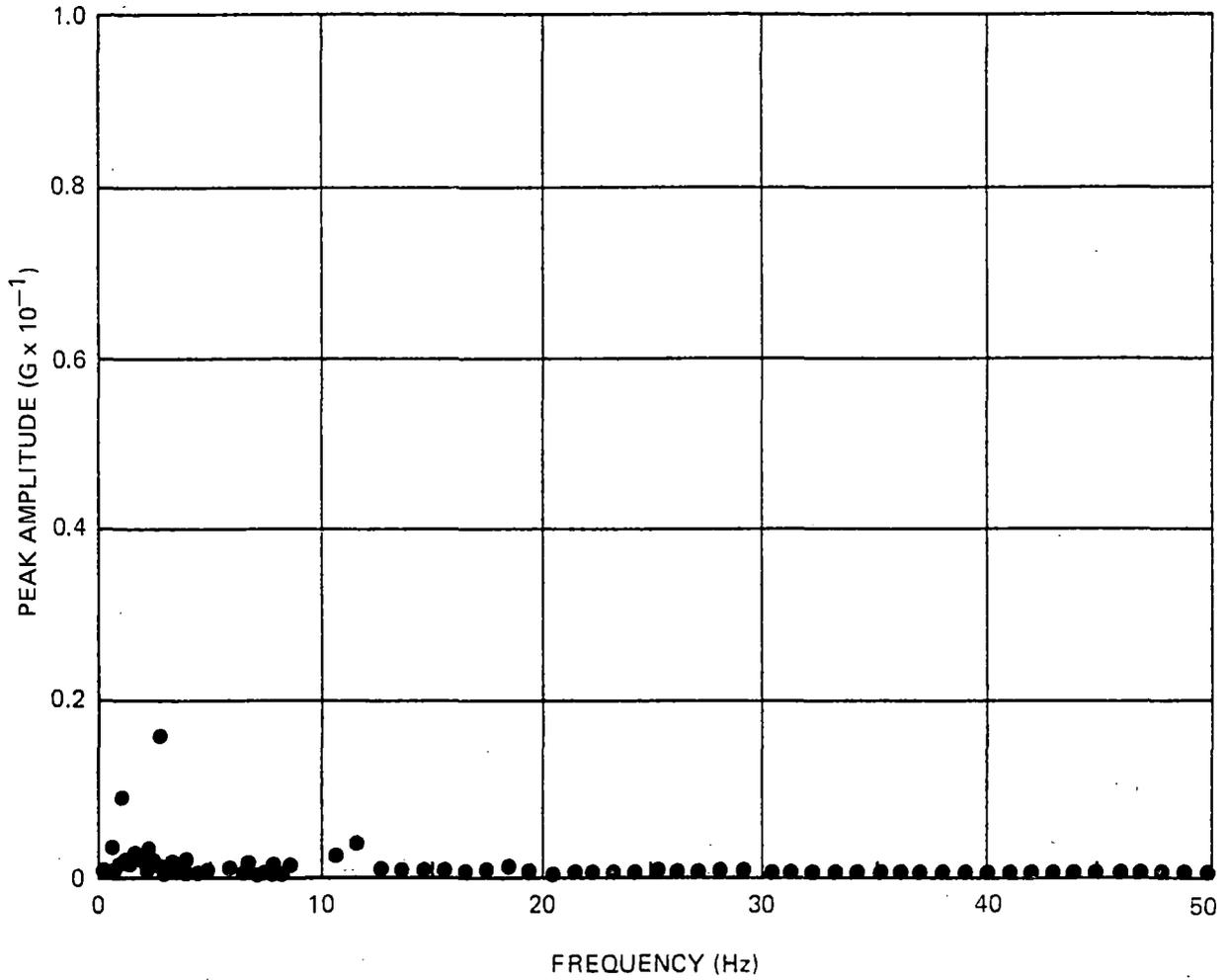
Figure A-26. Narrow-Band Spectrum Analysis — End Car, Vertical
