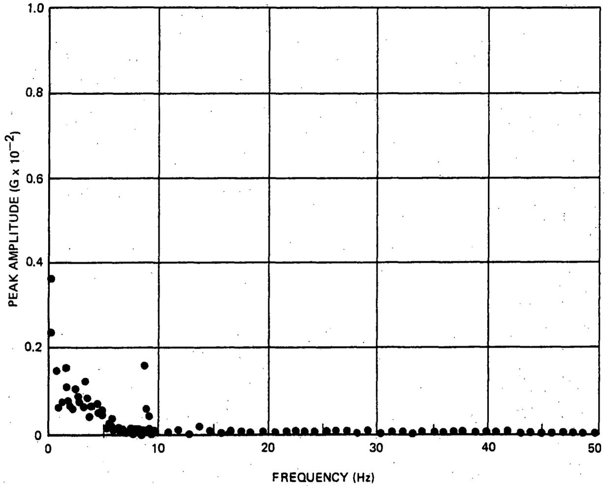
Figure A-56. Narrow-Band Spectrum Analysis – End Car, Longitudinal
