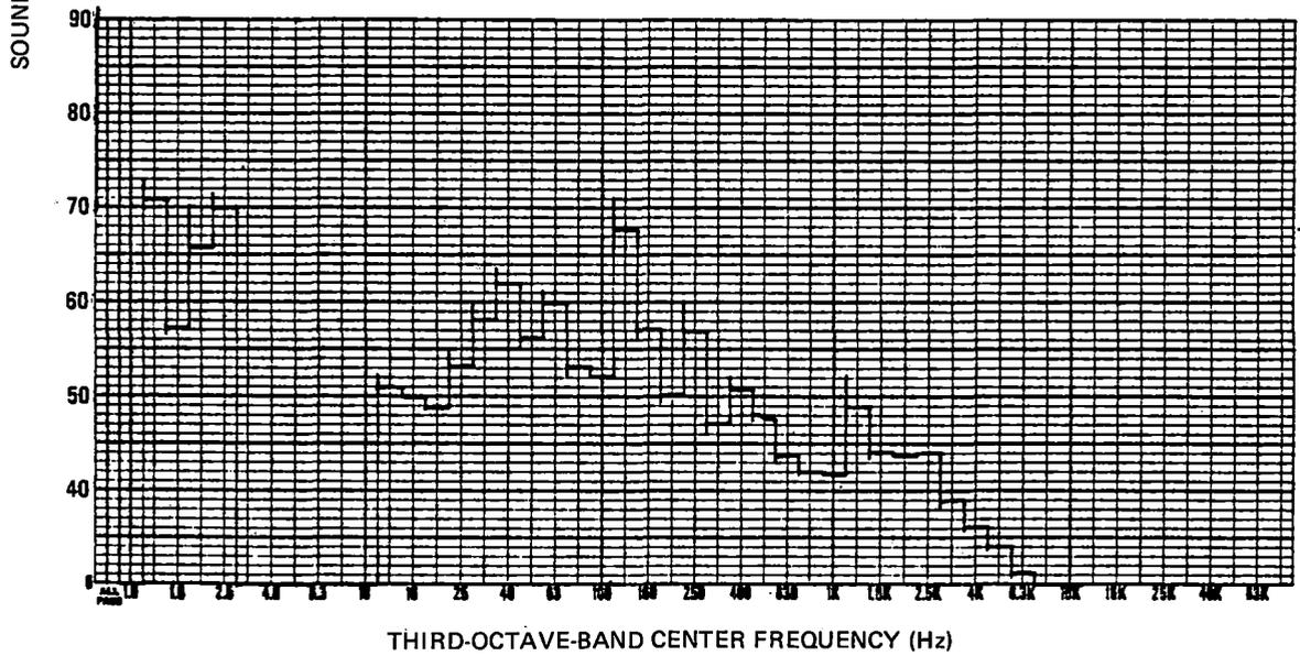
Figure 3-6. SLRV Equipment Noise, 50-Ft Wayside, Third-Octave Analysis
