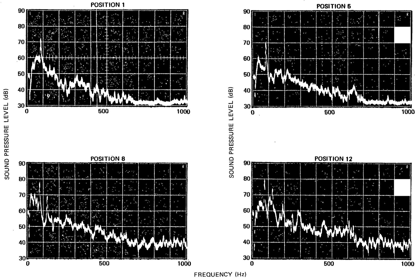
Figure 3-45. Narrowband Analysis of Interior Noise, SFMR, AW0, 25 mph
