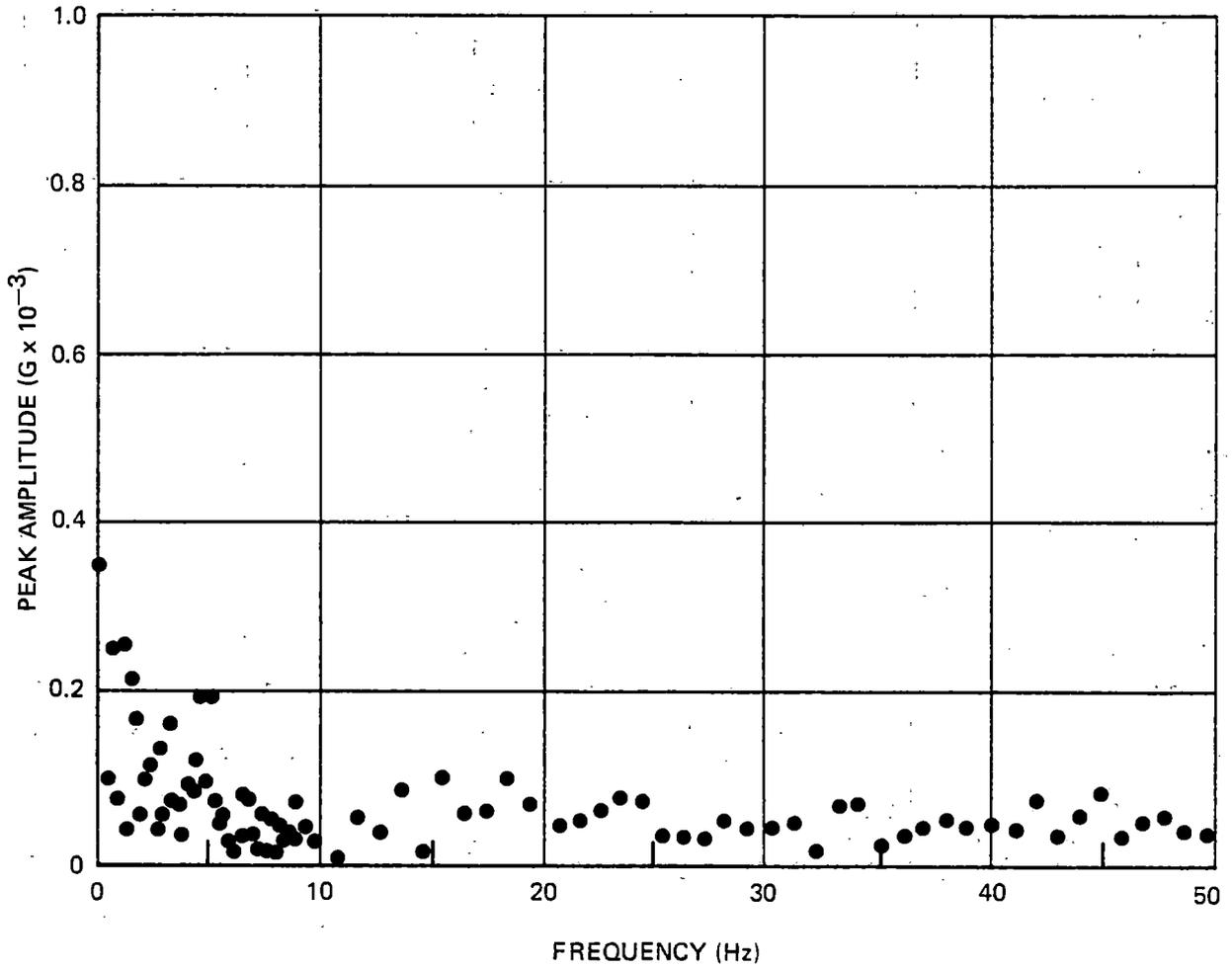
Figure A-38. Narrow-Band Spectrum Analysis — End Car, Longitudinal
