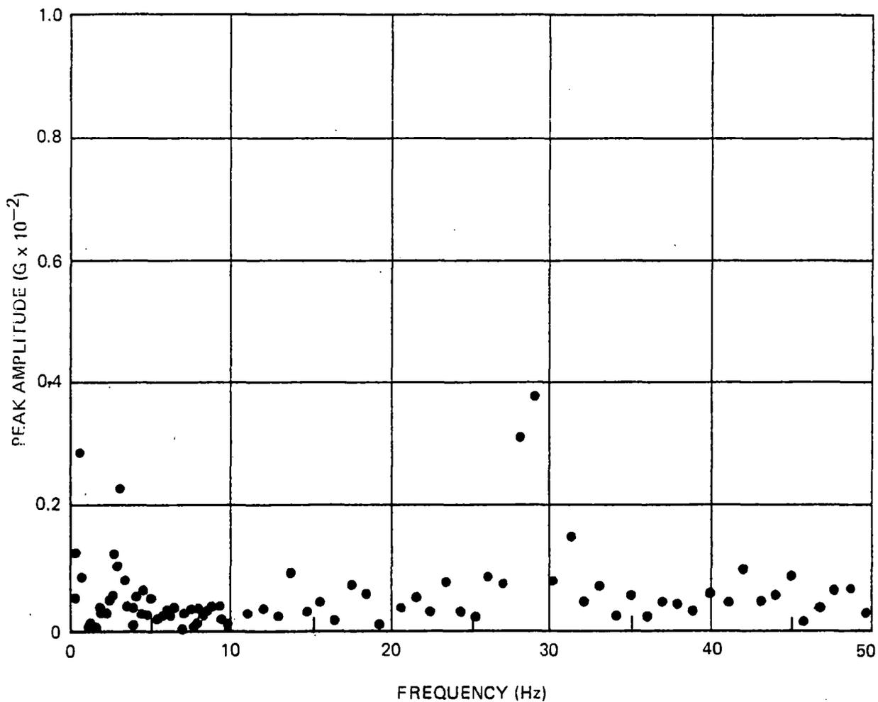
Figure A-40. Narrow-Band Spectrum Analysis – Mid Car, Lateral
