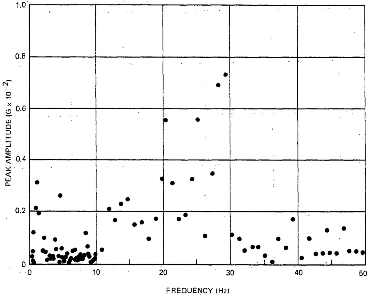
Figure A-9: Narrow-Band Spectrum Analysis — Mid Car, Vertical
