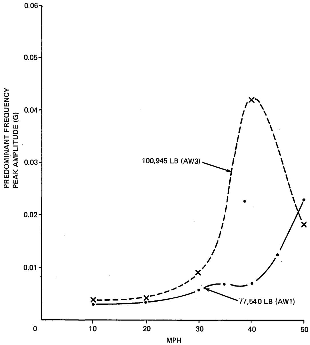
Figure 2-8. Effect of Speed and Weight on Lateral Ride Roughness, Mid Car
