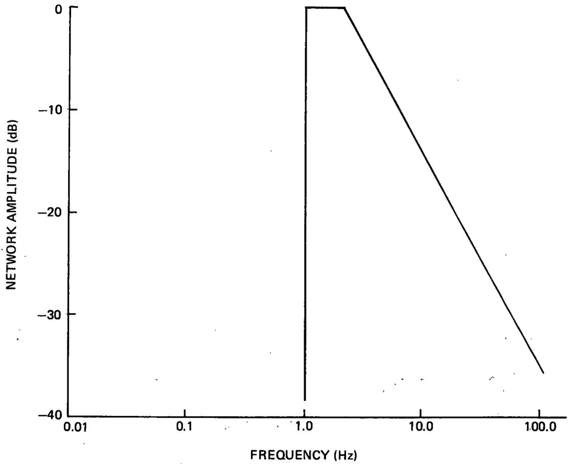
*Figure 2-2. Weighting Network Frequency Response for Horizontal Ride Roughness*
