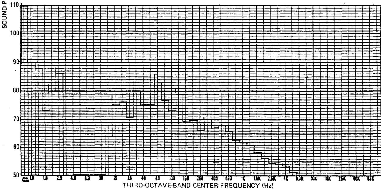
Figure 3-26. Third-Octave-Band Analysis of MBTA Interior Noise, AWO, 15 mph
