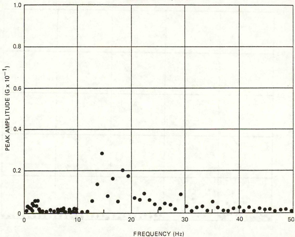
Figure A-19. Narrow-Band Spectrum Analysis – Mid Car, Vertical
