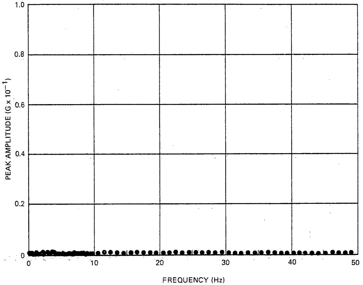
*Figure A-3. Narrow-Band Spectrum Analysis – End Car, Longitudinal*
