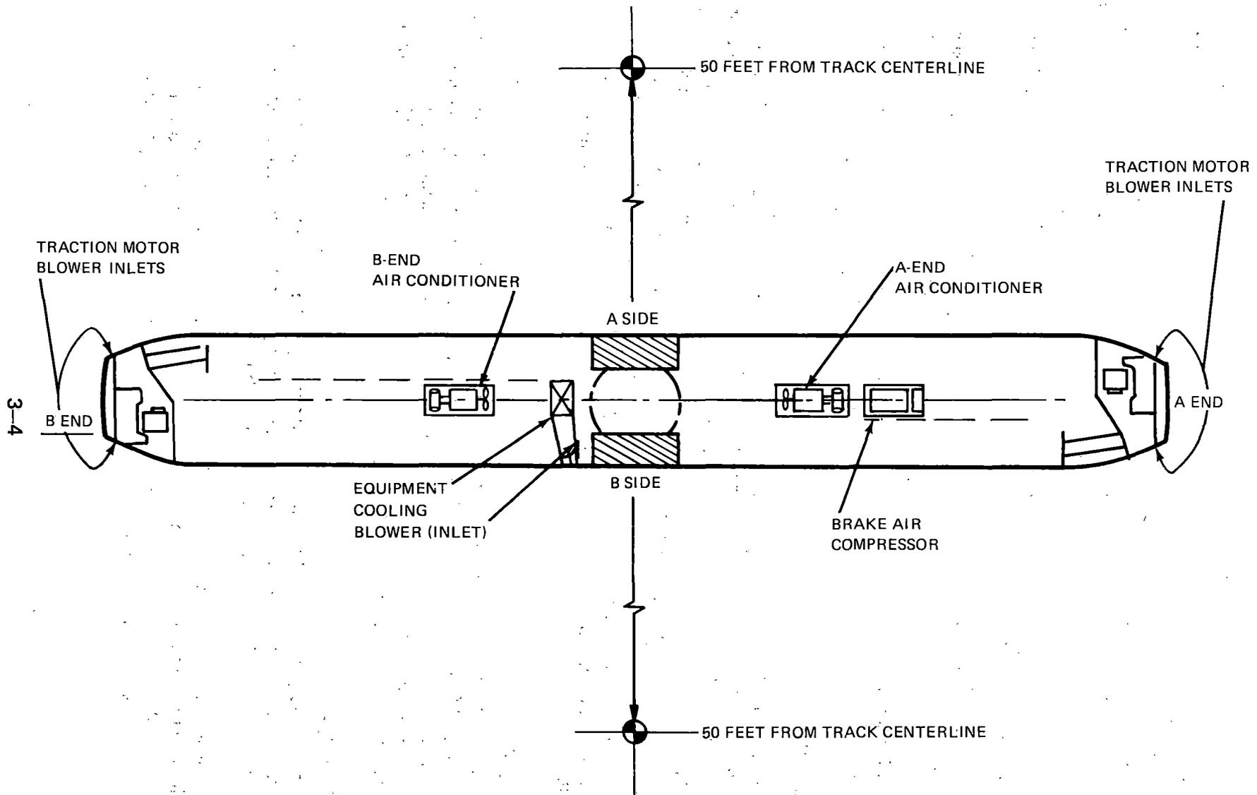
Figure 3-2. SLRV Undercar Equipment Measured for Wayside Noise
