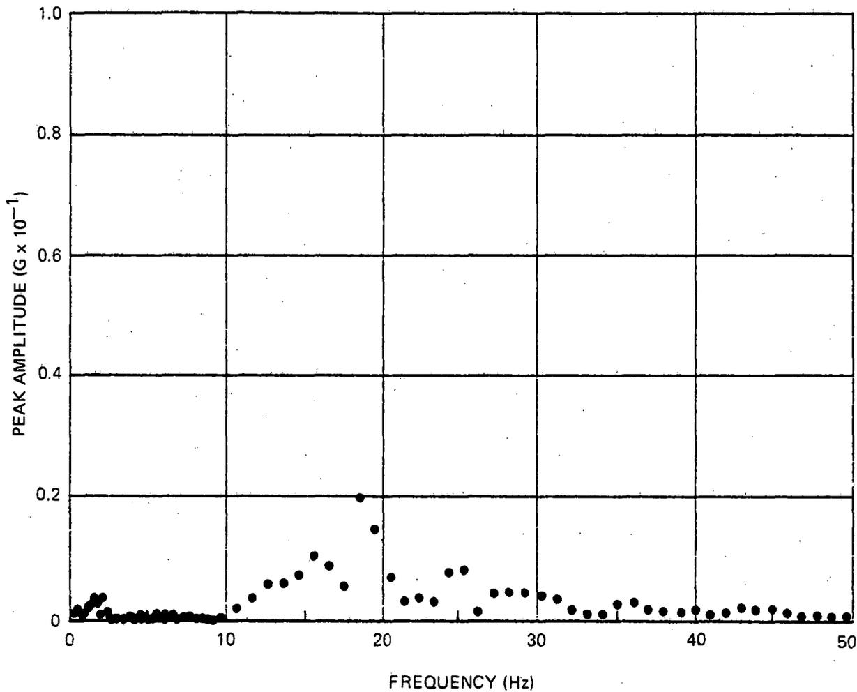
Figure A-14. Narrow-Band Spectrum Analysis — Mid Car, Vertical
