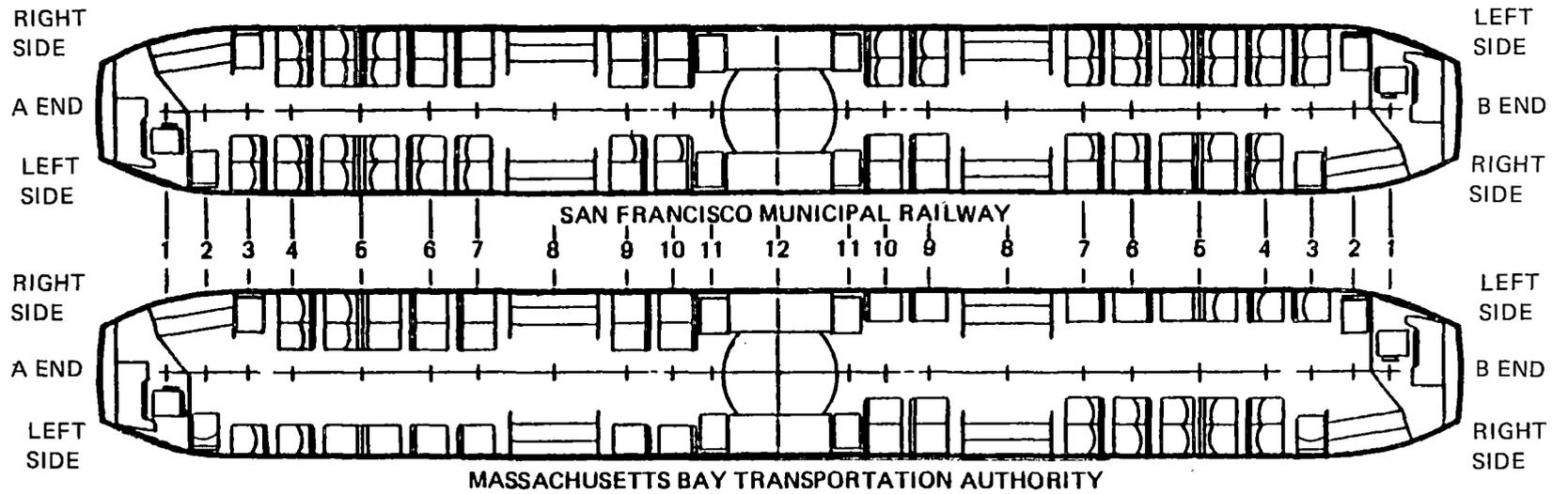
Figure 3-13. Measurement Locations for SLRV Interior Noise Survey
