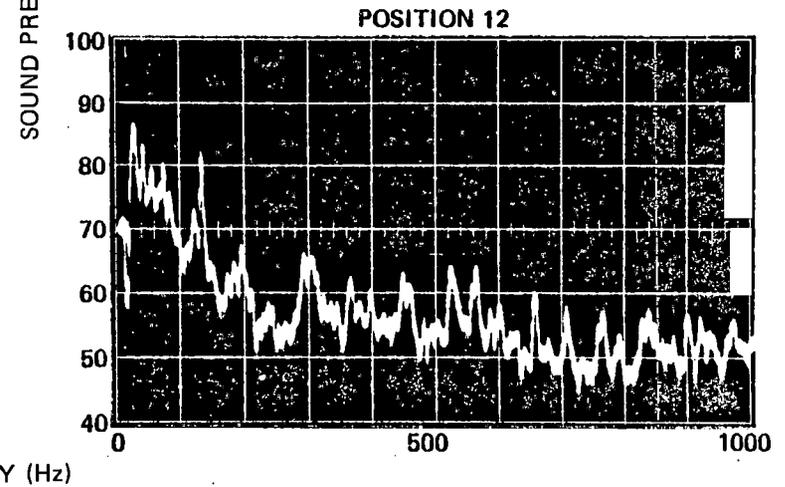
Figure 3-51. Narrowband Analysis of Interior Noise, MBTA, AWO, 50 mph
