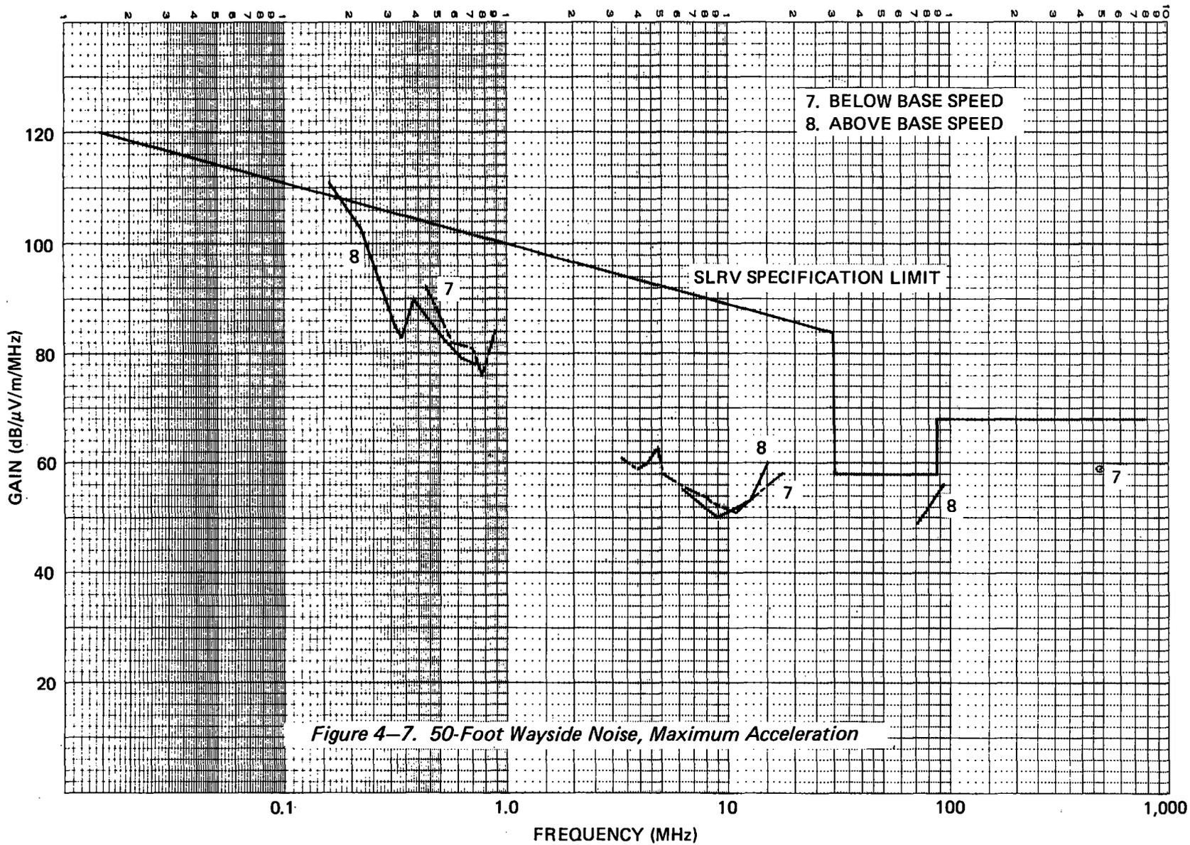
Figure 4-7. 50-Foot Wayside Noise, Maximum Acceleration
