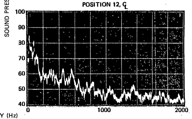
Figure 3-55. Narrowband Analysis of Interior Noise, SFMR, AWO, 40 mph
