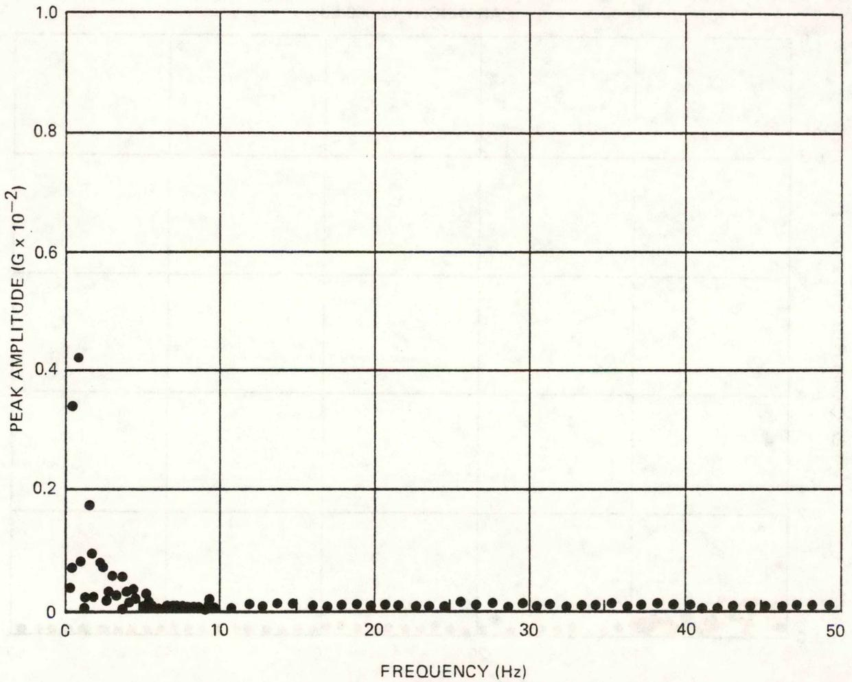
Figure A-7. Narrow-Band Spectrum Analysis – End Car, Lateral
