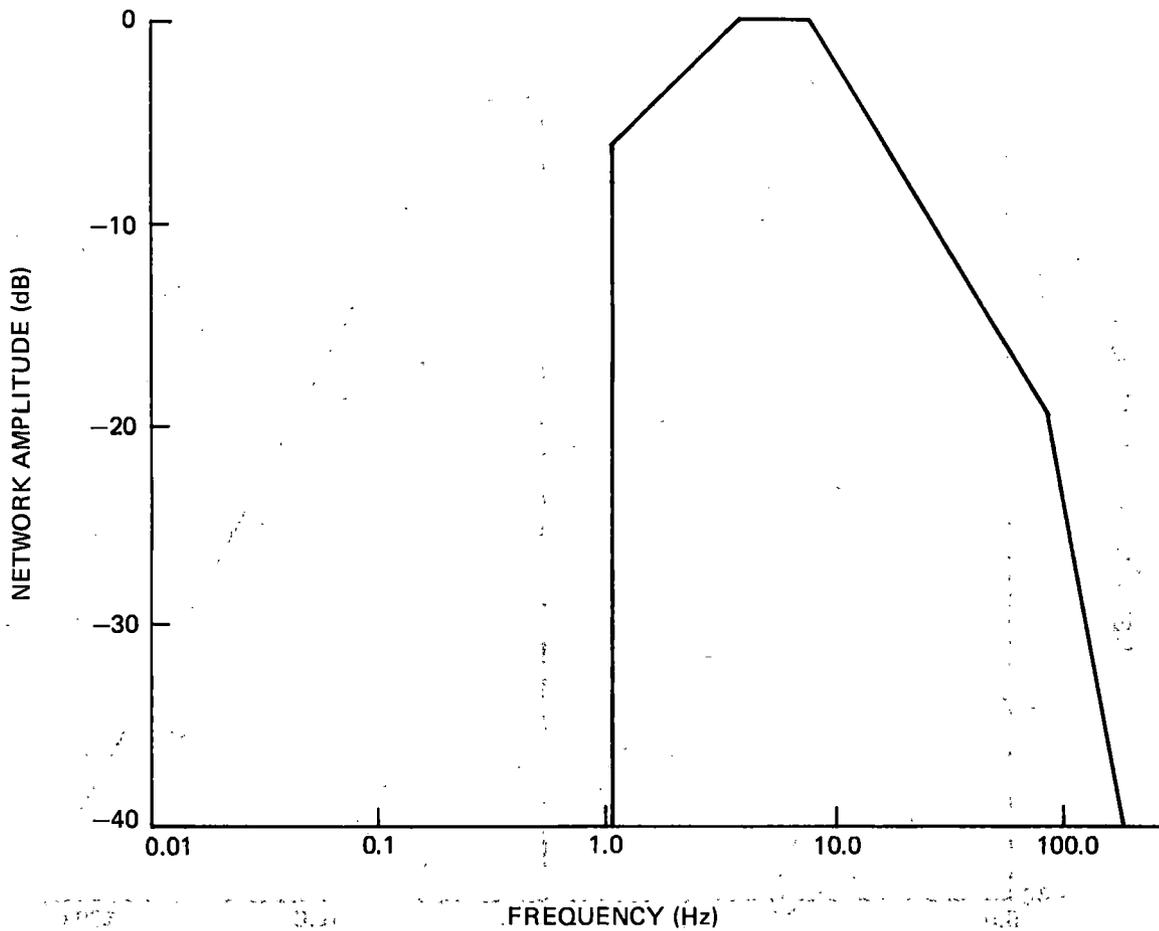
*Figure 2-3. Weighting Network Frequency Response for Vertical Ride Roughness*
