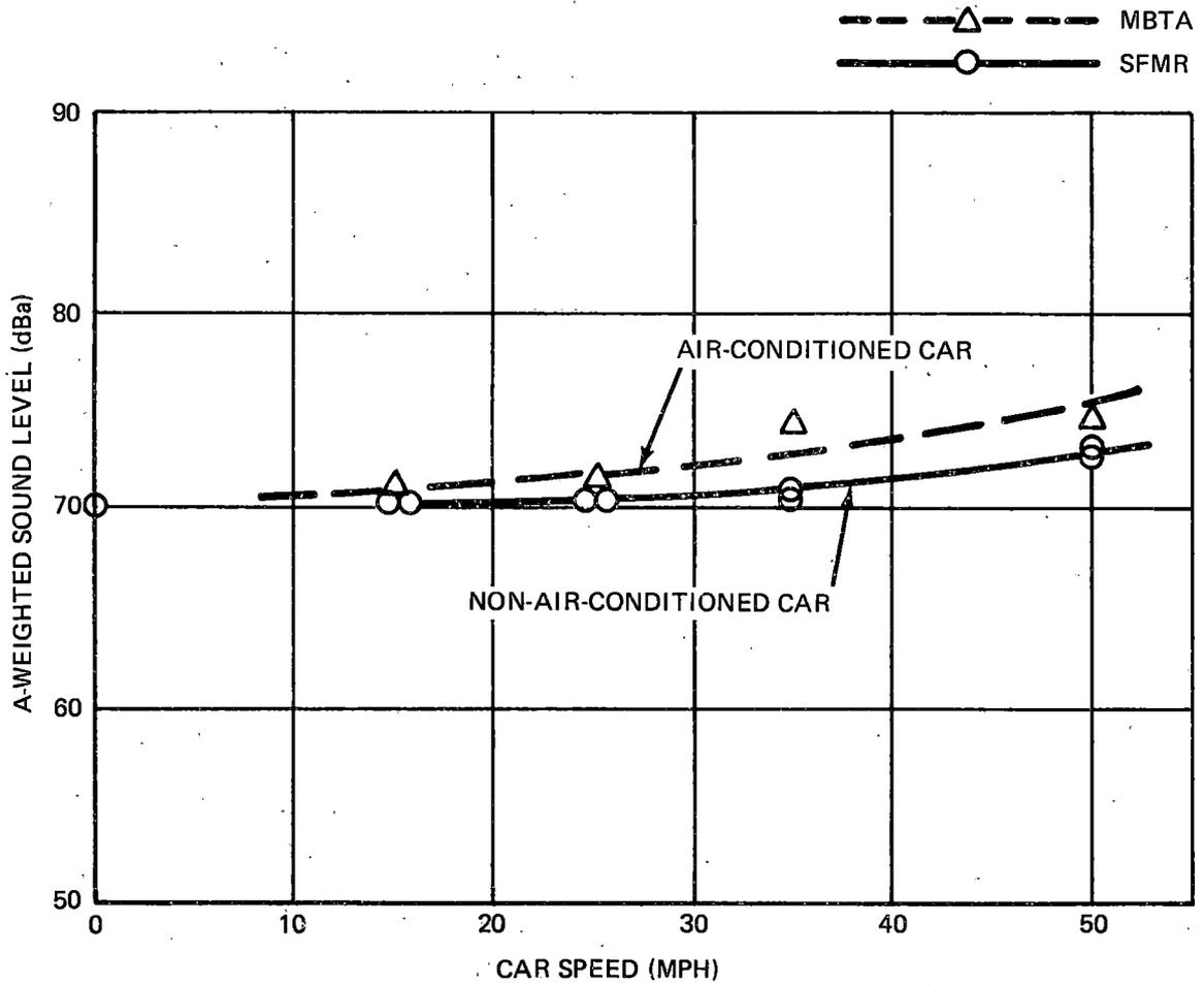
Figure 3-56. SLRV Interior Noise, Position 8, Centerline Between Doors
