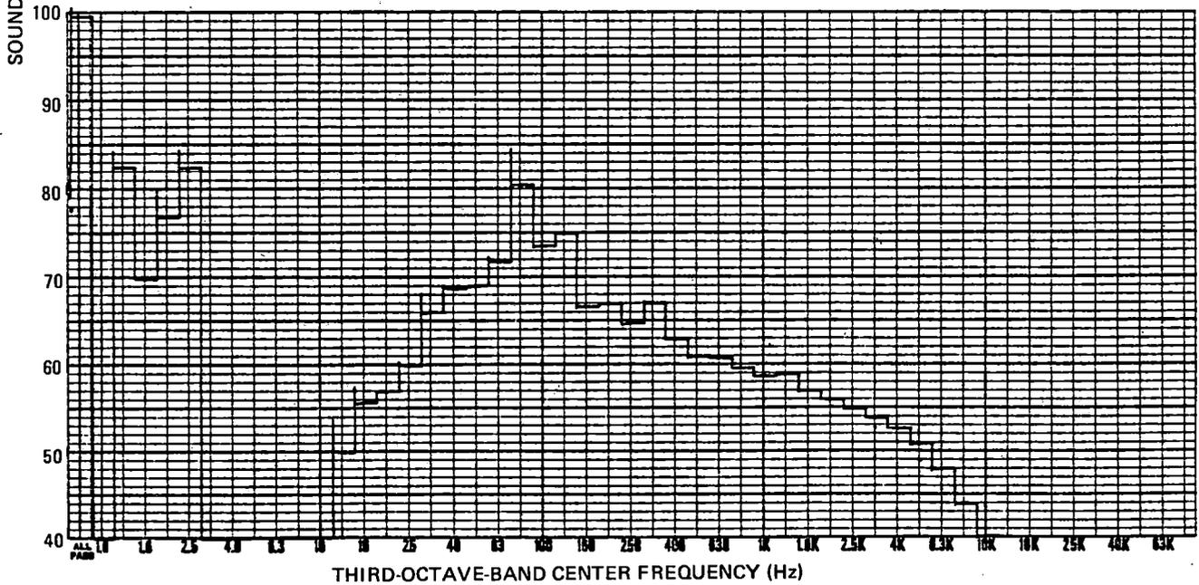
Figure 3-18. Third-Octave-Band Analysis of SFMR Interior Noise, AWO, 15 mph
