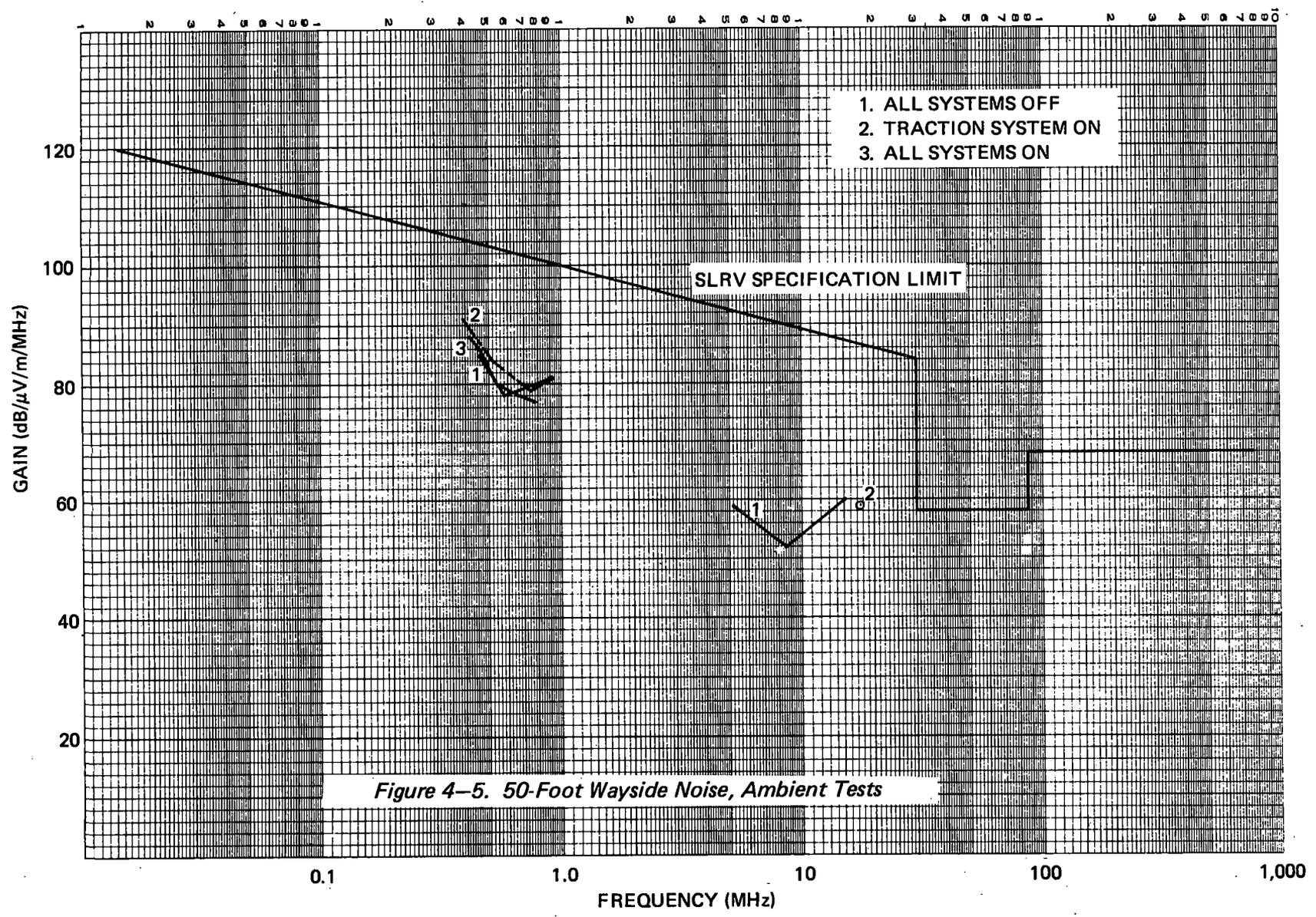
Figure 4-5. 50-Foot Wayside Noise, Ambient Tests
