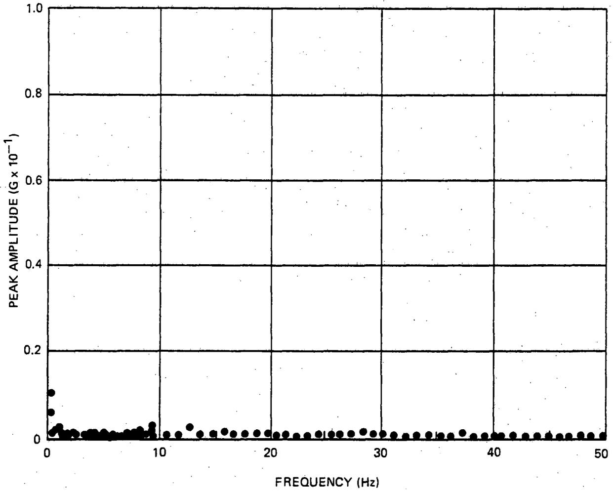
Figure A-8. Narrow-Band Spectrum Analysis — End Car, Longitudinal
