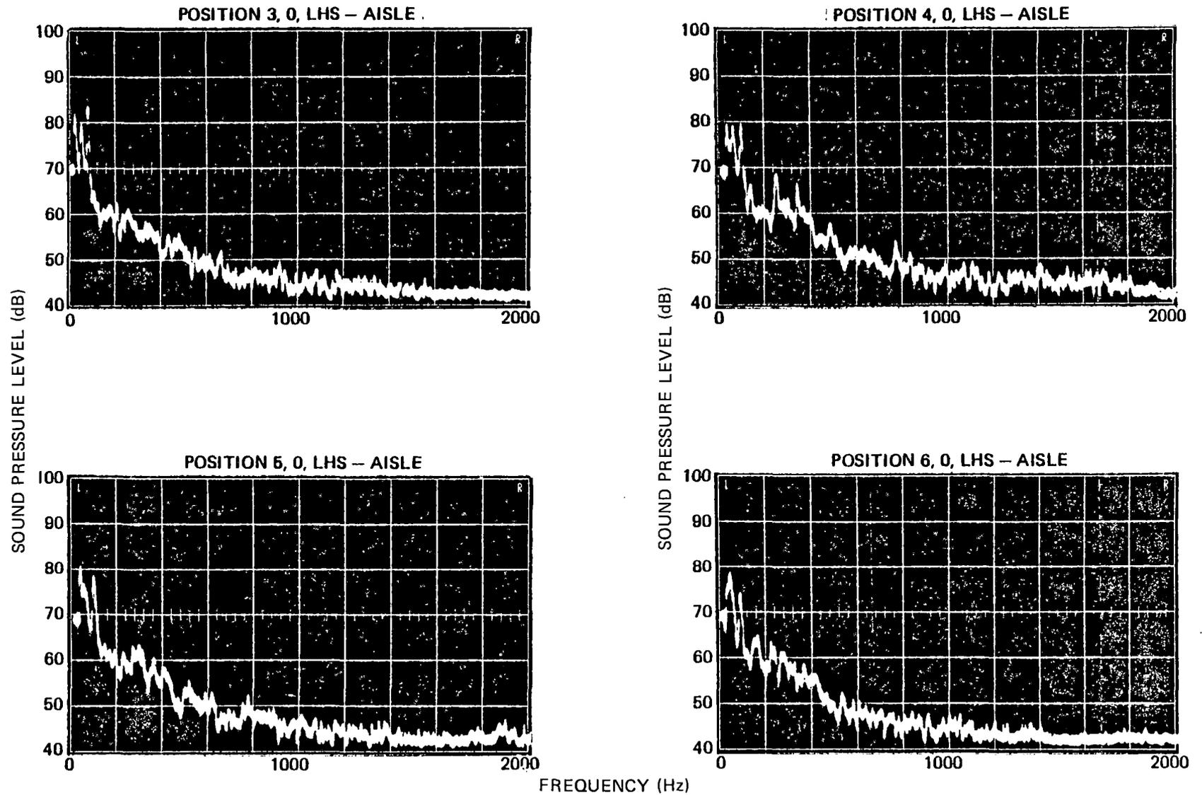
Figure 3-53. Narrowband Analysis of Interior Noise, SFMR, AW0, 40 mph
