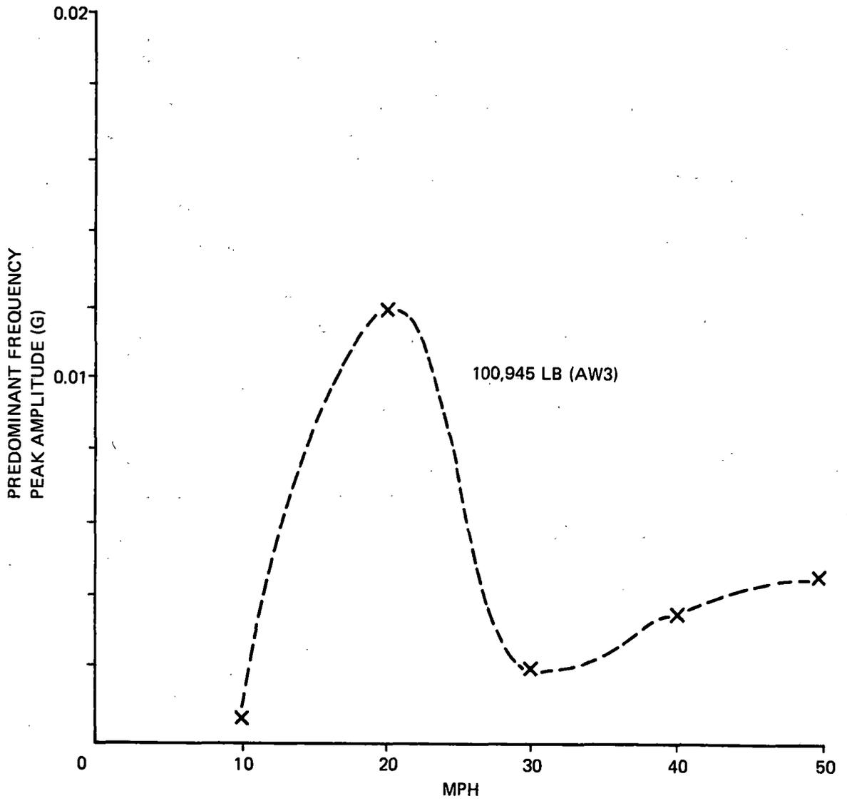
Figure 2-9. Effect of Speed on Longitudinal Ride Roughness, Mid Car
