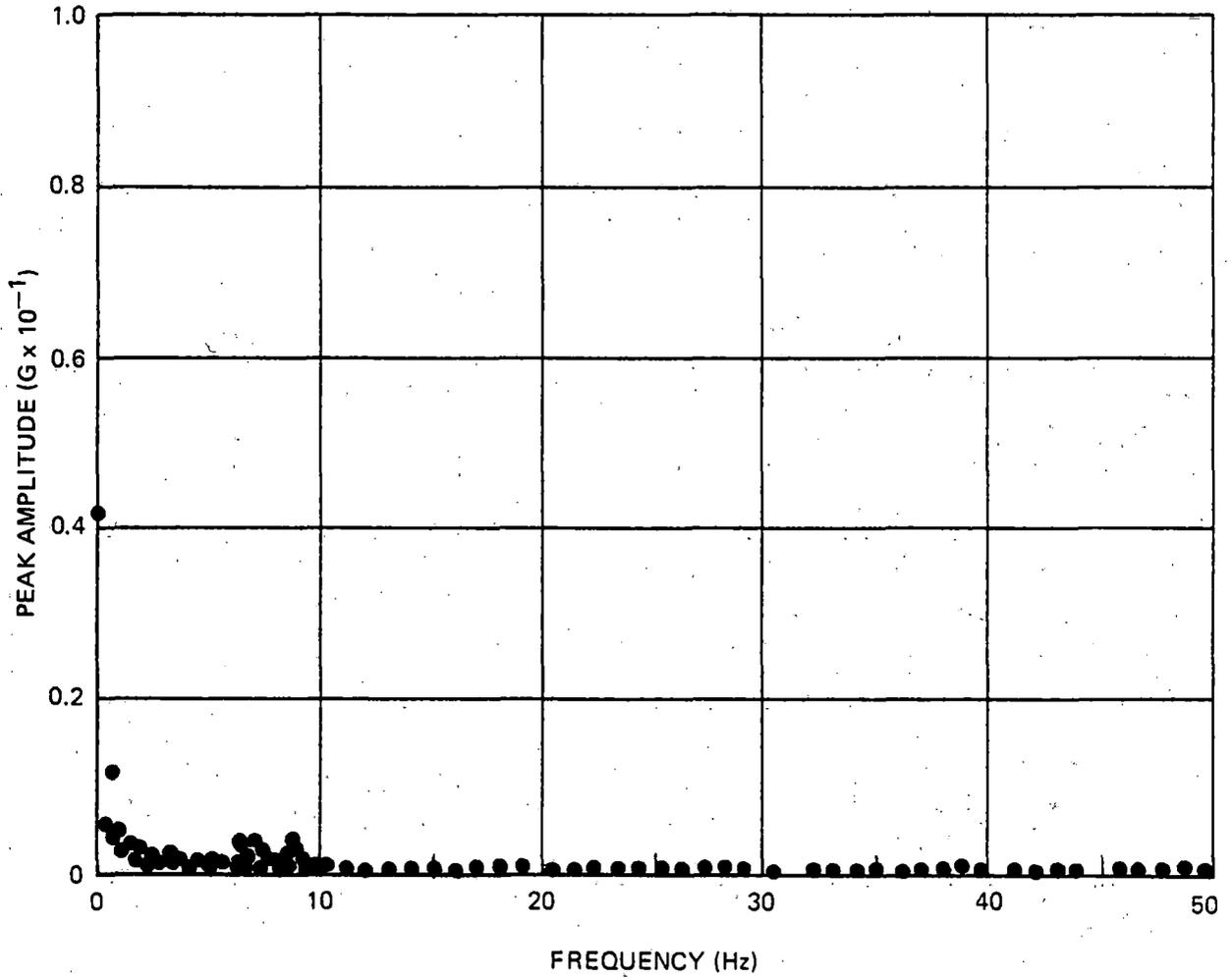
Figure A-44. Narrow-Band Spectrum Analysis — End Car, Longitudinal
