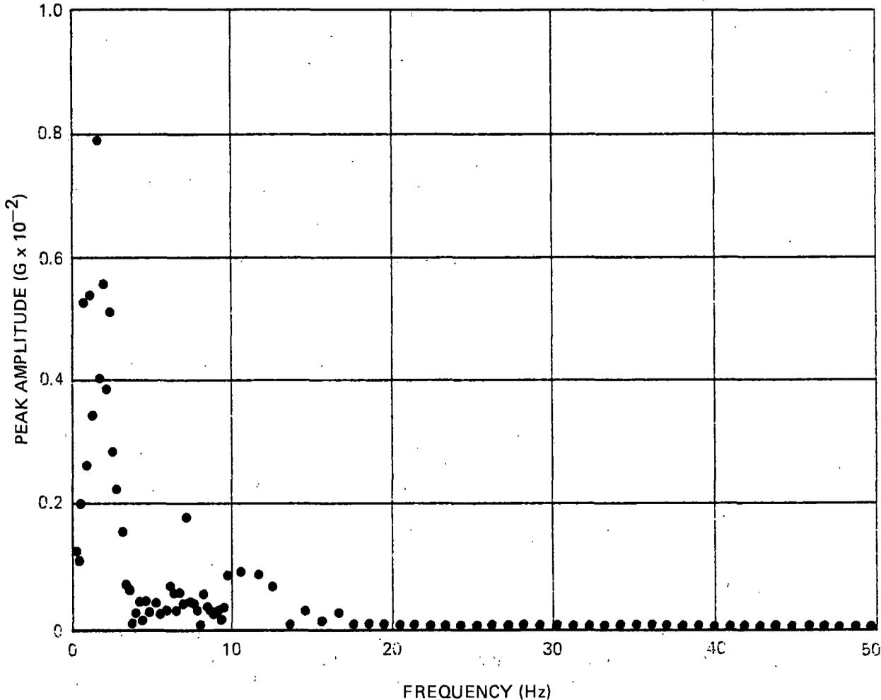
Figure 2-1. Typical Spectrum Analysis – Car Body Vertical Vibration
