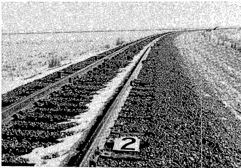
2. SECTION 2 - PIECEWISE LINEAR ALIGNMENT PERTURBATION ON CURVE
