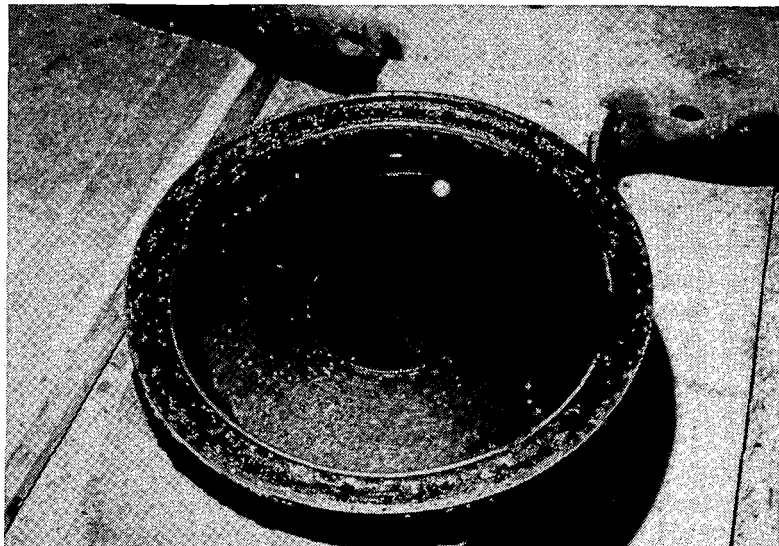
64. SDP-40F BOLSTER CENTER PLATE
