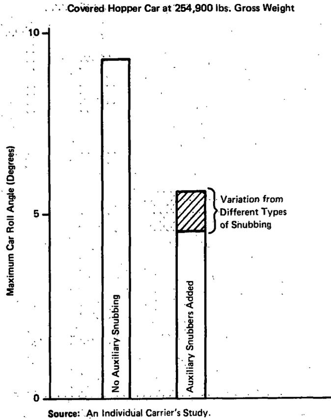
**FIGURE 1-10 IMPROVEMENT POSSIBLE WITH ADDITION OF SNUBBERS**
