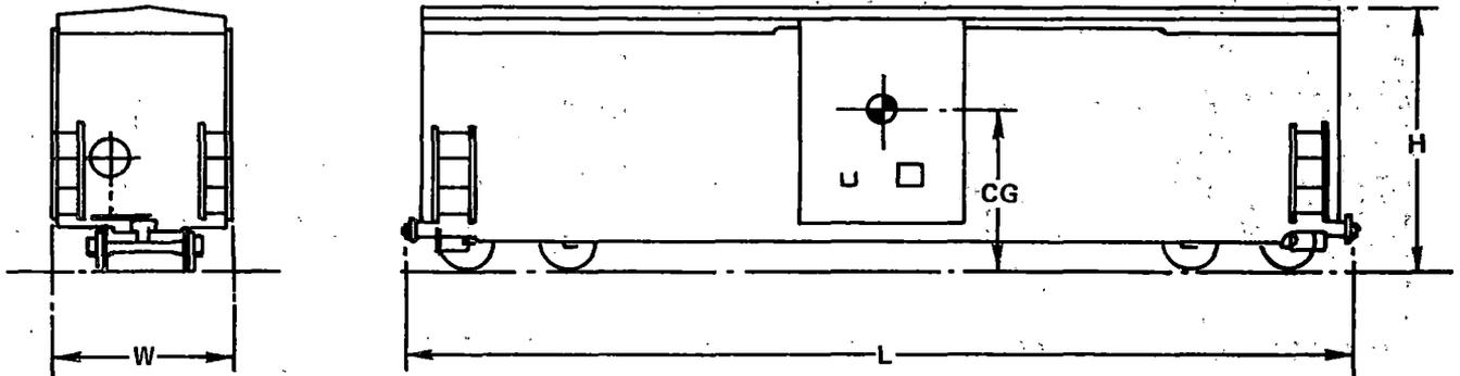
**Length:** Measured between pulling faces of couplers (in normal position)
