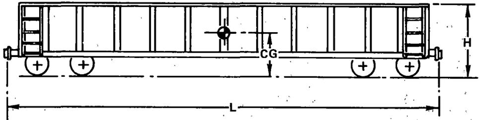
**Length:** Measured between pulling faces of couplers (in normal position)
