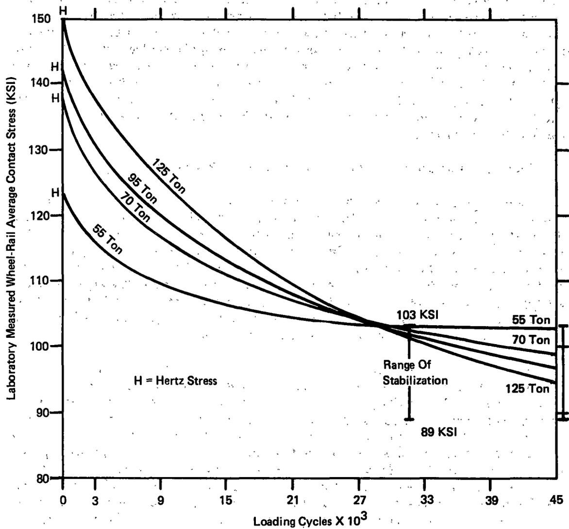
**FIGURE E-2 REDUCTION OF CONTACT STRESS WITH LOADING CYCLES FOR VARIOUS TONNAGE CARS IN LABORATORY SIMULATION**
