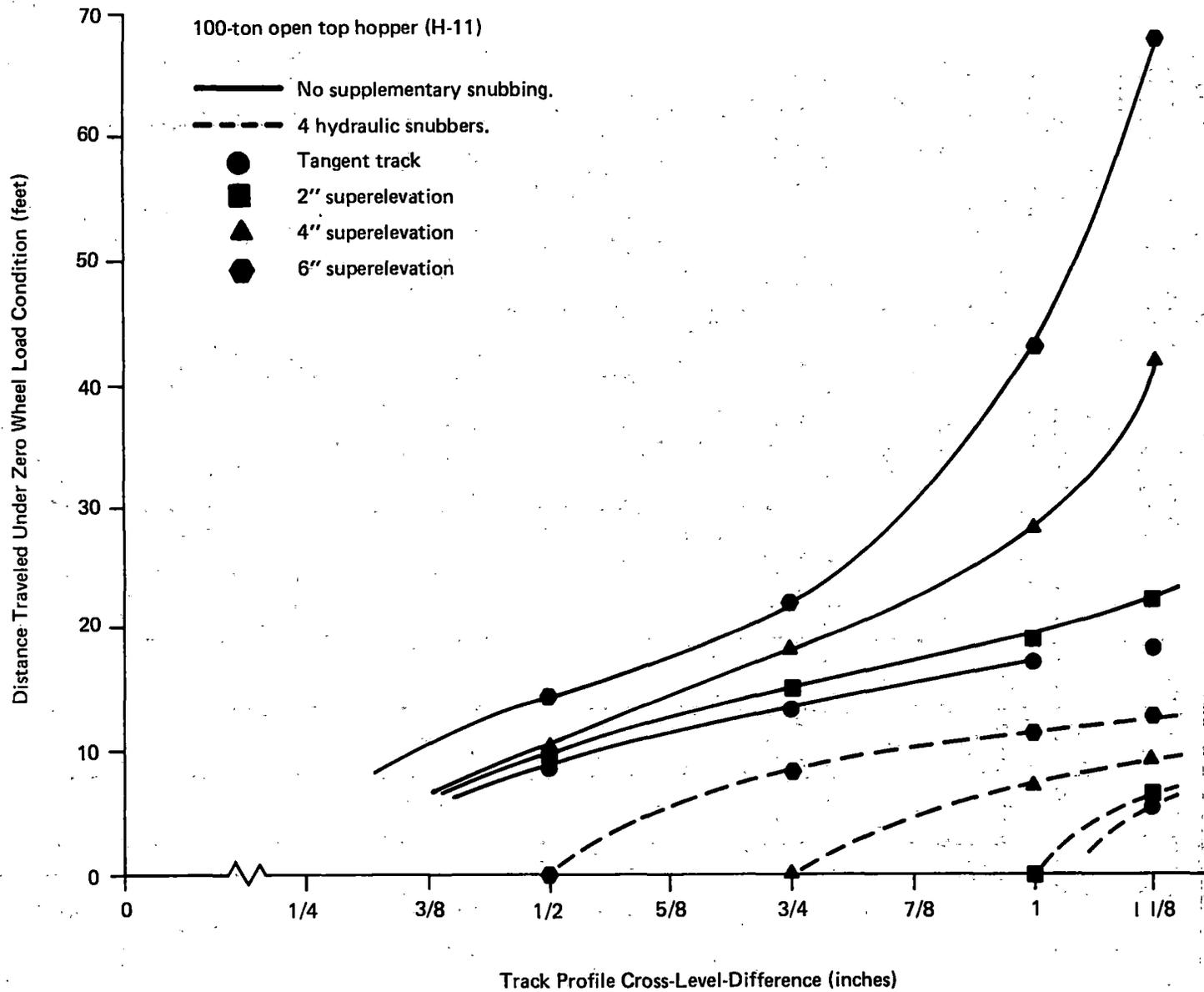
**FIGURE F-10 DISTANCE TRAVELED UNDER ZERO WHEEL LOAD CONDITION AT RESONANT SPEED FOR VARIOUS TRACK CONDITIONS**
