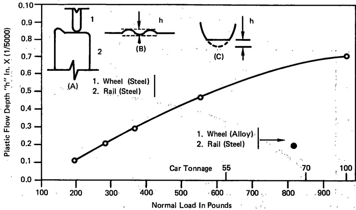
FIGURE E-4 PLASTIC FLOW VS NORMAL LOAD
