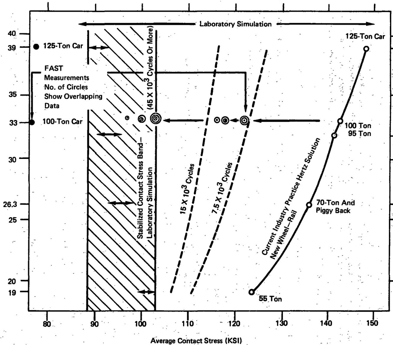
FIGURE E-3 LABORATORY AND FIELD MEASUREMENTS OF WHEEL RAIL CONTACT STRESSES FOR NEW, INTERMEDIATE, AND STABILIZED CONDITIONS
