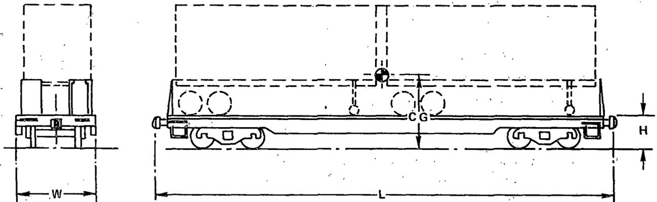
**Length:** Measured between pulling faces of couplers (in normal position)
