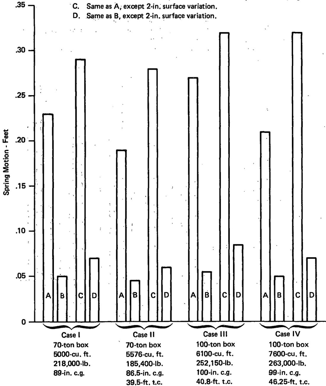
**FIGURE F-9 EFFECT OF SNUBBING AND TRACK GEOMETRY ON SPRING MOTION**
