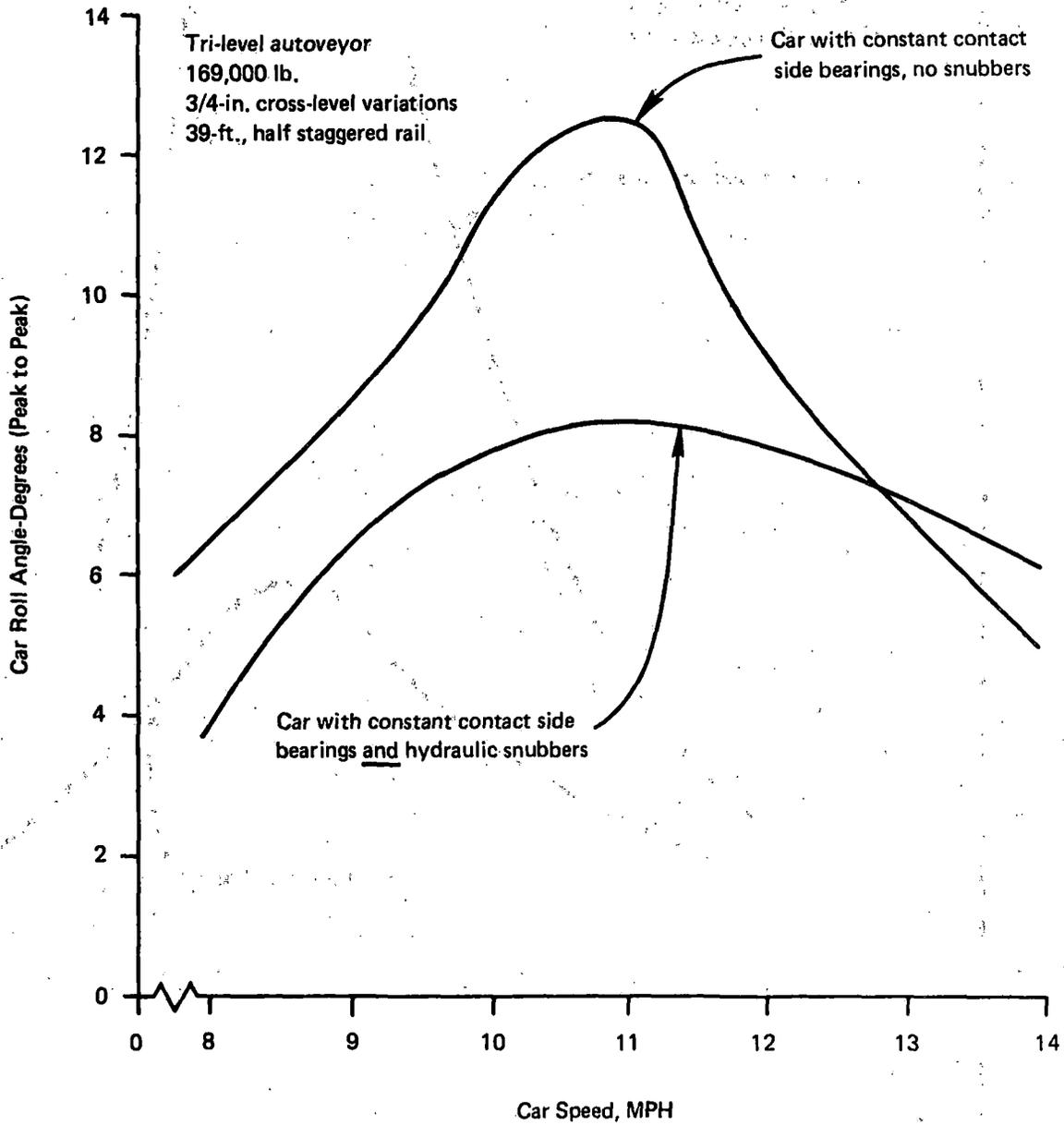
**FIGURE F-2 EFFECT OF CONSTANT CONTACT SIDE BEARINGS AND HYDRAULIC SNUBBING ON MAXIMUM CAR ROLL ANGLE**
