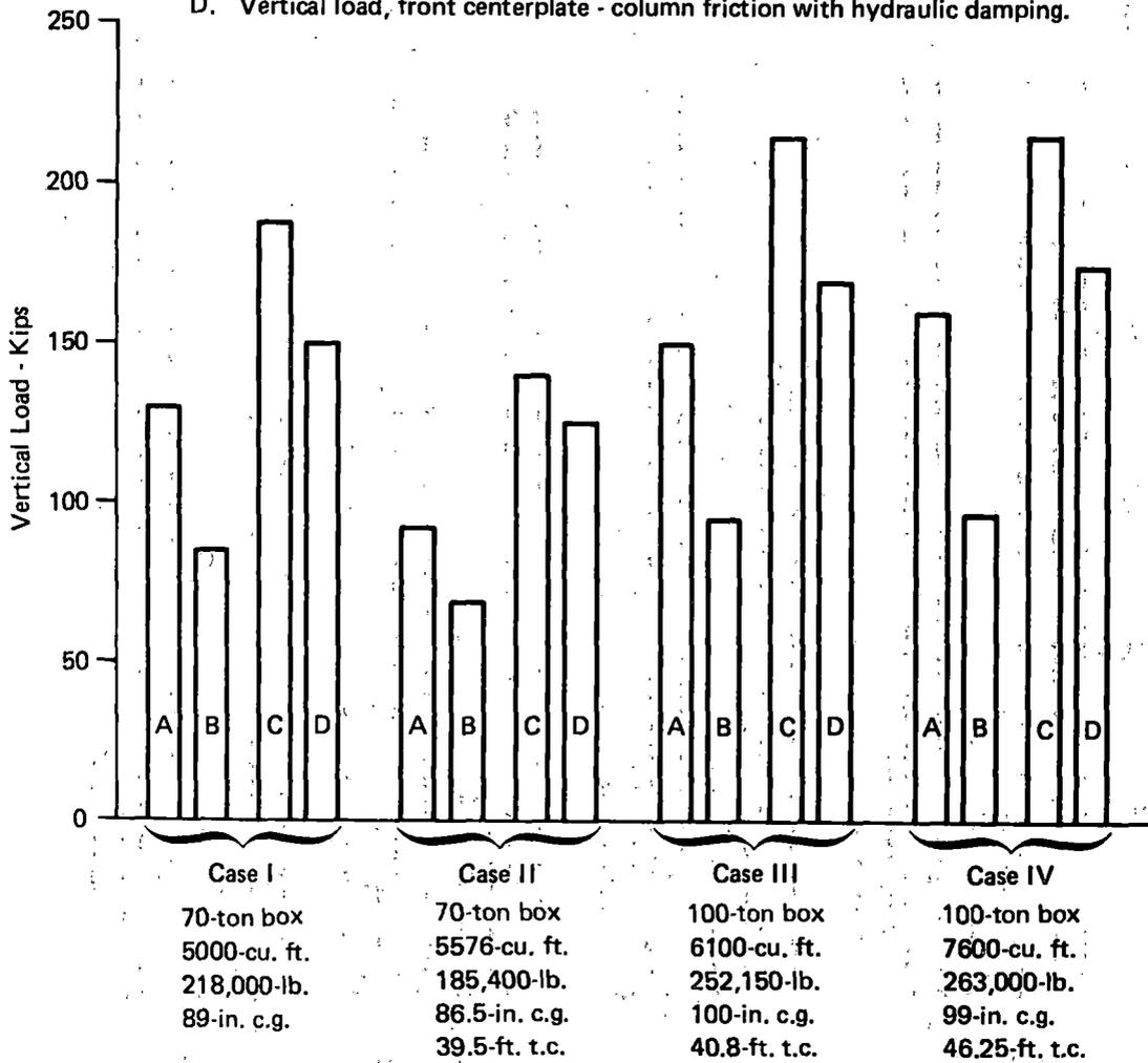
FIGURE F-8 EFFECT OF SNUBBING ON VERTICAL WHEEL LOADS
