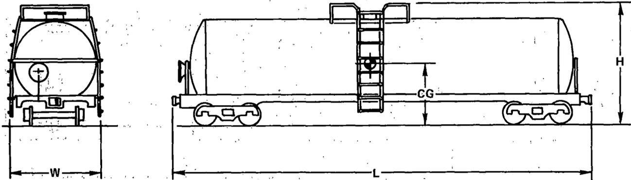
**Length:** Measured between pulling faces of couplers (in normal position)
