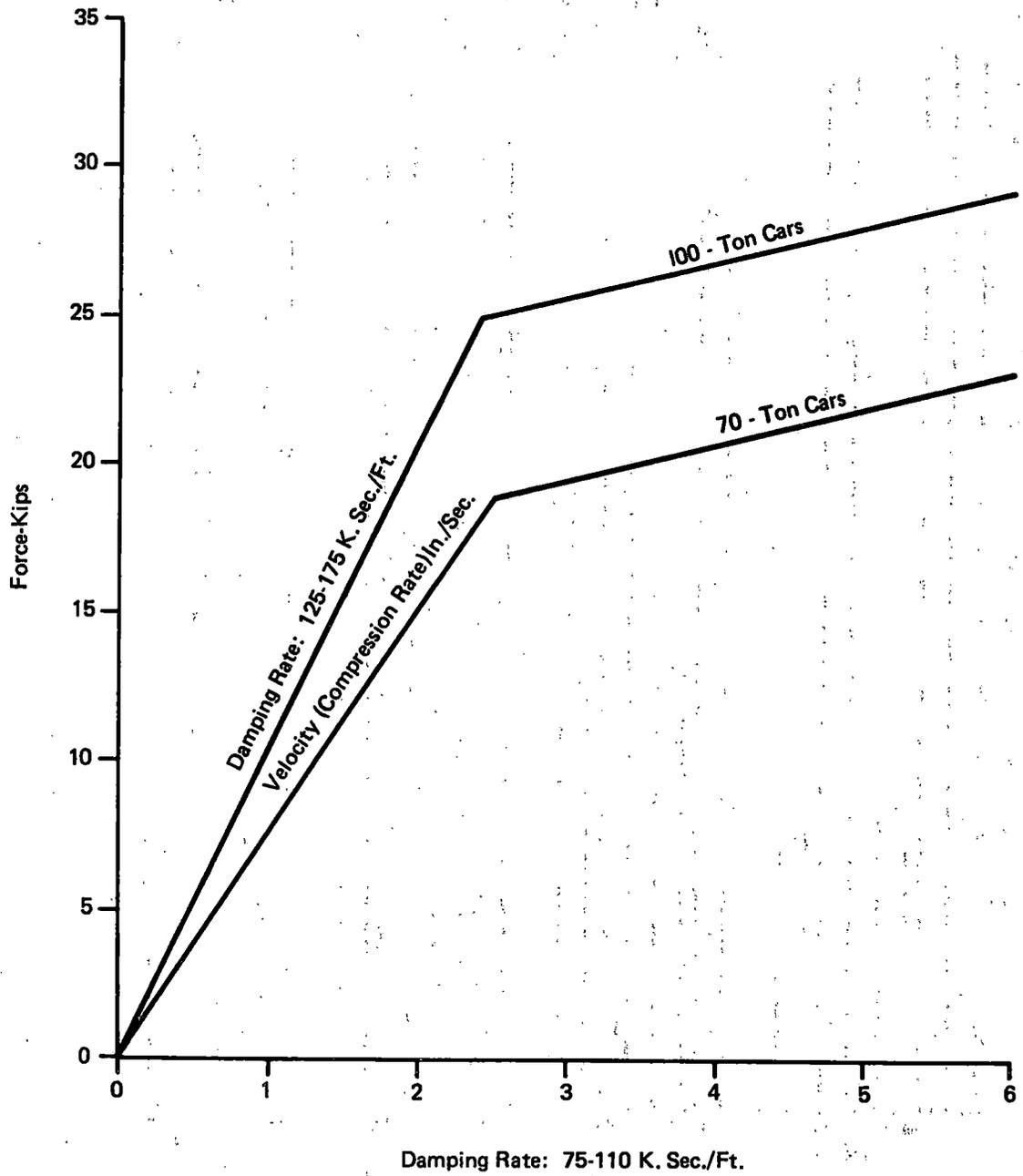
**FIGURE F-4 DAMPING CHARACTERISTICS OF HYDRAULIC STABILIZERS FOR 70 AND 100-TON CARS**
