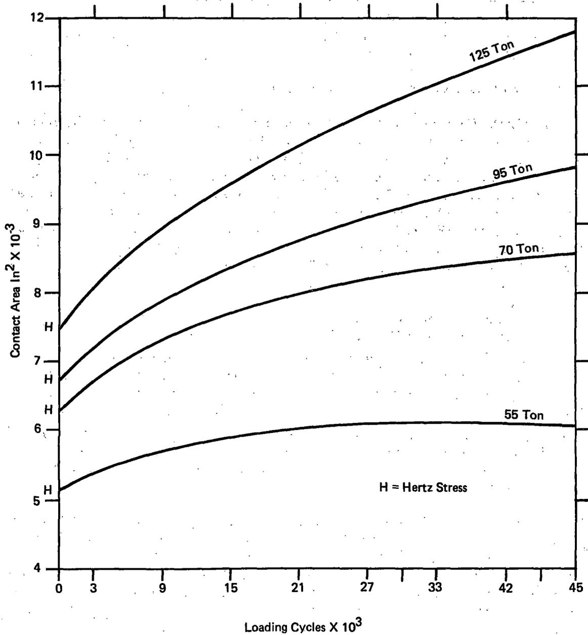
**FIGURE E-1 GROWTH OF AREA OF CONTACT FOR WHEEL AND RAIL IN DIFFERENT TONNAGE CARS IN LABORATORY SIMULATION**
