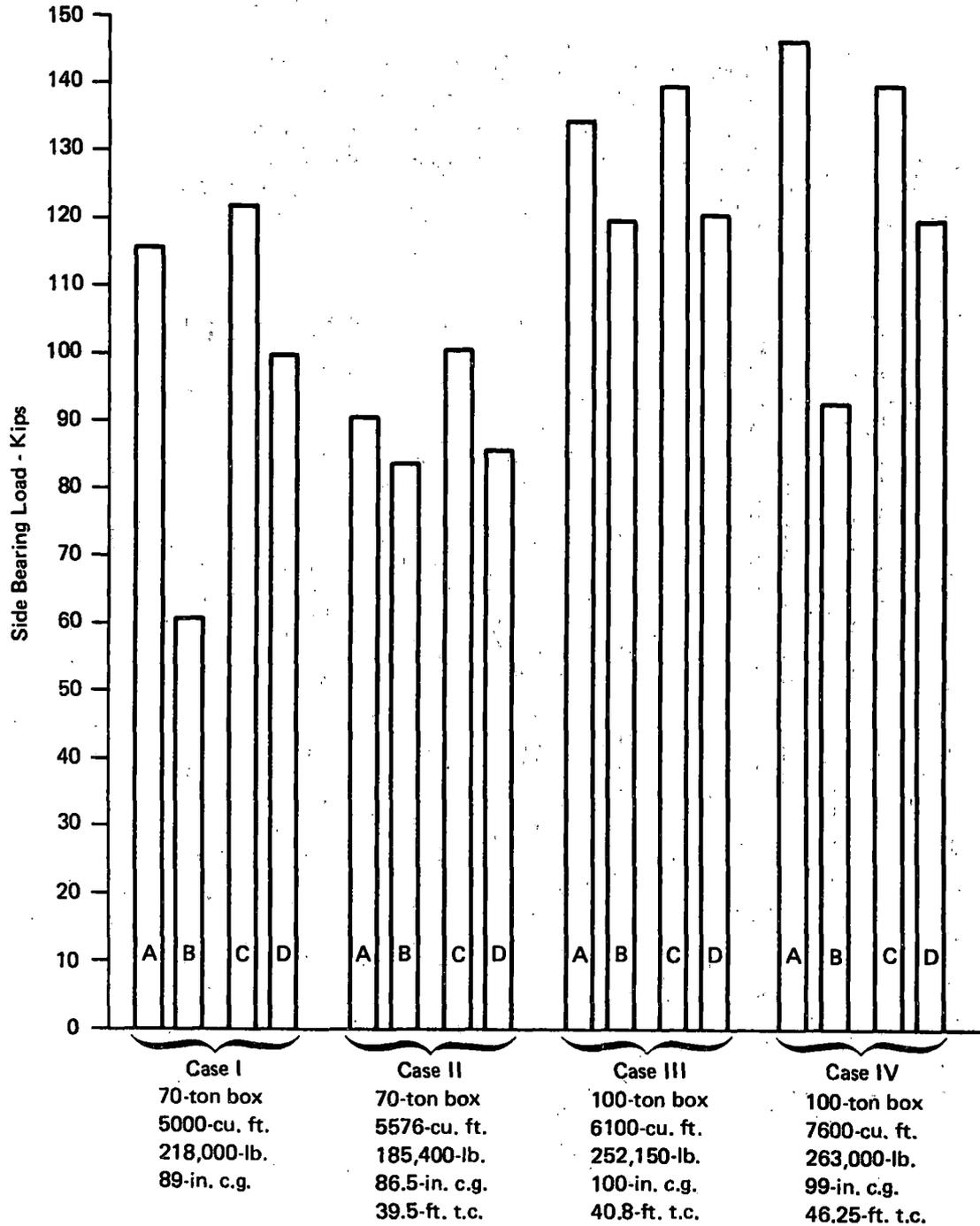
FIGURE F-6 EFFECT OF SNUBBING ON SIDE BEARING LOAD
