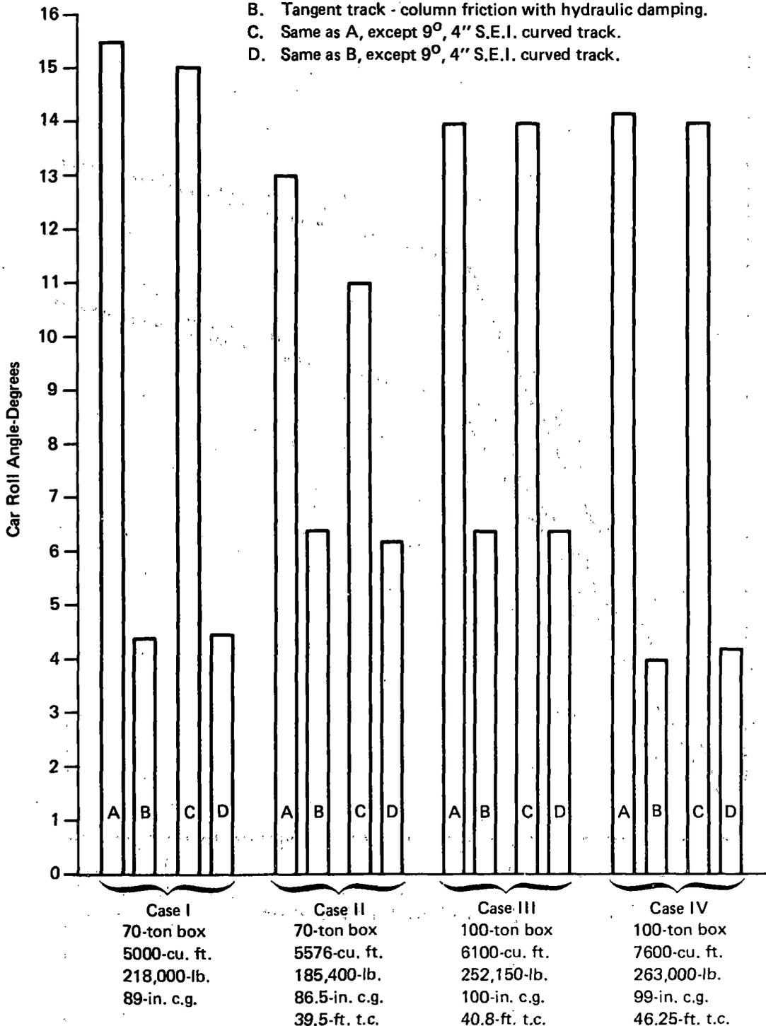
**FIGURE F-5 EFFECT OF SNUBBING ON CAR BODY ROLL ANGLE ON TANGENT AND CURVED TRACK**
