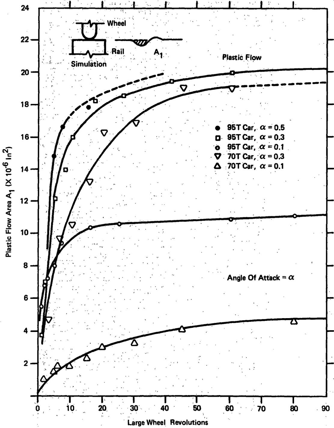
FIGURE E-9 GROWTH OF PLASTIC FLOW FOR 95-TON AND 70-TON CARS AT VARIOUS ANGLES OF ATTACK
