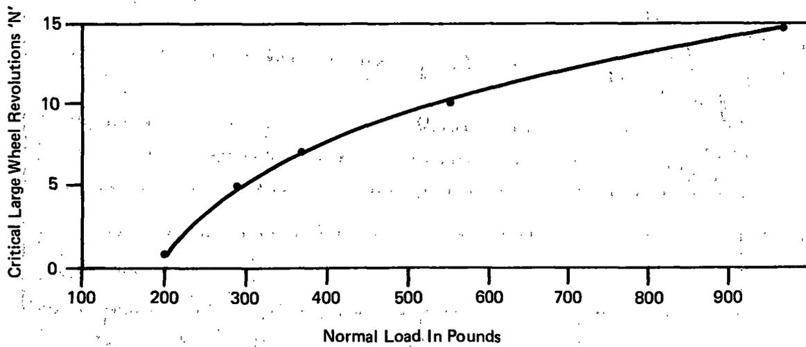
FIGURE E-7 CRITICAL DISTANCE VS NORMAL LOAD
