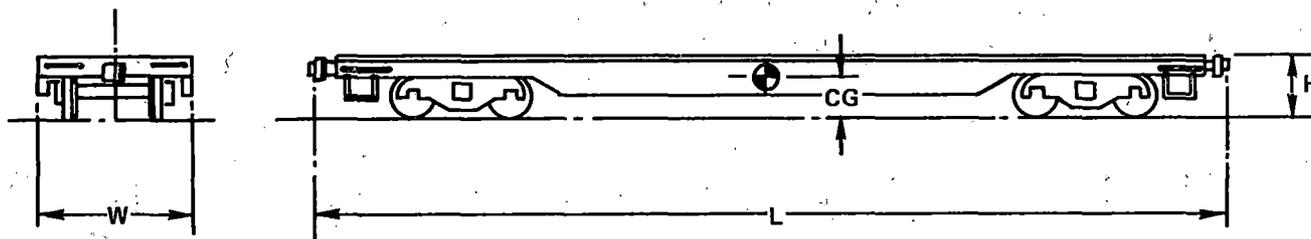
**Length:** Measured between pulling faces of couplers (in normal position)
