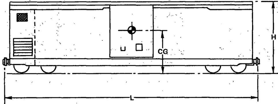
**Length:** Measured between pulling faces of couplers (in normal position)
