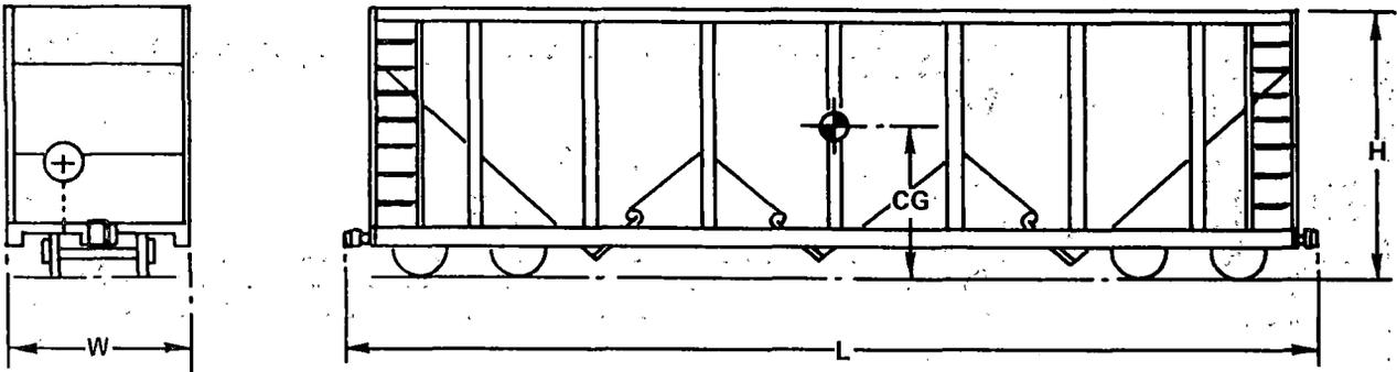
**Length:** Measured between pulling faces of couplers (in normal position)
